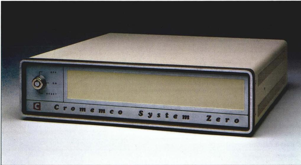
The System Zero is ideal for ROM-based, dedicated applications. A basic System Zero includes a fast, Z-80A based single card computer, 8K bytes of on-board 2716 PROM capacity (PROMs not included), and 1K byte of static RAM memory. Interfacing is through an RS-232 (or 20mA current loop) serial interface with programmable baud rates to 76,800 baud. The single card computer also provides 24 bits of bidirectional parallel I/O, five programmable
