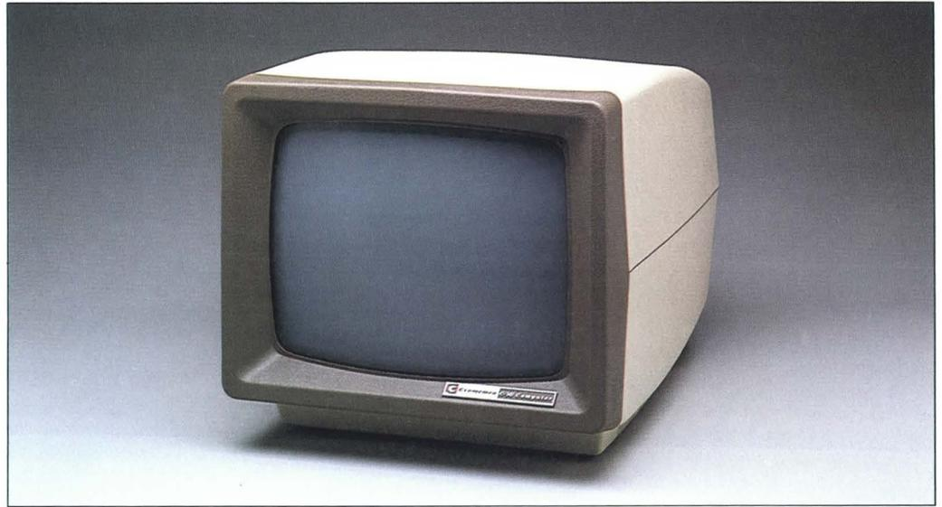
The basic C-10 includes the Z-80A microprocessor, 64Kb of RAM, 24Kb of ROM, and a high-resolution 12" green phosphor CRT, which is capable of displaying 80 columns and 25 lines of data.
