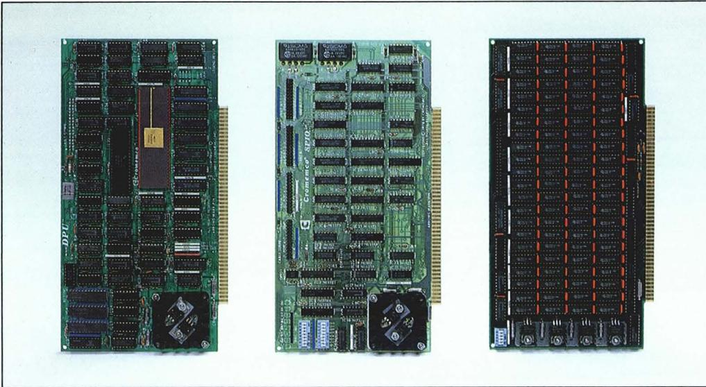
Cromemco offers a wide variety of board-level products which are designed to expand the capability of Cromemco systems. These products include CPUs, memory boards, and I/O boards. All boards have been fully integrated with each other and with Cromemco systems to assure reliability. With these S-100 bus (IEEE-696 standard) boards, systems can be
