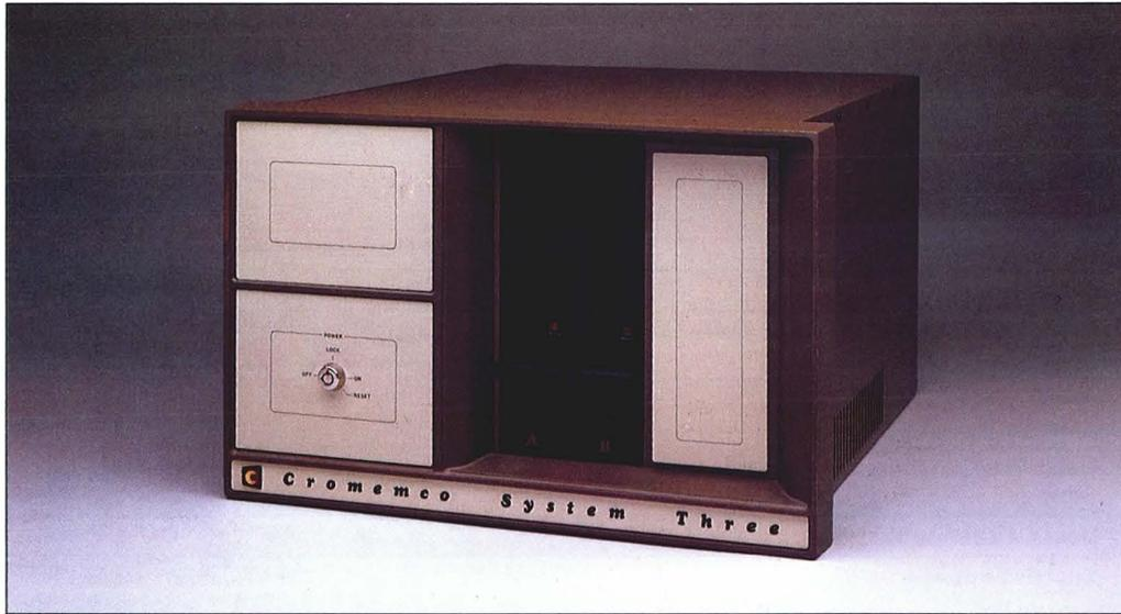
The Cromemco System Three, which combines large disk storage with processing power and room for expansion, is ideal for commercial applications. The D-Series System Three can easily handle multiple users performing multiple jobs such as the manipulation of large data bases, data analysis, accounting, word processing, and a variety of similar applications.
