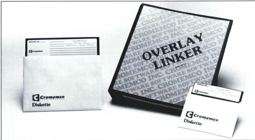
Cromemco's Z-80 Overlay Linker permits construction and execution of programs that are too large to fit into available memory. To do this, the programmer first writes the large program in modules. The Overlay Linker program is then used to build a tree-like structure of overlays with the modules.
