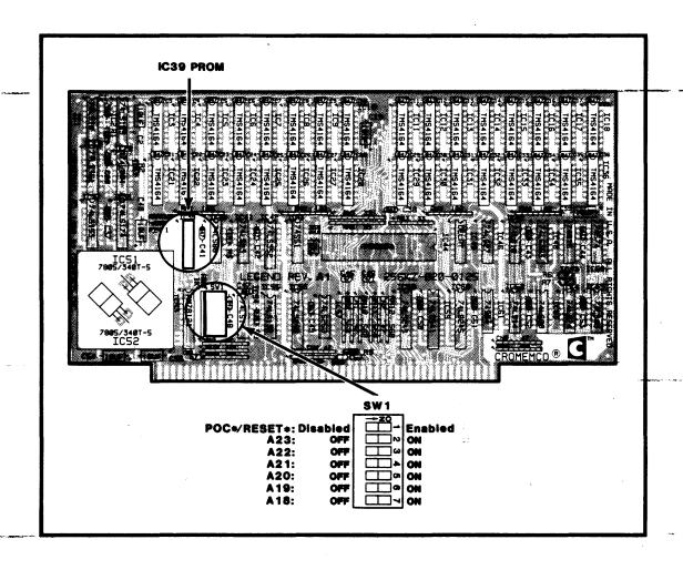
Switch bits two through seven are only significant in 68000 based Cromix systems.
