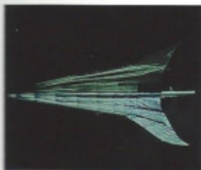
High Speed Civil Transport surface flow visualization calculated with TLNS3D (top) compared with experimental oil flow (bottom).
