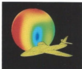
Radar cross section (RCS) of a military aircraft. Red indicates regions of high RCS and blue indicates low RCS. Calculations performed using a frequency domain code with an out-of-core solver from the EMMA software suite. PATRAN has been used for preprocessing and visualization is via MPGS.
