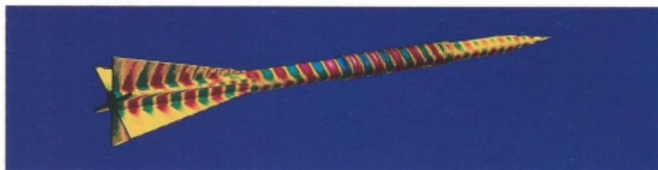
Radar cross section (RCS) of a finned projectile computed from surface electrical fields at one instant of time. The RCS was obtained from solving the Maxwell's equations on a CRAY Y-MP supercomputer.
