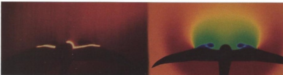
Airflow over a High Speed Civil Transport model calculated using TLNS3D, a central difference, finite volume, Navier-Stokes code. The computed flow pattern shows the correct shape and growth of the primary and secondary vortices and is found to be in agreement with the experimental data.
