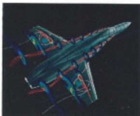
F-18 aircraft flowfield. Image shows pressure contours and the vortical nature of the flow, as well as traces showing the path of selected fluid particles. Computations required 100 million 64-bit words of memory for the solution at 1.25 million grid points.
