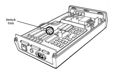
Utility Server Circuit Board & Switch Unit Choose an address from 0 to 63 for your utility server. The address you choose must be different from the addresses of all other devices on your network. Write down your choice on a piece of paper and tape it to the outside of your server. Set the switches for your chosen address as shown in the table below.
