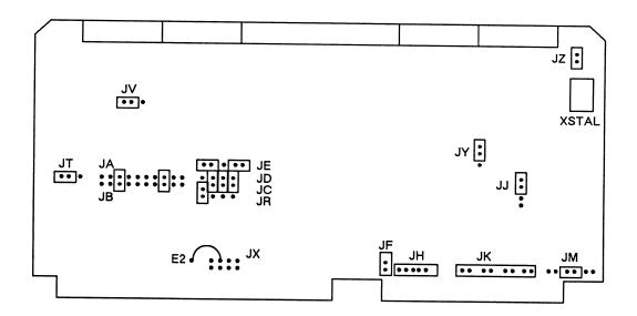
Figure 3-3. Xylogics Model 450 Disk Controller, Revision L, Jumper Configurations
