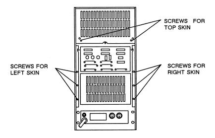
Figure 2-13. Model 31 CADDStation Deskside Module, Rear View
