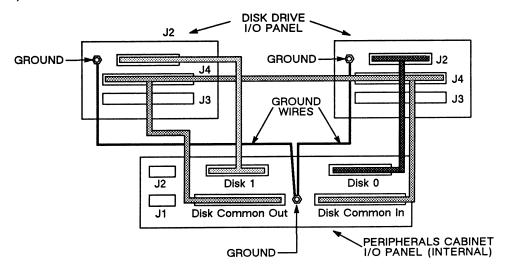
Figure 7-18. 515MB Disk Drive Internal Cabling, First Configuration
