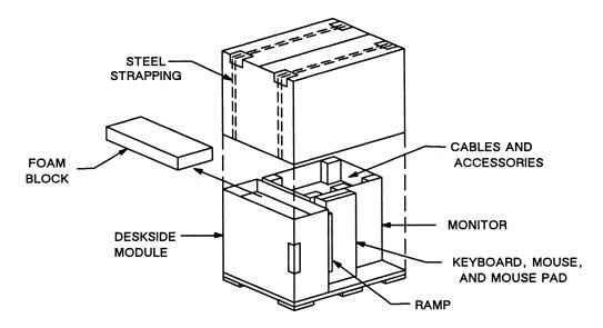
Figure 1-1. Shipping Configuration for Model 32 and 31 CADDStations
