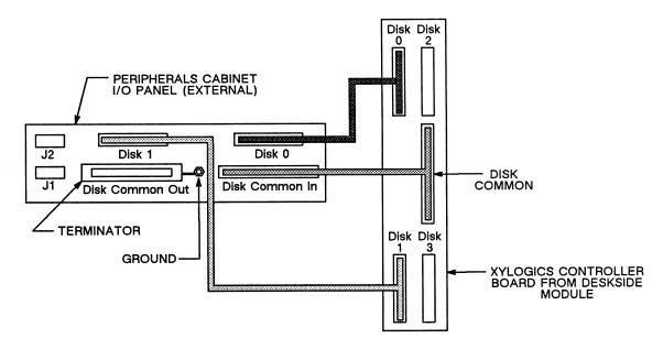
Figure 7-19. 515MB Disk Drive External Cabling, First Configuration
