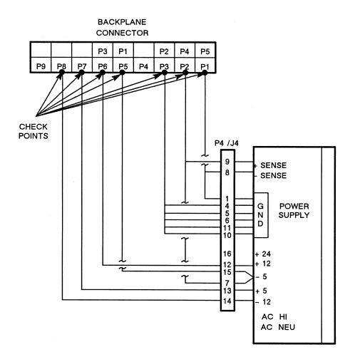
Figure 6-3. Nine-Slot DC Power Distribution and Backplane Checkpoints
