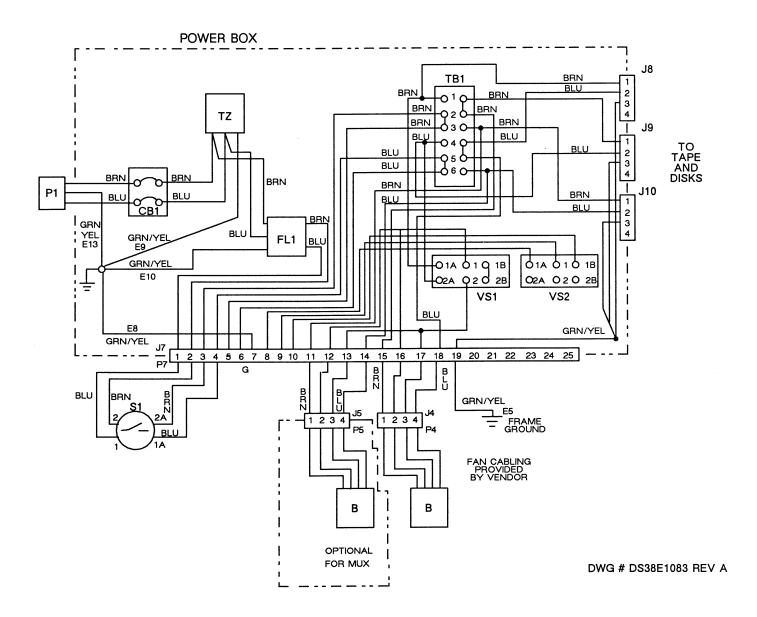
Figure 8-3. CADDServer Peripherals Cabinet, Power Distribution
