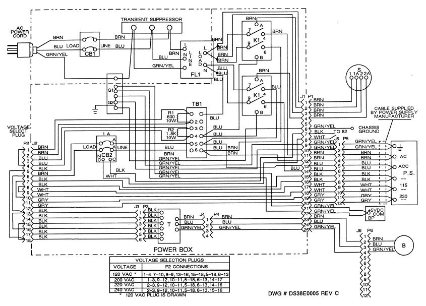
Figure 8-1. Model 32 CADDStation Deskside Module AC Power Distribution
