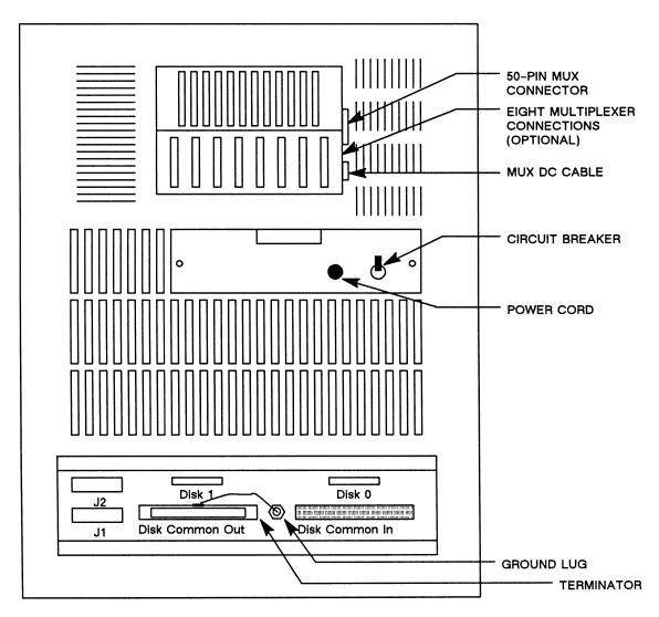
Figure 5-6. CADDServer Peripherals Cabinet I/O Panel
