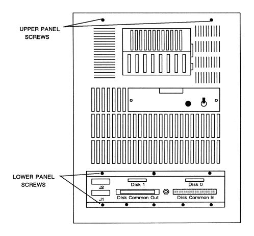
Figure 2-17. CADDServer Peripherals Cabinet, Rear Panel
