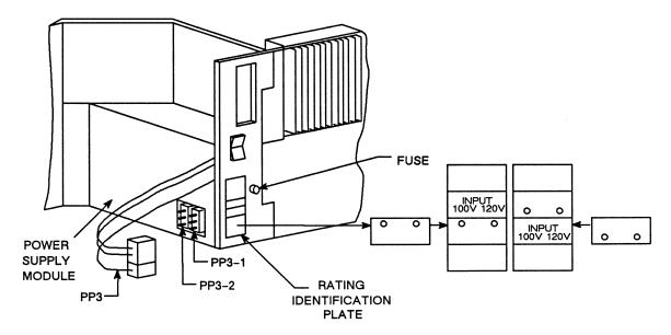
Figure 2-8. Color Monitor Voltage Selection
