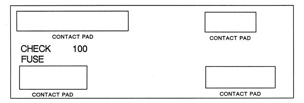
Figure 2-6. Model 30M 100 VAC Voltage Selection through PCB
