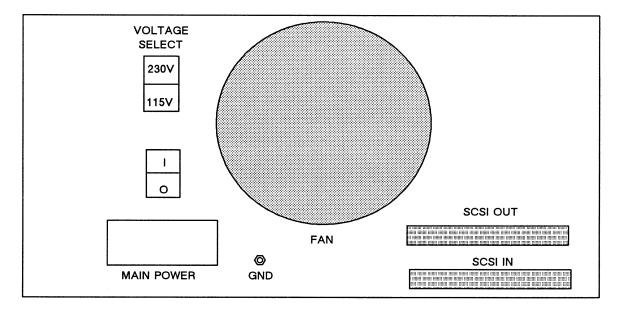
Figure 7-14. 170MB Disk Drive Expansion Box, Rear View
