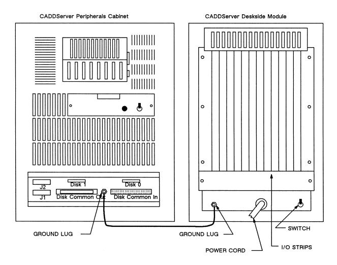
Figure 5-7. CADDServer Grounding Connection
