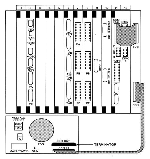
Figure 7-15. Expansion Box Connections for a Diskful CADDStation with an SMPL Board
