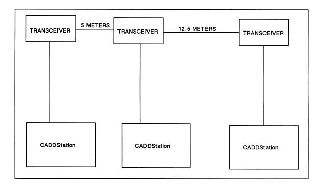
Figure 5-9. Ethernet Cabling Lengths
