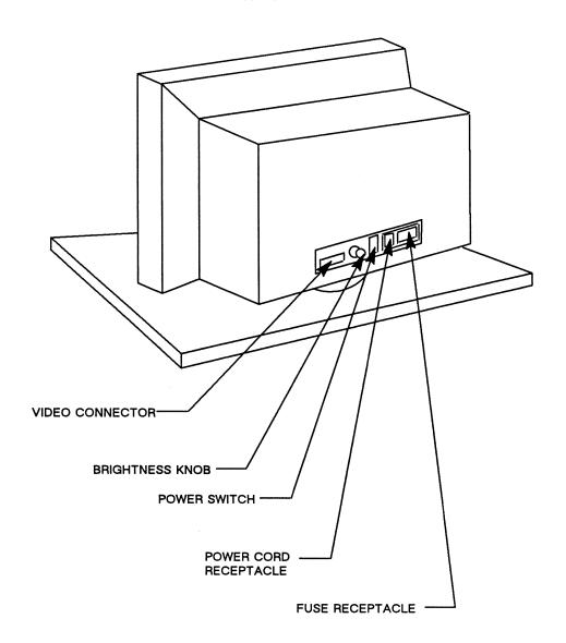
Figure 6-1. Monochrome Graphics Display, Rear View
