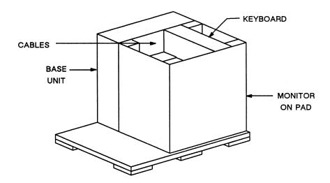
Figure 1-3. Shipping Configuration for Model 32CV/32MV CADDStations
