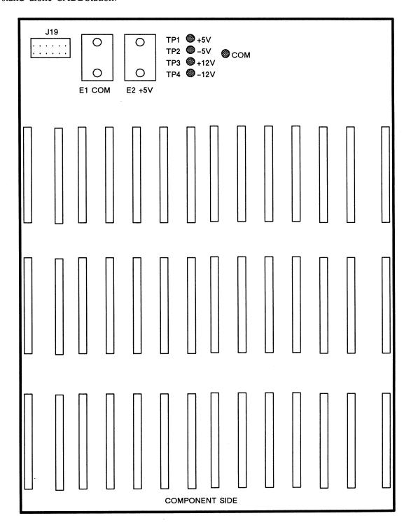
Figure 6-4. 12-Slot Backplane Power Supply Checkpoints
