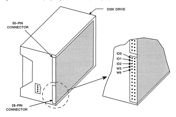
Figure 7-11. 170MB Disk Drive Jumpering Locations, Second Configuration
