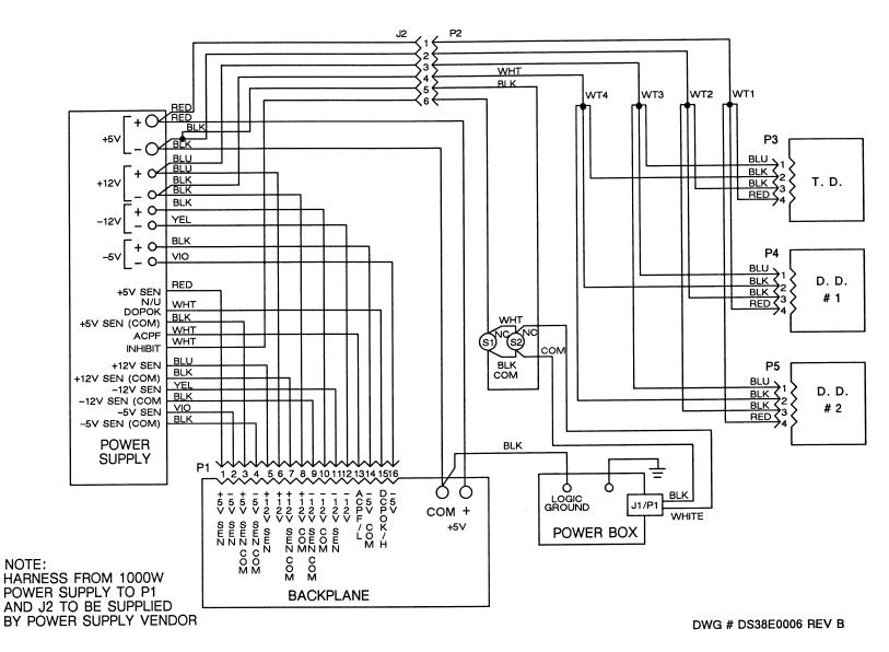
Figure 8-2. Model 32 CADDStation Deskside Module DC Power Distribution
