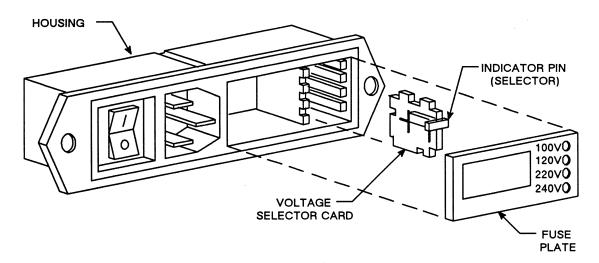
Figure 2-2. Computervision Monochrome Monitor Voltage Selection
