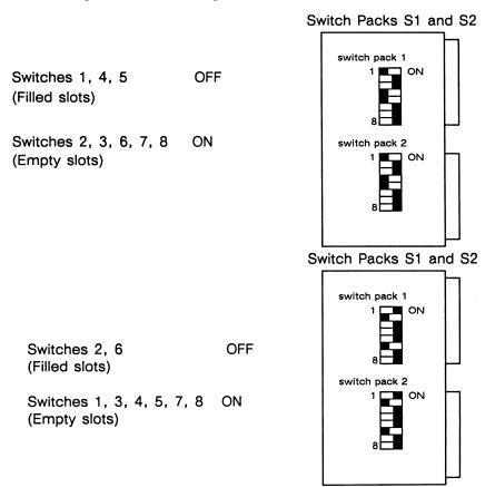
Figure 3-1. Terminator Board Switch Settings Example, Revision A
