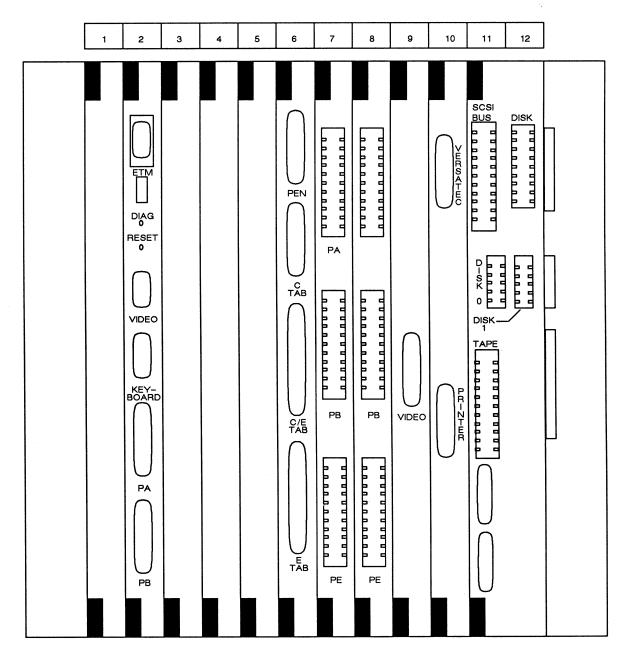
Figure 5-2. Deskside Module I/O Strips, Model 32 12-Slot CADDStation
