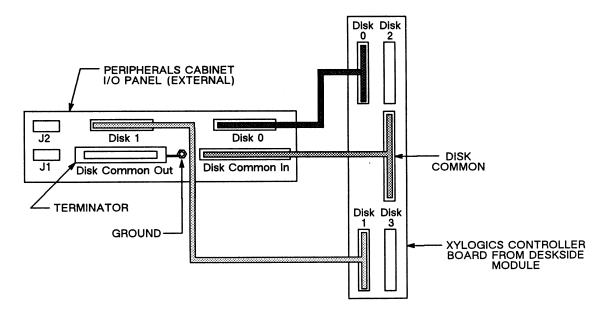
Figure 7-22. 515MB Disk Drive External Cabling, Second Configuration
