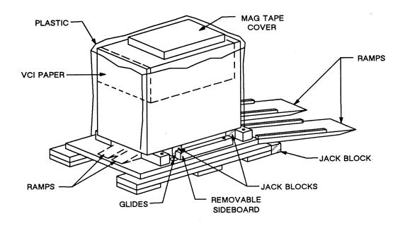
Figure 1-6. Unpacking the CADDServer Peripherals Cabinet
