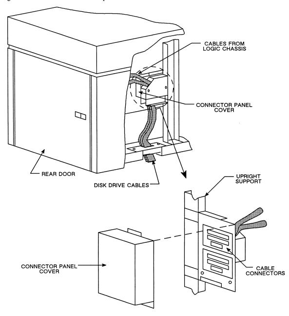
Figure 7-17. 300MB Disk Drive Connector Panel and Cables
