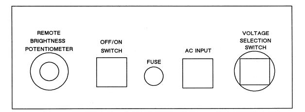
Figure 2-3. Model 30M Voltage Selection through Switch Setting
