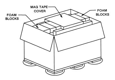
Figure 1-5. Shipping Configuration for the CADDServer Peripherals Cabinet
