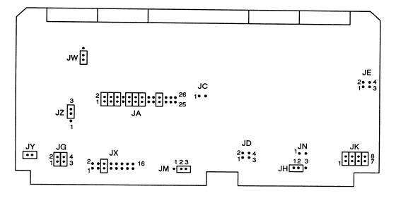
Figure 3-4. Xylogics Model 451 Disk Controller, Revision F, Jumper Configurations
