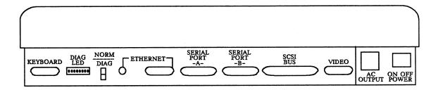
Figure 5-5. Base Unit I/O Panel, Model 30 One-Slot CADDStation
