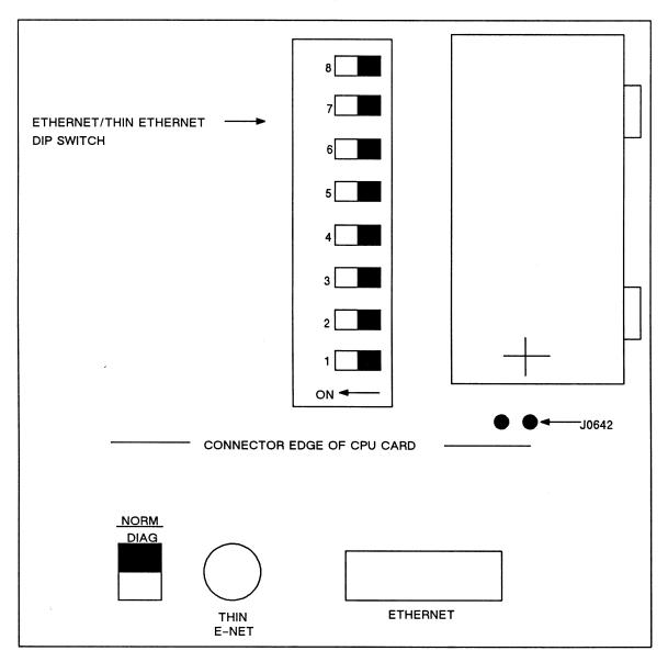
Figure 5-10. Standard Ethenet Dip Switch Setting for Model 30 CADDStation
