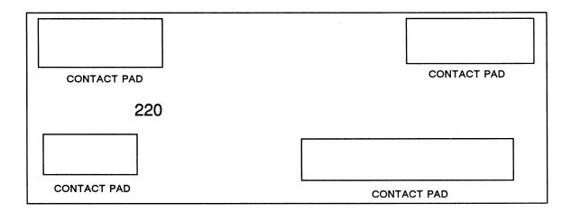
Figure 2-7. Model 30M 220 VAC Voltage Selection through PCB
