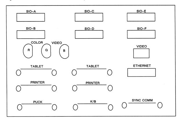
Figure 5-4. Deskside Module I/O Panel, Model 31 Nine-Slot CADDStation
