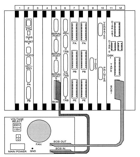
Figure 7-16. Expansion Box Connections for a Diskful CADDStation with a SCSI Board
