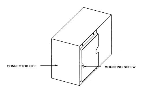
Figure 7-13. Mounting a 170MB Disk Drive
