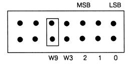
Figure 7-9. Selecting an Installed 170MB Disk Drive as Drive 0, Second Configuration
