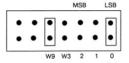
Figure 7-10. Selecting a Second 170MB Disk Drive as Drive 1, Second Configuration
