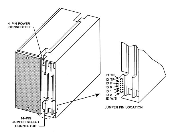
Figure 7-8. 170MB Disk Drive Jumpering Locations, First Configuration
