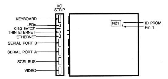
Figure 4-1. Installing the Computervision Host ID PROM on the CPU Board
