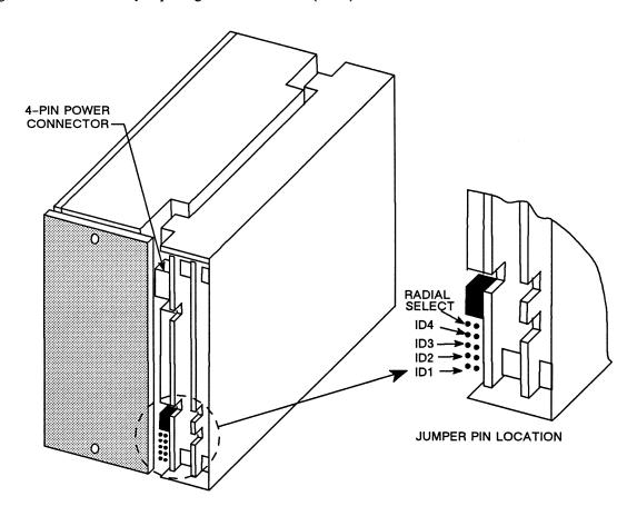
Figure 7-3. 85MB Disk Drive Jumpering Locations
