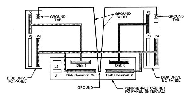
Figure 7-21. 515MB Disk Drive Internal Cabling, Second Configuration
