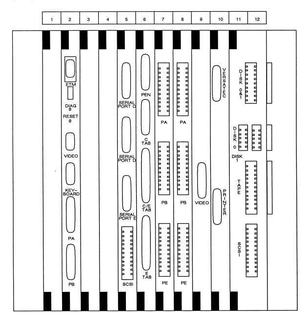
Figure 5-1. Deskside Module I/O Strips, Model 32 12-Slot CADDStation
