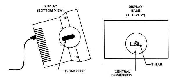
Figure 2-1. Monochrome Graphics Display Assembly
