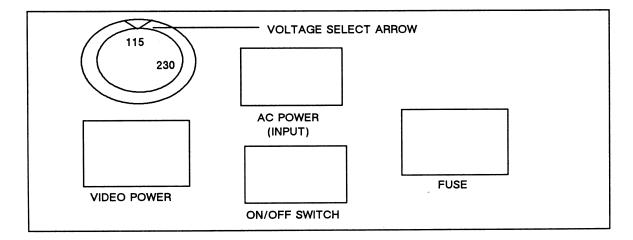
Figure 2-15. Model 30 CADDStation Base Unit Voltage Selection
