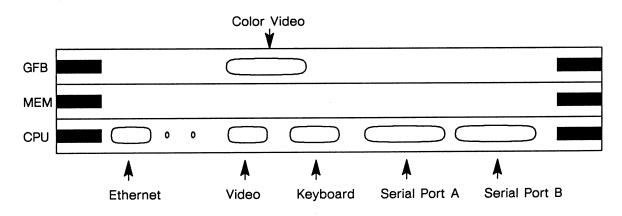
Figure 5-3. Base Unit I/O Strips, Model 32 Three-Slot CADDStation
