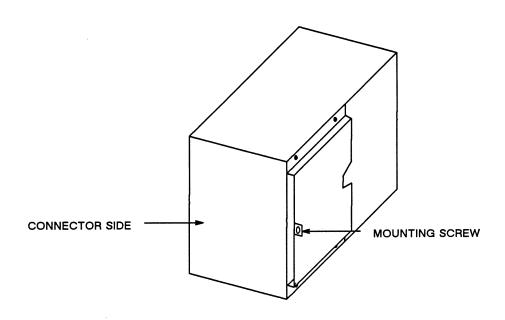
Figure 7-5. Mounting an 85MB Disk Drive
