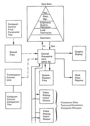
Figure 1. DIMS Data Configuration and Flow
