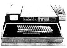
To operate the terminal, the user simply plugs it into an ordinary outlet, folds out the keyboard, pops up the screen, inserts an ordinary telephone into the builtin acoustic coupler and dials his computing center or service bureau. (For more information, circle #70 on the Reader Service Card)
