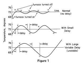
whole cycle repeats as illustrated in Fig. 1. As long as the capacity of the furnace and the outside temperature are within limits, this system maintains the room temperature within several degrees of that set on the thermostat.
