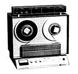
and a marginal error level (operator selected). Standard densities include 800 or 1600 BPI and are operator selectable. A write inhibit feature protects data tapes when the 7900 is in the cleaning mode. The new device uses a self-sharpening, rotating cylindrical blade for tape cleaning and is able to determine whether a reel of tape is computer acceptable, marginal or unacceptable. Options selectable by the operator include: clean only, test only, and combination clean/ test. - SJCC Booth 1000
