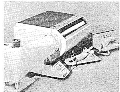
with a Bell System Dataphone, Telecopier II can receive transmission calls automatically and turn on the machine. A new accessory, the Xerox roll feed, will supply paper and carbon for as many as 200 documents.
