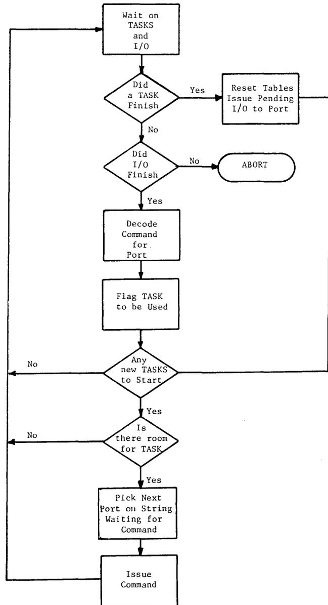
With one exception all MATS tasks are allowed to run concurrently with MATS EXEC. This exception is a utility routine used to examine or rectify faults in the MATS tables. Once a task has been given control, it has access to the necessary tables to allow it to continue processing user requests independently of MATS EXEC. This feature can reduce overhead substantially.
