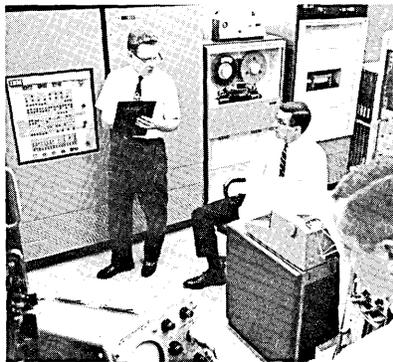
— The IBM 1800 data acquisition and control system (in background) also will be used by engineers and scientists to help design and develop improved space data transmission systems.
