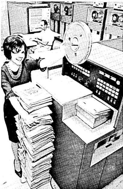
— SSA supervisor Sharon Trieber balances four-foot stack of earnings reports that the optical page reader has condensed onto a single reel of magnetic tape
