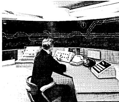
control equipment includes a track-layout display panel and a control console. Reports are printed out on the typewriter at the left. Messages requiring action by the dispatcher are typed in red.
