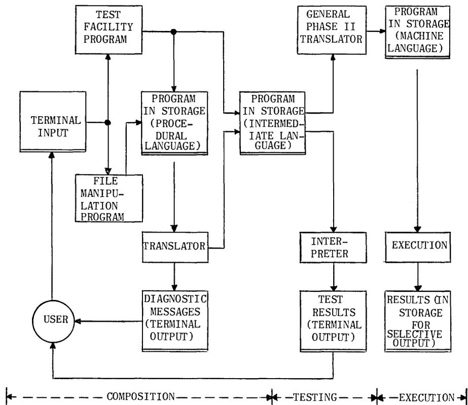
Fig. 2. User Program Flow in a Computing Utility Service
