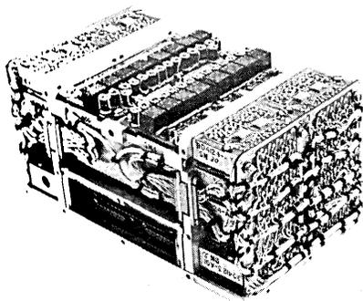
weighs less than 7 pounds and has a volume of only 128 cubic inches. It stores 4096 words of 32 bits each. It also is available with storage capacities of from 256 to 16,384 words, from 8 to 32 bits.
