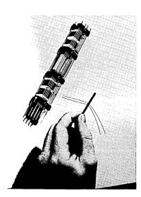
The ferrod (shown at the left), a magnetic current sensing device, is the building block for the scanners used in ESS No. 1. It consists of a ferrite stick around which is wound a pair of solenoid coils. Two wires threaded through holes in the stick carry interrogating and read-out pulses. Two sensors are combined into one unit. Sixteen ferrods may be interrogated simultaneously and their output is sent to Central Control.
