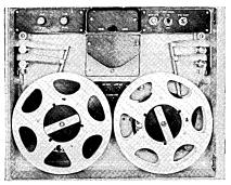
500RM TAPE READER / Photocircuits Corporation — The reader utilizes a printed motor direct capstan drive for tape transport, completely eliminating pinch rollers, brakes and clutches. The 500RM will read at speeds up to 500 characters per second and will Wind/Search at 1000 characters per second. The device will accommodate 5, 6, 7 or 8 level tape and has 8 inch reels. Optional polarities for input and output are available. (For more information, circle 98 on the Readers Service Card.)
