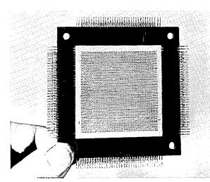
20 MIL FERRITE CORES / Ferroxcube Corporation of America — To meet the increasing demand of high speed memory systems, ferrite core planes and stacks are being produced which make 1 microsecond cycle times for coincident current memory systems possible. These new devices have 20 mil diameter cores with 180 nano-second switching times. They are available in various bit and winding configurations. (For more information, circle 107 on the Readers Service Card.)
