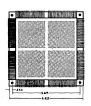
Laminated frame with dip-soldered terminations Four quadrants of 4,096 cores
