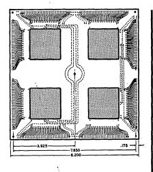
**Printed circuit quad-frame** 4,096 cores per quadrant • 30mil cores on 30-mil centers • Available in choice of three coretypes • Solid copper shielding • We'll stack any number of planes and package the way you want
