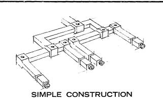
rugged "whiffletree" binary head positioning mechanism combines simplicity with precision . . . eliminates complex servo mechanisms.
