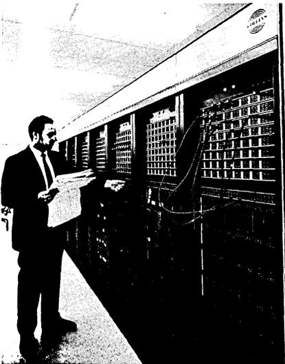
— A Collins systems engineer checks out the line termination or jack units of the Delta Data Central system.
