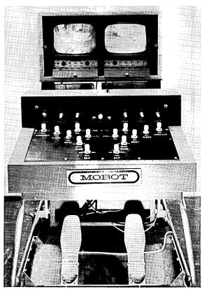
an operator employing a manual control desk similar to those used in remote operation. All of the control signals are recorded on tape. When this tape is played back, the motion sequences are reproduced. Means are provided to ensure that under changing conditions the geometrical paths are reproduced with the desired accuracy.
