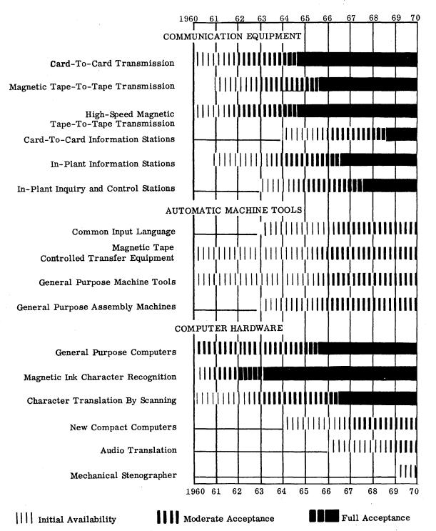
Figure 1 — Timetable for Automation
