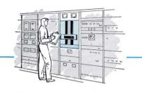
The design of the PB 250 enables it to be mounted as a systems component in 311/2 in. of a standard relay rack.
