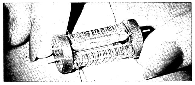
The ferreed, developed at Bell Telephone Laboratories, is a very fast electromechanical switch with metallic contacts, requiring no holding power.
