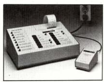
The device features user-adjustable disturbance thresholds, disturbance value printouts, and ambient temperature and dc voltage level monitoring. It allows continuous analysis of line power quality at installation sites. An onsite pot adjustment triggers power disturbance recording. The unit monitors both the dc voltage of power supply and high frequency or spike on the dc supply line via a BNC. The monitor is priced below \$2000. Sola Electric, 1717 Busse Rd, Elk Grove Village, IL 60007.
