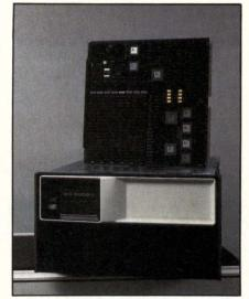
When memory control receives an address from the system cache, the circuitry addresses specific memory locations and performs error checking and correction on data transfers between the bank controller and main memory. It also provides byte parity checking on data transfers from the system cache. Each main memory location is put through a check at a 2-s/Mbyte rate. At the same time, refresh operations are performed on the 64- or 256-Kbit DRAMbased memory array.
