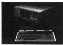
Through a DSA bus, the 2610 provides high speed data transfers essential to complex microprocessor-based devices. Available modules include diagnostic control, micro interface, measurement, and protocol floppy tests. Based on a Z80A micro, hardware consists of a 5-in. CRT, 256 Kbytes of memory, an 89-key tactile keyboard and a 31/2-in. disk drive. Prices start under \$7000. GenRad. Inc. 300 Baker Ave, Concord, MA 01742.
