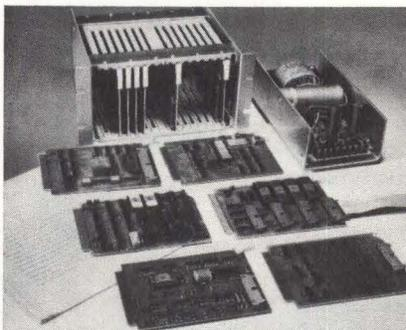
Versatile microprocessing system features bus-oriented backplane, with  $4\frac{1}{2} \times 6\frac{1}{2}$ " cards designed for uniform interfacing. Six individual cards are crate controller (top left), CPU board (top right), 4K ROM/2K RAM (center left), PIA board (center right), ACIA board (bottom left), and Kluge card (bottom right). Omnibin and power supply are also available (top)
