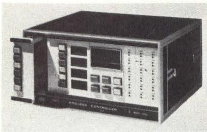
Industrial microcomputer module is housed in a mainframe containing power supply. Various modules contained in the series are (left to right): micro-computer, memory, I/O, set point, display, A-D converter, frequency counter, and D-A converter
