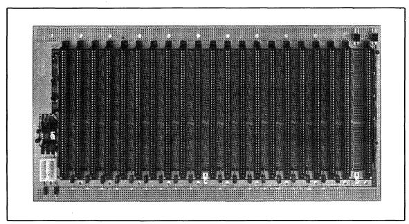
Figure 4: 21-Slot Motherboard
