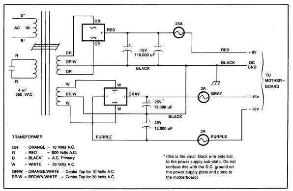
Figure 3: Power Supply Schematic
