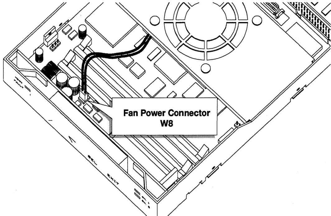
**Figure 1-7: Cooling Fan Power Connection**
