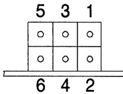
The top row of pins are for connecting external temperature sensor.
