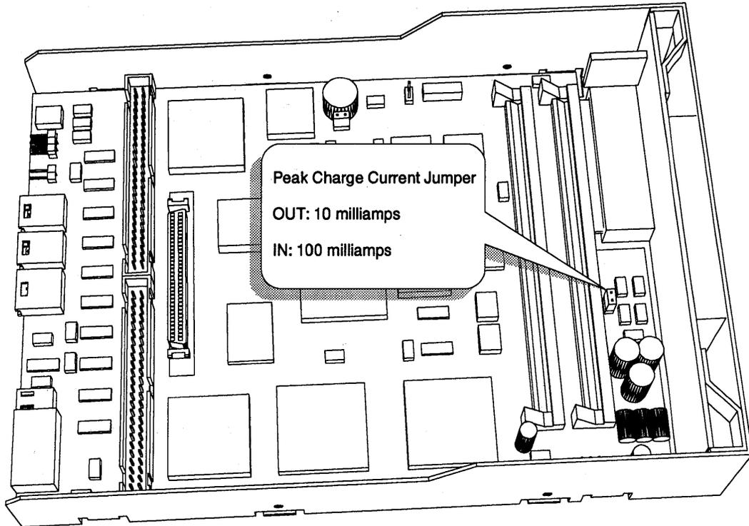
**Figure 1-3: Peak charge current jumper**
