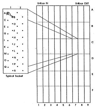
Figure 1: Unibus Wire Wrap Side of Backplane
