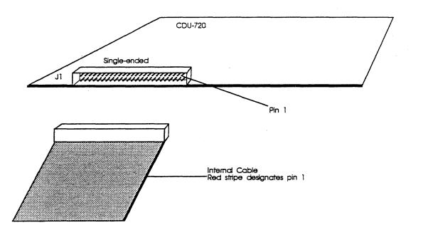
Figure 3-4: CDU-720 cable connection
