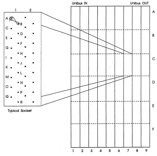
Figure 3-3: Unibus Wire Wrap Side of Backplane
