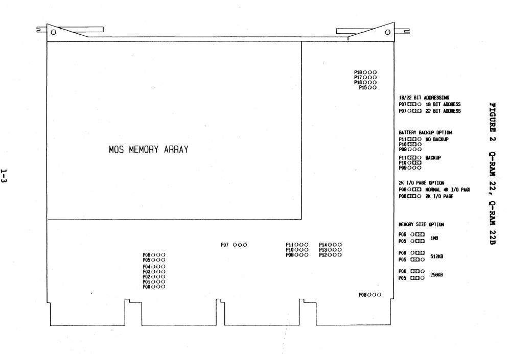
When any byte of data is written to Q-RAM 22(B) boards which contain parity, a parity bit is generated which is stored along with the byte of data in the memory array. Whenever a byte of data is read the parity logic checks it against the stored parity bit. If parity is bad, an error has occurred and data is asumed to be bad.
