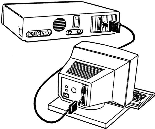
**Figure 2-4. Connecting to a Local Computer**
