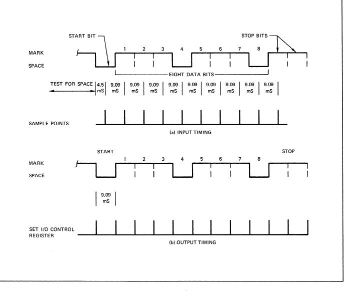
Figure 2-2. Serial I/O Timing
