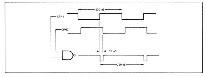
Figure 3-2. Relationship of Control Signals CPH1 and CPH2/
