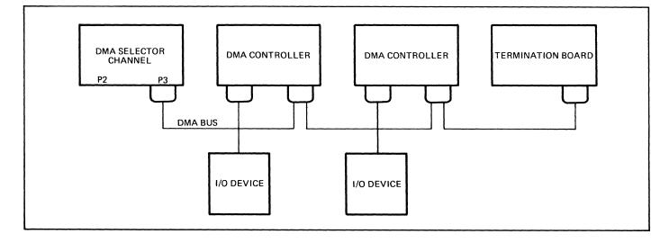
Figure 4-5. DMA Bus Cabling for Multiple Controllers
