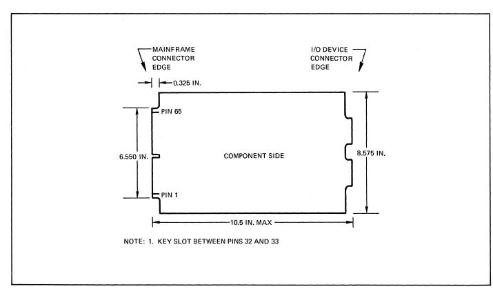
Figure 1-3. Interface Circuit Board Dimensional Data
