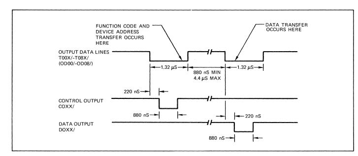
Figure 3-3. Data or Function Output Timing
