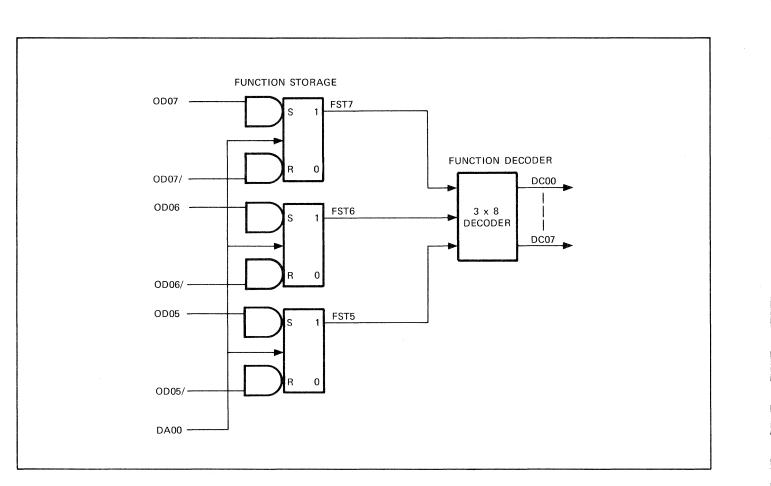
Figure 3-5. Function Output Storage and Decoding Logic
