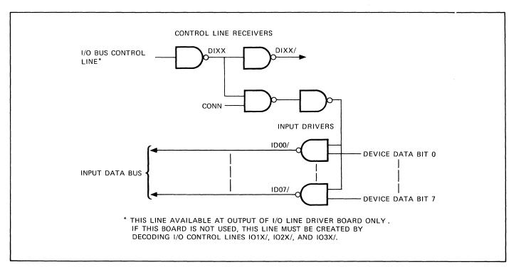
Figure 3-7. Data Input Logic
