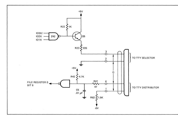
Figure 2-1. Serial I/O Interface Circuit
