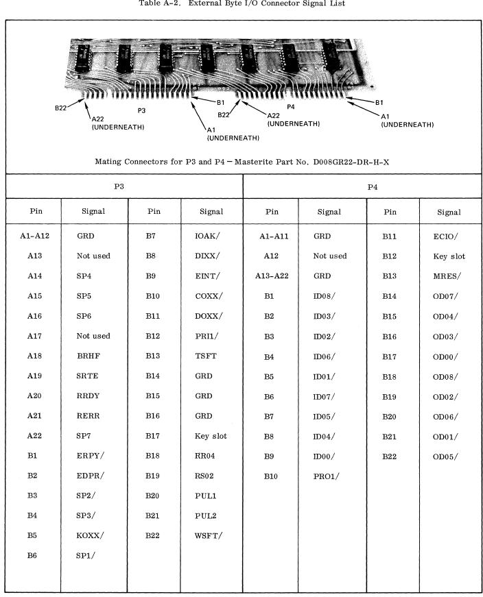
Table A-2. External Byte I/O Connector Signal List
