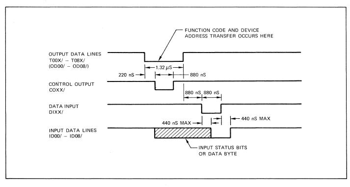
Figure 3-6. Data or Status Input Timing
