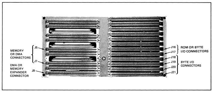
Figure 1-2. Mainframe Chassis Interface Connectors
