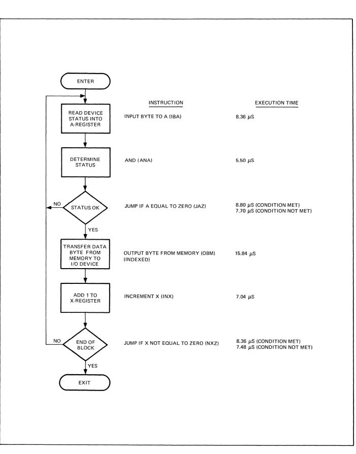
Figure 3-9. Typical Program-Controlled Transfer Sequence
