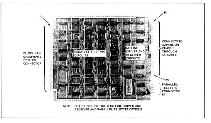
Figure 1-4. I/O Line Driver and Receiver Interface Option
