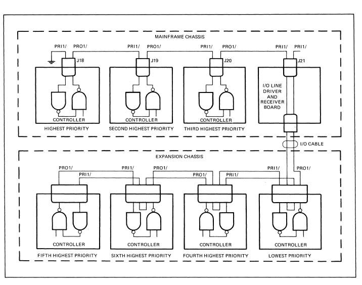
Figure 3-12. Typical Priority Wiring Scheme
