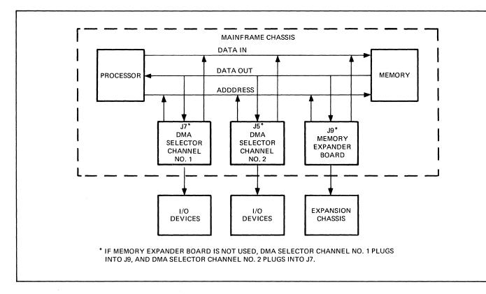
Figure 4-1. Relationship of Processor, Memory, and DMA Channels
