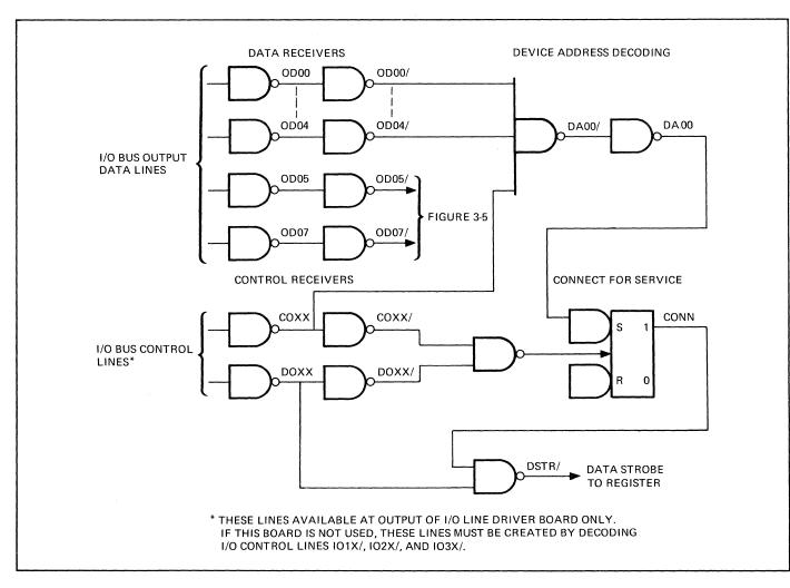
Figure 3-4. Data Output Logic
