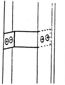
Figure 1-5 Card Cage Retainer
