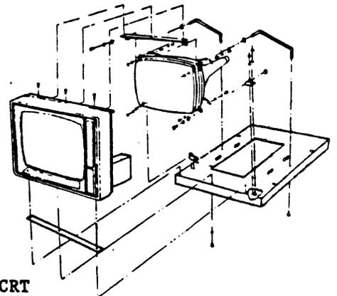
Figure 1-18 Bezel Assembly and CRT
