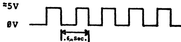
VERTICAL OUTPUT (SET SCOPE TO 5V/DIV, 1m SEC/DIV)
