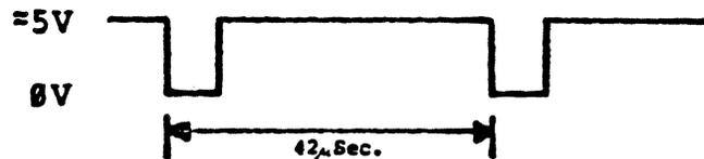
RED, GREEN AND BLUE VIDEO OUTPUT WITH A WHITE (ERASE PAGE) SCREEN, SET BRIGHTNESS POT TO FULL INTENSITY (SET SCOPE TO 1V/DIV, 10uSEC/DIV)
