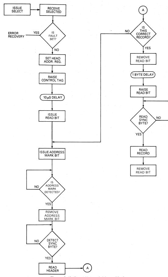
Figure 8-13. Read Using Address Marks
