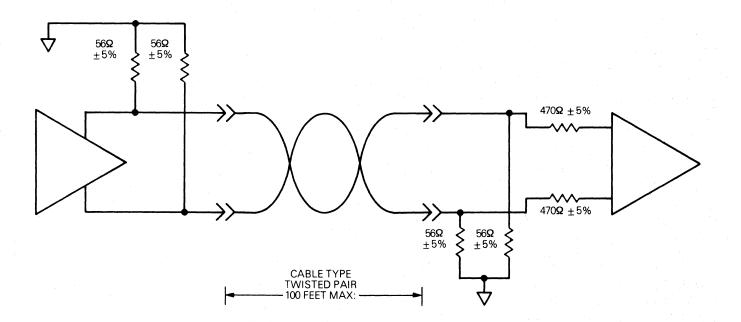
Figure 9-1. Bussed (Signal) Cable Recommended Driver/Receiver Cable Termination Circuit
