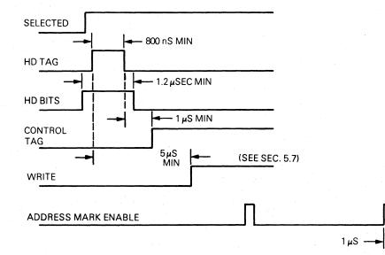
Figure 8-5. Initializing for Address Mark Sectoring
