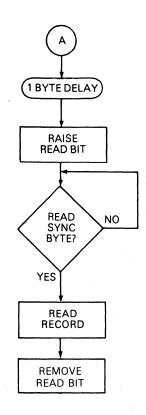
Figure 8-8. Read Using Electronic Sectoring
