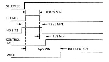
Figure 8-4. Initializing for Electronic Sectoring (Format A)
