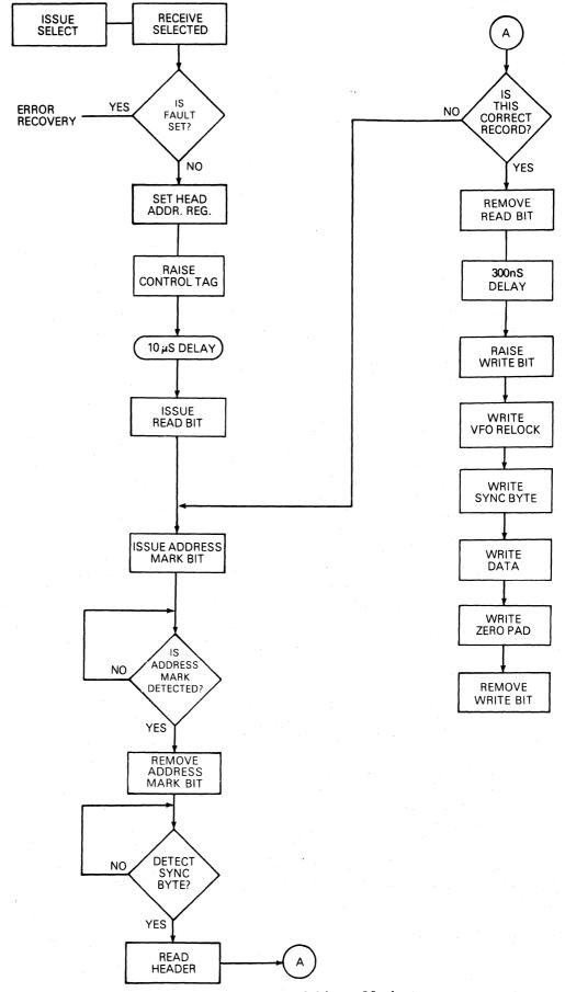
Figure 8-10. Write Using Address Marks
