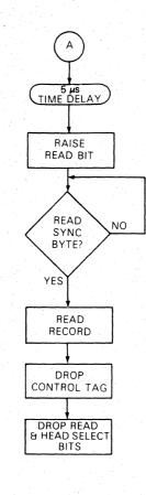
Figure 5-5. Read Electronic Sectoring
