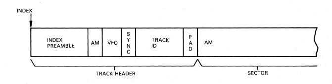
Figure 3-4. Address Mark/Track Header with Track ID Field
