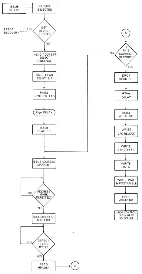
Figure 5-6. Write Using Address Marks
