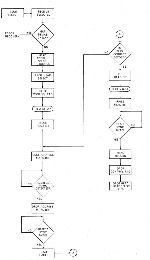
Figure 5-7. Read Using Address Marks
