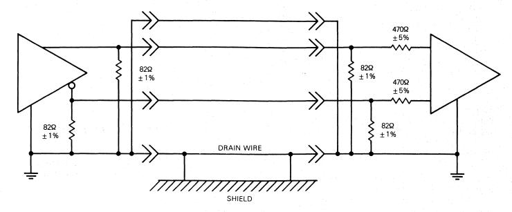
50 FT. MAX. OF FLAT CABLE HAVING 130  $\pm$  13 OHMS CHARACTERISTIC IMPEDANCE.
