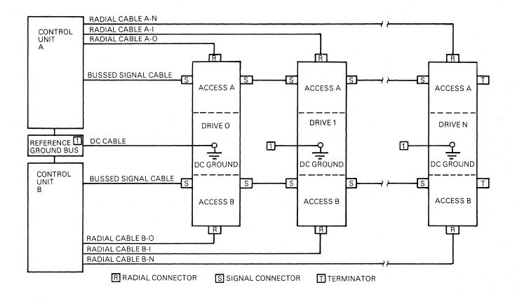
Figure 6-6. Dual Access Cabling, Daisy Chain Configuration
