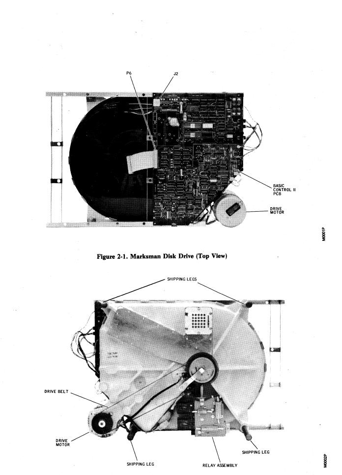
Figure 2-2. Marksman Disk Drive (Bottom View)
