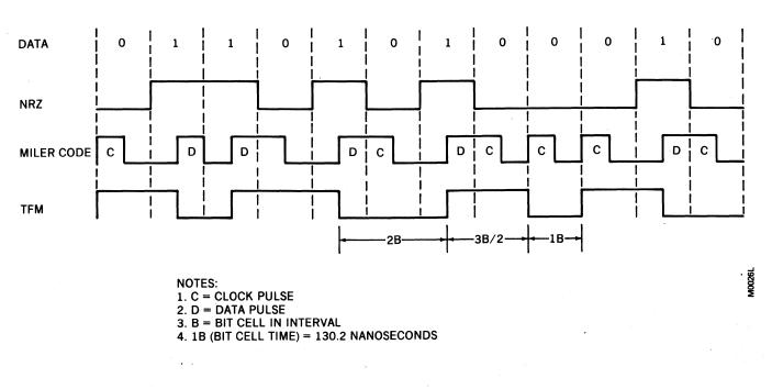
Figure 3-6. Code Format Comparisons and TFM Characteristics
