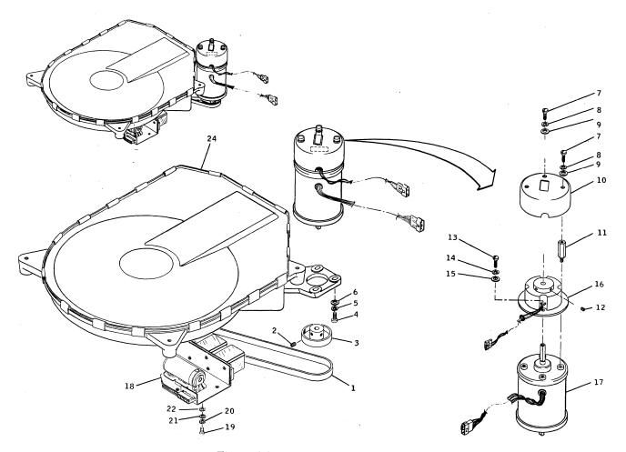
Figure 6-3. Wired Drive Assembly
