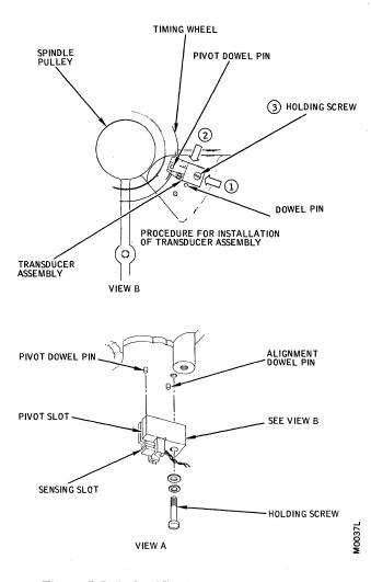
Figure 5-5. Index/Clock Transducer Assembly
