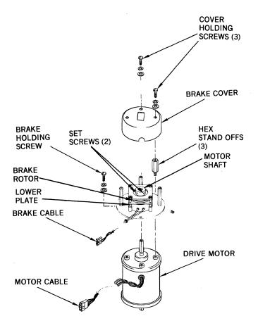
Figure 5-3. Brake Assembly
