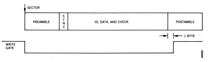
Figure 2-20. Imbedded ID Field Write Timing
