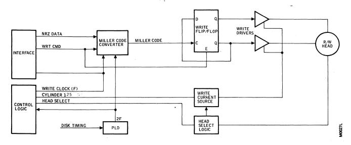
Figure 3-7. Write Data System Block Diagram
