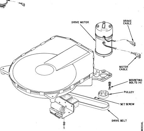
Figure 5-2. Drive Motor Assembly
