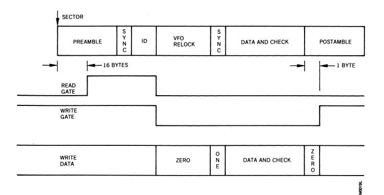
Figure 2-19. Non-Imbedded ID FIeld Write Timing
