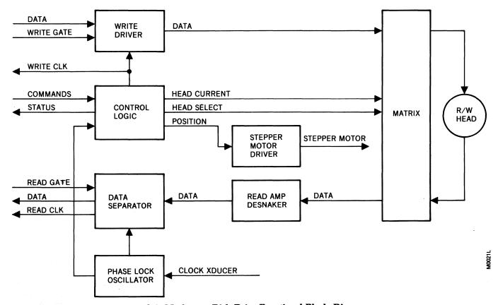
Figure 3-1. Marksman Disk Drive Functional Block Diagram
