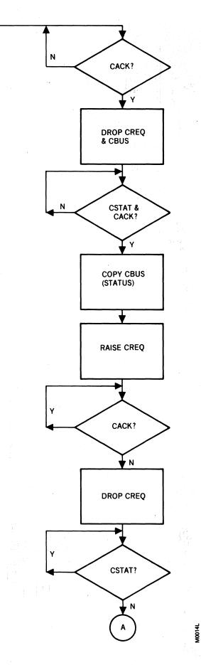
Figure 2-14. Two Byte Commands Flow Chart
