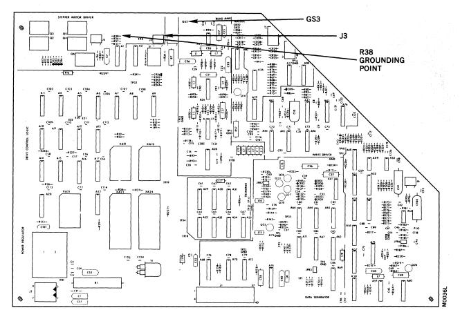
Figure 5-4. Brake Adjustment Jumper Location
