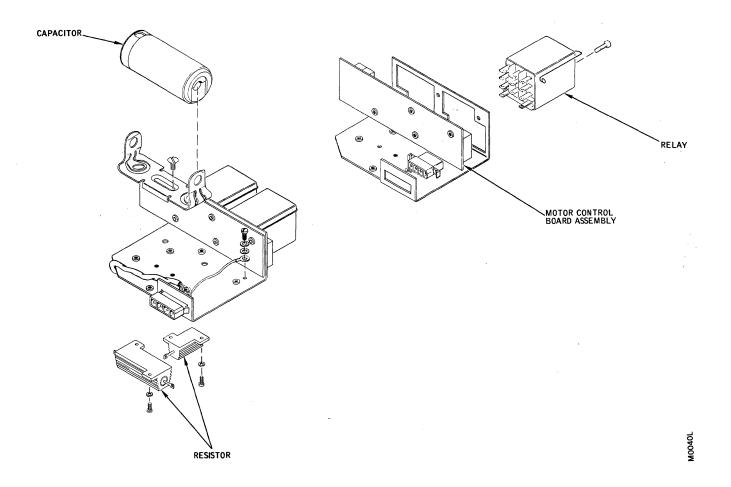
Figure 5-8. Control Relay Assembly
