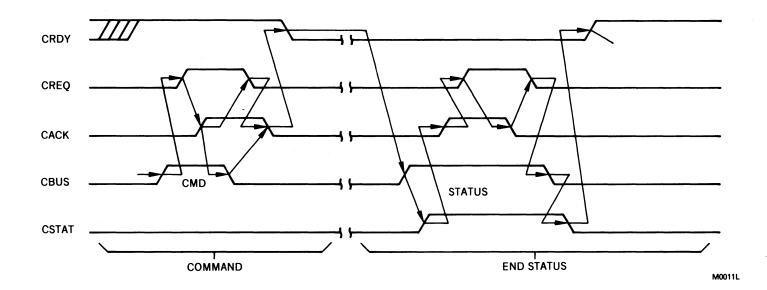
Figure 2-11. One Byte Commands (Except head advance) Timing Diagram
