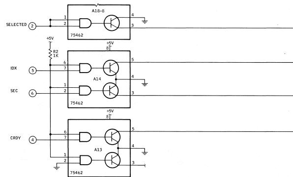
Figure 4-1. Driver/Receiver II Logic Diagram (Sheet 3)
