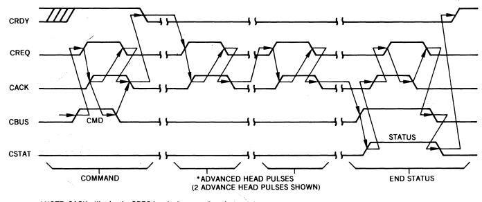
\*NOTE: CACK will echo the CREQ head advance pulses, but can rise after CREQ has dropped if CREQ is very narrow. (The head advance operation is still performed prior to the rise of CACK). CREQ for head advance, should be at least 2 μs wide.
