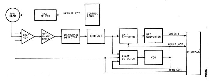
Figure 3-8. Read Data System Block Diagram
