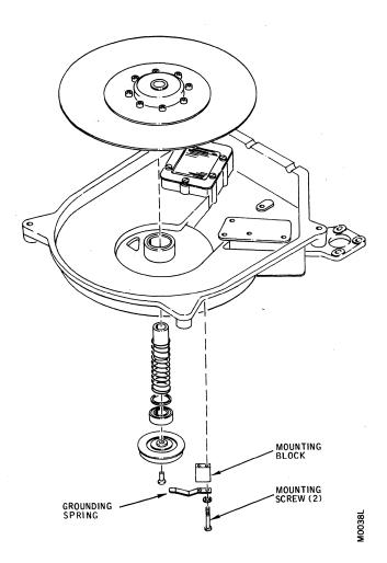
Figure 5-6. Grounding Spring Assembly
