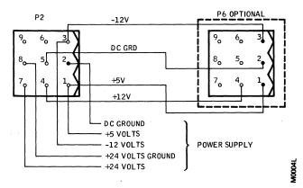
**Figure 2-4. DC Voltage Connections**
