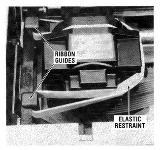
Figure 1-2 Remove Head Restraint
