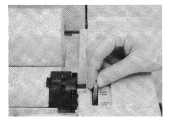
Figure 2-6C Control Lever to FRICTION
