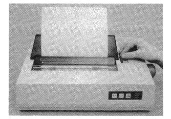
Figure 2-4C Lever to Friction Position
