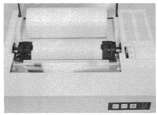
Figure 2-6B Tractors Closed on Roll Paper
