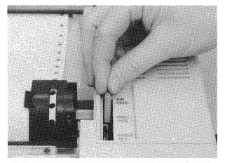
Figure 2-5D Lever To PIN FEED Position
