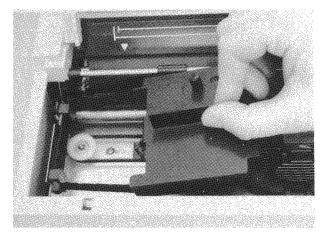
Figure 2-3A Looping the Ribbon onto the Left Ribbon Guides
