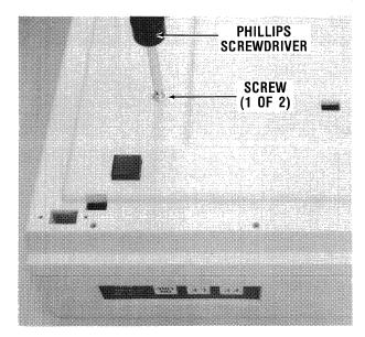
Figure 1-1 Remove Bottom Screws (2)
