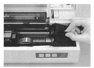
Figure 2-3B Seating the Ribbon Cassette into the Right End of the Printer
