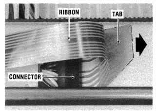
Figure 5-2 Flexible Ribbon Connector
