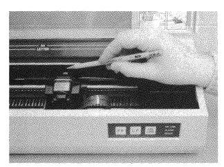
Figure 2-3C Inserting Ribbon at Print Head
