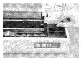
Figure 2-3D Tightening the Ribbon (Knob)
