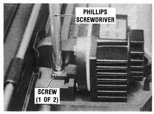
Figure 5-1 Print Head Mounting Screws (2)
