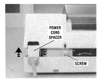
Figure 2-8 Left Rear View of Printer
