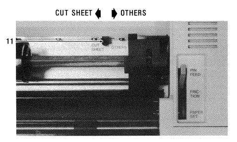
Figure 2-2B Cut Sheet/Others Switch (Paper End Alarm Control)
