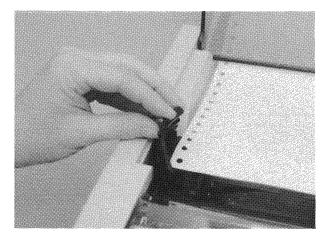
Figure 2-5C Engaging Left Sprocket
