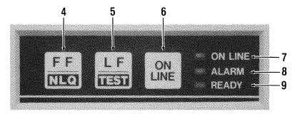
Figure 2-1B Control Panel Switches and Indicators
