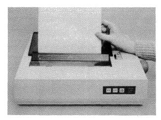
Figure 2-4B Inserting Sheet Paper
