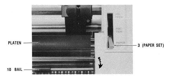
Figure 2-2A Internal Controls
