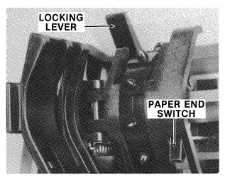
Figure 2-5A Left Tractor Controls
