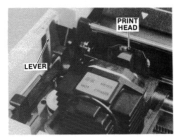
Figure 2-3C Print Head Position Control Lever
