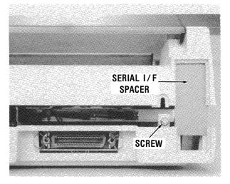
Figure 2-9 Right Rear View of Printer
