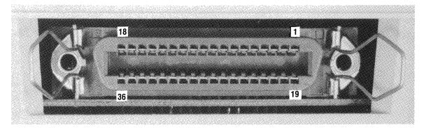
Figure B-1 36-Pin Female Connector (Centronics P/N 31310012-1016)
