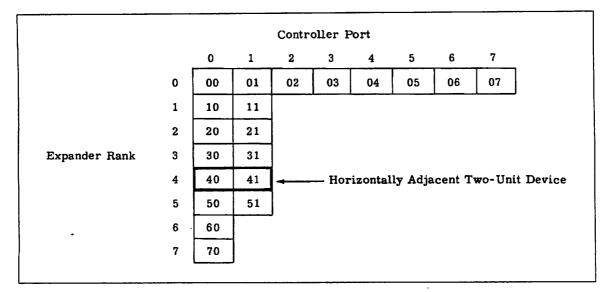
Figure 3-4. Horizontally Adjacent Two-Unit Device
