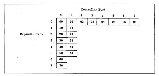
Figure 3-2. 844 Expander Configuration With 20 Drives
