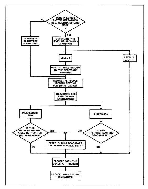
Figure 13-1. Deadstarting a Machine in a Multimainframe Complex
