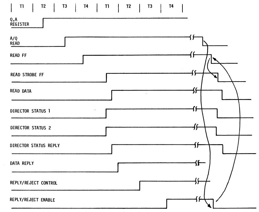
Figure 4-2. A/Q Read/Reply Timing Diagram
