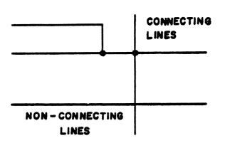
Lines connected to a common point or at a junction point are shown in the upper part of this illustration. No more than four lines are connected to a common point in the diagrams.
