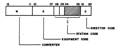
Figure 2-1. Q Register Format
