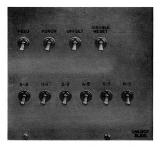
Figure 10. Maintenance Switch Panel
