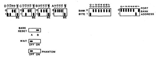
In the last diagram memory groups A and B are bank-independent and located in the last 8K of memory. Groups C and D reside in bank 2 between 12K and 20K. The bank port address is 40h. Only groups A and B are enabled on start-up and reset. Phantom and Wait are enabled.
