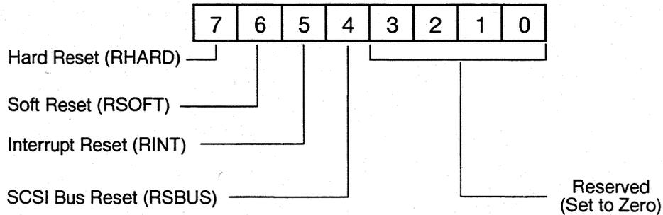
Figure 4-1. Control Register (Write)
