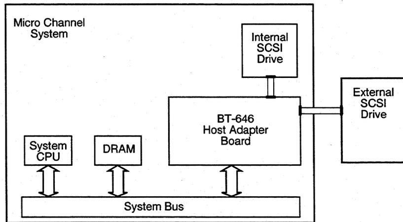
Figure 1-1. System Architecture
