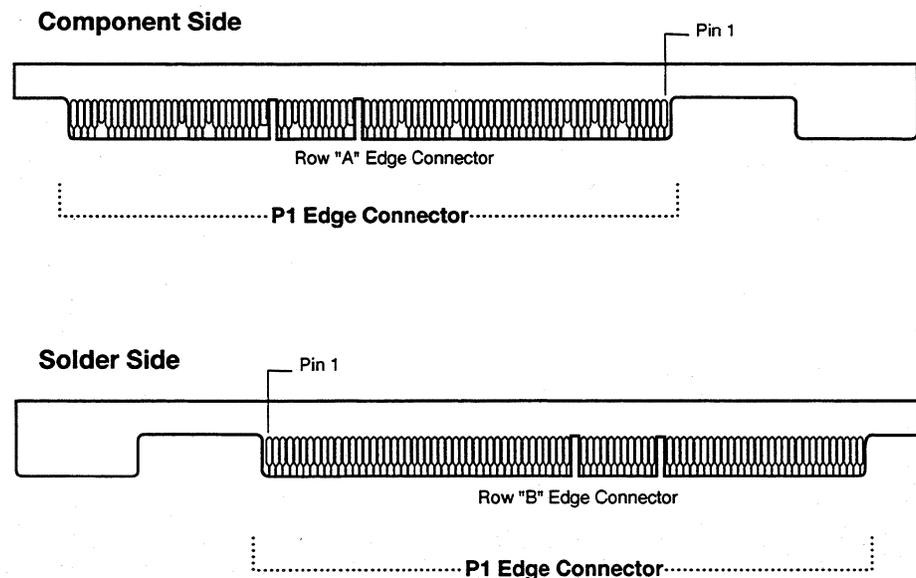
Figure 3-1. Connector Rows on the BT-646 Board Edge
