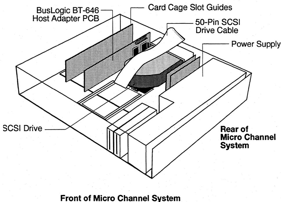
3. Remove the mounting screw and the existing bracket from the rear panel behind the 16-bit or 32-bit slot that has been selected for insertion of the BT-646. The Micro Channel slot closest to the internal hard drive(s) is the best choice.
