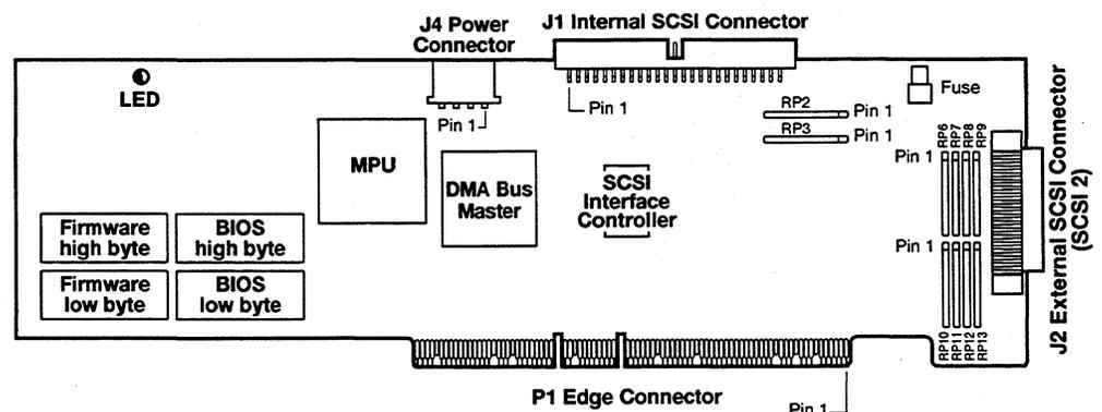
Figure 2-1. The BT-646 Host Adapter Board
