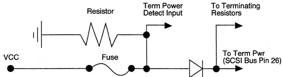
**Figure 3-2. Terminator Power Schematic**
