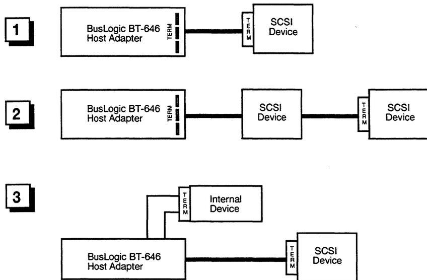
**Figure 2-2. SCSI Terminator Configurations**
