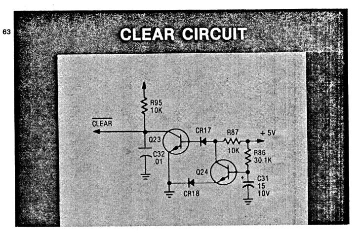
AT POWER ON, Q24 IS HELD ON UNTIL CAPICATOR C31 HAS CHARGED THROUGH RESISTOR R86. Q23 IS HELD ON WITH Q24 CAUSING CLEAR/ TO REMAIN LOW UNTIL CAPACITOR C31 HAS CHARGED. CLEAR/ REMAINS LOW FOR APPROXIMATELY 0.1 SECOND AFTER THE +5 VOLT LEVEL IS ESTABLISHED.
