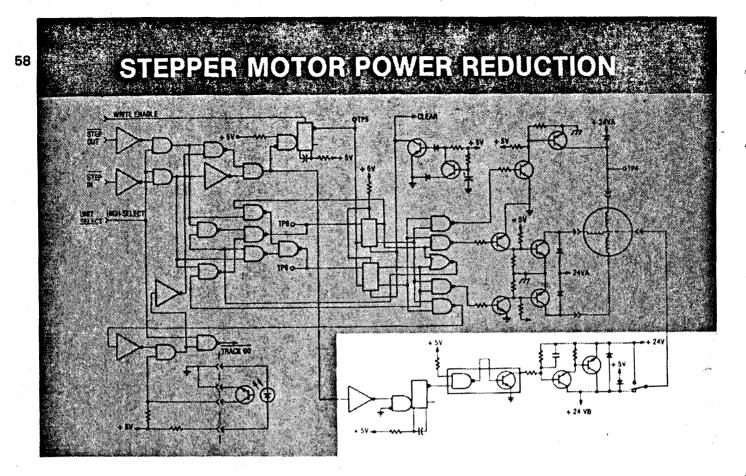
THE POWER SUPPLIED TO THE STEPPER MOTOR IS CONTROLLED BY THE STEPPER MOTOR POWER REDUCTION LOGIC. AS MENTIONED EARLIER, THE POWER SUPPLIED TO THE MOTOR WHEN IT IS NOT MOVING MUST BE REDUCED TO AVOID OVERHEAT-ING.
