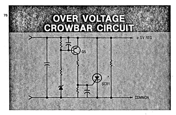
THE CROWBAR CIRCUITS FOR BOTH THE +5 VOLT AND -12 VOLT SUPPLIES ARE IDENTICAL EXCEPT FOR COMPONENT VALUES. IF THE SAFE VOLTAGE DETERMINED BY THE ZENER DIODE IS EXCEEDED, TRANSISTOR Q5 IS SWITCHED ON FIRING SCR1 TO SHORT CIRCUIT THE SUPPLY. THE RESULTANT OVER CURRENT CONDITION CAUSES THE REGULATOR CIRCUIT TO SHUT DOWN.
