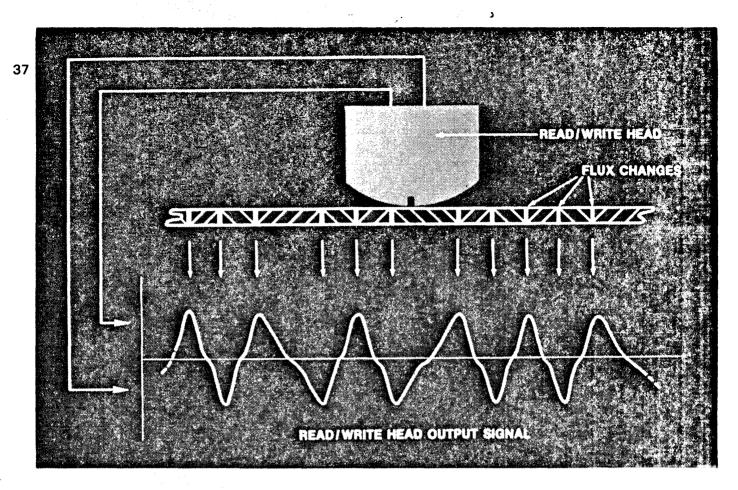
ONE BITS AND CLOCK BITS ARE REPRESENTED BY A CHANGE IN DIRECTION OF MAGNETIC FLUX RECORDED IN THE OXIDE COATING ON THE DISKETTE. WHEN THE DISKETTE ROTATES UNDER THE READ/WRITE HEAD DURING A READ OPERATION, THESE FLUX CHANGES PRODUCE EITHER POSITIVE OR NEGATIVE GOING PEAKS IN THE OUTPUT FROM THE READ/WRITE HEAD DEPENDING ON THE DIRECTION OF THE FLUX CHANGE.
