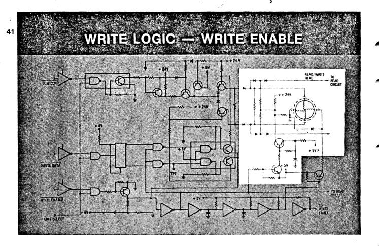
THE WRITE ENABLE LOGIC IS BASICALLY THE SAME AREA OF LOGIC DESCRIBED EARLIER IN THE READ LOGIC SECTION OF THIS LECTURE. AS YOU WILL REMEMBER, THE WRITE ENABLE LOGIC DETERMINES WHETHER THE READ/WRITE IS READ OR WRITE ENABLED ACCORDING TO THE CONDITION OF THE HOST SYSTEM CONTROL-LER SIGNAL WRITE ENABLE.
