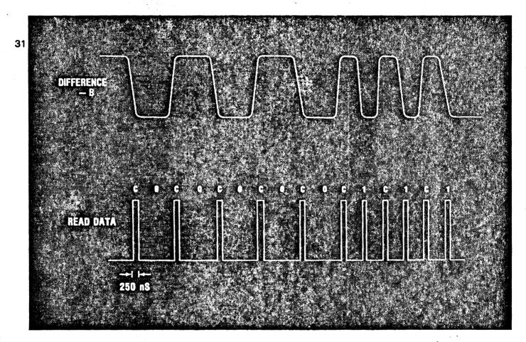
THE DIFFERENCE SIGNAL, IN WHICH BOTH CLOCK AND ONE BITS ARE REPRESENTED BY TRANSITIONS, IS INPUT TO A ONE SHOT MULTIVIBRATOR WHICH IS TRIGGERED TO PRODUCE A POSITIVE OUTPUT PULSE FOR BOTH NEGATIVE AND POSITIVE GOING INPUT PULSES. THESE 250 NANOSECOND OUTPUT PULSES BECOME THE DIGITAL INTERFACE SIGNAL, "READ DATA."
