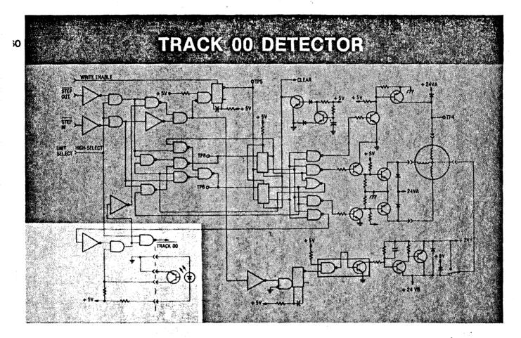
THIS DIAGRAM HIGHLIGHTS THE TRACK 00 DETECTOR LOGIC WHICH ESTABLISHES THAT THE READ/WRITE HEAD IS AT TRACK 00.
