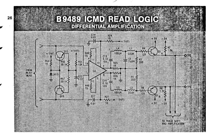
THE DIFFERENTIAL AMPLIFIER IS A MULTI-STAGE CIRCUIT THAT CONSISTS OF A DIFFERENTIAL VIDEO AMPLIFIER U4 AND THE DUAL PACKAGED TRANSISTORS Q1A AND Q1B. THE GAIN OF THE AMPLIFIER IS PRESET BY THE VALUE OF THE RE-SISTORS R49 AND R48. NOTICE THAT THE VALUE OF THESE RESISTORS IS INDICAT-ED BY THE LETTERS "TS." TS MEANS THE VALUES ARE TEST SELECTED. DETAILED PROCEDURES FOR ESTABLISHING THE CORRECT VALUES FOR THESE COMPONENTS, IN CASE REPLACEMENT IS NECESSARY, ARE DESCRIBED IN A LATER LECTURE.
