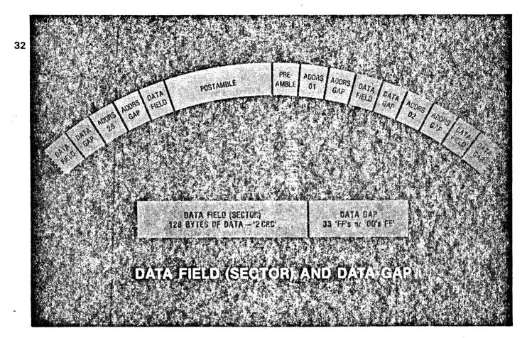
AFTER THE DATA SYNCH MARK CHARACTER "FB" IN THE ADDRESS GAP FIELD COMES THE DATA FIELD OR SECTOR. THIS CONSISTS OF 128 BYTES OF DATA FOLLOWED BY TWO CRC CHARACTERS TO CHECK THAT DATA READ BACK FROM THE DATA FIELD IS CORRECT.
