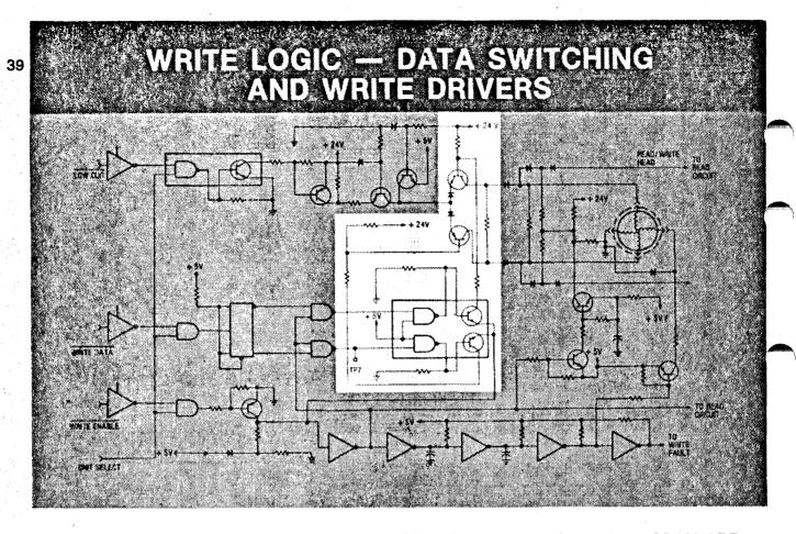
THE DATA SWITCHING AND WRITE DRIVERS, HIGHLIGHTED IN THIS DIAGRAM ARE THE NEXT STAGE IN THE WRITE LOGIC. THE DATA SWITCHING DRIVERS CONTROL THE CONDUCTION OF THE WRITE DRIVERS WHICH IN TURN PROVIDE CURRENT TO THE WRITE HEAD.
