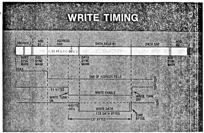
THE TIMING OF A WRITE OPERATION IS DETERMINED BY THE HOST SYSTEM CON-TROLLER. THIS TIMING DIAGRAM SHOWS THE WRITE SEQUENCE FOR SECTOR ONE WHICH IS BASICALLY THE SAME FOR ALL OTHER SECTORS.
