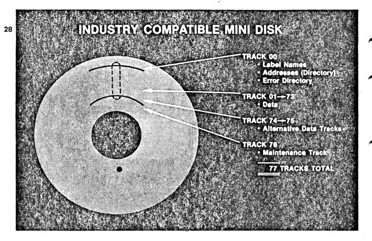
THE REMAINING TRACK IS THE FIRST PHYSICAL TRACK ON THE DISK, TRACK 00, WHICH CONTAINS DESCRIPTIVE INFORMATION ABOUT THE DATA RECORDED ON THE DISKETTE. THIS INFORMATION INCLUDES THE LABEL NAMES OF FILES WRITTEN ON THE DISKETTE, THE DISKETTE ADDRESSES TO INDICATE WHERE THE FILES ARE LOCATED, THE ERROR DIRECTORY, ETC. YOU CAN FIND A DETAILED DESCRIPTION OF THE CONTENT OF THE INDEX TRACK IN SECTION 1 OF THE FIELD ENGINEERING TECHNICAL MANUAL.
