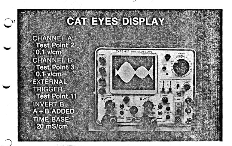
CHECK THE ALIGNMENT ADJUSTMENT USING AN OSCILLOSCOPE AND THE PROCE-DURE IN THE TECHNICAL MANUAL.
