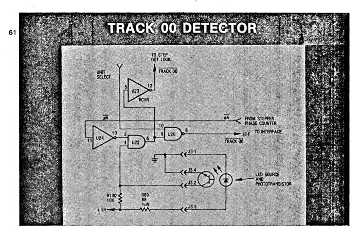
THE BOTTOM RIGHT OF THE DIAGRAM SHOWS THE "LED" LIGHT SOURCE AND PHOTO TRANSISTOR WHICH COMPRISE THE OPTICAL DETECTOR. A METAL TAB ON THE READ/WRITE HEAD CARRIAGE ASSEMBLY INTERRUPTS THE BEAM OF LIGHT WHEN THE READ/WRITE HEAD IS AT TRACK 00.
