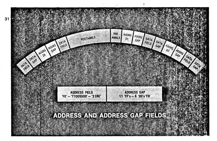
THE FIRST ADDRESS FIELD FOLLOWS THE PREAMBLE AND CONTAINS THE ADDRESS OF THE FIRST DATA FIELD. IN THE FORMAT SHOWN IN THE DIAGRAM, "TT" RE-PRESENTS THE TRACK ADDRESS IN THE RANGE 00 THROUGH 76, "00" IS A SEPARA-TOR "SS" REPRESENTS THE SECTOR, THAT IS DATA FIELD ADDRESS, "00" IS AN-OTHER SEPARATOR FOLLOWED BY TWO CYCLIC REDUNDANCY CHECK (CRC) CHARACTERS.
