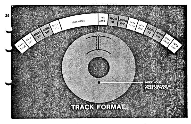
THE START OF A TRACK IS INDICATED TO THE MINI DISK CONTROLLER IN THE HOST SYSTEM BY THE SIGNAL "INDEX" AS THE INDEX HOLE PASSES THE OPTICAL SENSOR, WHICH IS 180 DEGREES FROM THE READ/WRITE HEAD.
