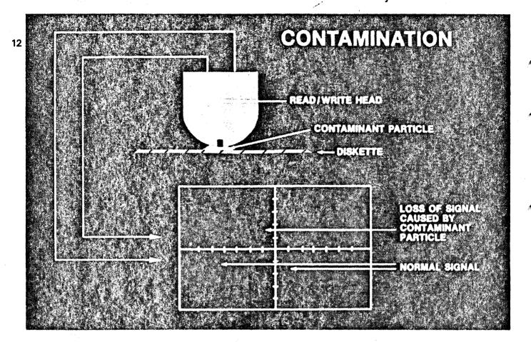
THE SECOND TYPE OF DAMAGE, CONTAMINATION, IS CAUSED BY PARTICLES OF DIRT ON THE MAGNETIC OXIDE SURFACE OF THE DISKETTE. AS WITH PHYSICAL DAMAGE, CONTAMINATION CAN CAUSE THE READ/WRITE HEAD TO LOOSE CLOSE CONTACT WITH THE MAGNETIC OXIDE RECORDING SURFACE OF THE DISK RESULTING IN A LOSS OF SIGNAL DURING A READ OPERATION OR, BADLY RECORDED DATA DURING A WRITE OPERATION.
