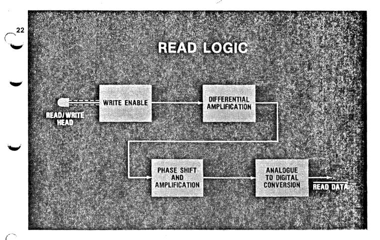
THE READ LOGIC CONSISTS OF FOUR MAIN FUNCTIONAL BLOCKS, WRITE ENABLE; DIFFERENTIAL AMPLIFICATION; PHASE SHIFT AND AMPLIFICATION; AND ANALOGUE TO DIGITAL CONVERSION. WE WILL HIGHLIGHT AND DESCRIBE EACH OF THESE FOUR FUNCTIONAL BLOCKS TO EXPLAIN THE OPERATION OF THE READ LOGIC IN DETAIL.
