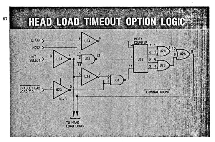
THE HEAD LOAD TIMEOUT OPTION IS DESIGNED TO ALLOW THE HEAD TO REMAIN LOADED FOR EIGHT INDEX TIMES, THAT IS DISKETTE REVOLUTIONS, AFTER THE DRIVE HAS BEEN DESELECTED. IN ORDER TO UTILIZE THIS FEATURE, THE COMMAND "ENABLE HEAD LOAD TIME-OUT" MUST BE RECEIVED PRIOR TO THE END OF THE "HEAD LOAD" SIGNAL AND THE DRIVE BEING DESELECTED.
