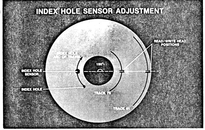
THE REMAINING ICMD ADJUSTMENT IS FOR THE INDEX HOLE SENSOR ASSEMBLY WHICH MUST BE LOCATED 180 DEGREES FROM THE READ/WRITE HEAD AND ALIGN WITH THE ARC OF TRAVEL OF THE INDEX HOLE IN THE DISKETTE.
