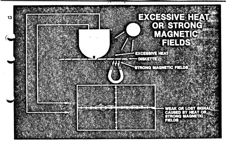
THE THIRD TYPE OF DAMAGE IS LOSS OF DATA RECORDED ON THE MAGNETIC OXIDE CAUSED BY EXPOSURE TO STRONG MAGNETIC FIELDS OR EXCESSIVE HEAT. STRONG MAGNETIC FIELDS CAN ERASE THE MAGNETICALLY RECORDED DATA ON THE DISK-ETTE CAUSING LOSS OF SIGNAL DURING A READ OPERATION. EXCESSIVE HEAT CAN BOTH ERASE MAGNETICALLY RECORDED DATA AND CAUSE PHYSICAL DISTORTION OF THE DISK.
