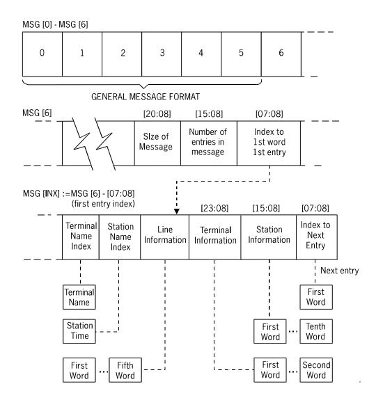
Figure 6–1. INTERROGATE STATION ENVIRONMENT RESULT Index Diagram
