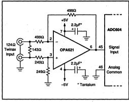
FIGURE 8. Differential Input Buffer Amplifier (Gain = -1V/V).
