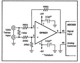
FIGURE 9. Differential Input Buffer Amplifier (Gain = -1V/V).
