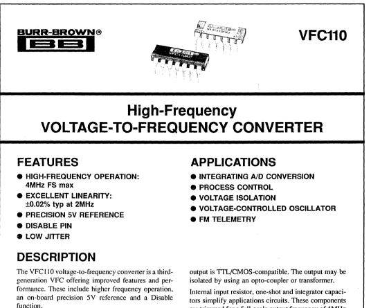
The precision 5V reference can be used for offsetting the VFC transfer function, as well as exciting transducers or bridges. The Enable pin allows several VFCs' outputs to be paralleled, multiplexed, or simply to shut off the VFC. The open-collector frequency Internal input resistor, one-shot and integrator capacitors simplify applications circuits. These components are trimmed for a full-scale output frequency of 4MHz at 10V input. No additional components are required for many applications.
