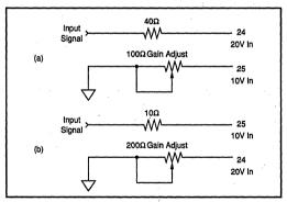
FIGURE 6. Optional Gain Adjust: (a) ±10VBipolar Operation, (b) ±15V Bipolar or 0 to -10V Unipolar Operation
