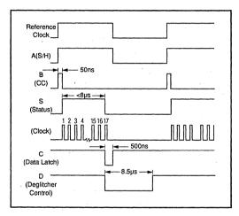
FIGURE 5. Timing Diagram for Figure 4.
