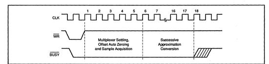
FIGURE 2. Converter Timing.
