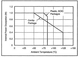
FIGURE 4. Maximum Power Dissipation.
