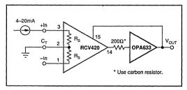
FIGURE 16. 4–20mA Receiver with Output Current Boosted to  $\pm 100$ mA.
