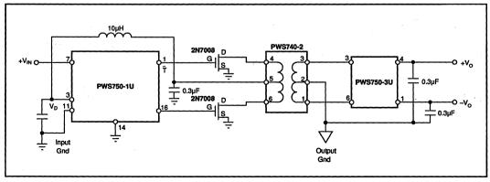
FIGURE 8. 1500VAC Isolation Using PWS740-2 Transformer.
