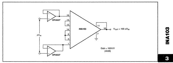
FIGURE 17. Gain-of-100 INA103 with FET Buffers.
