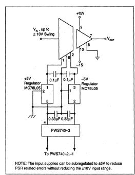
FIGURE 10. Improved PSR Using External Regulator.
