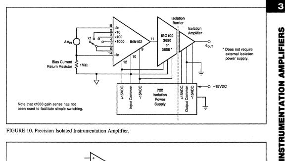
FIGURE 10. Precision Isolated Instrumentation Amplifier.
