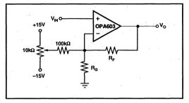
FIGURE 6. Offset Voltage Adjustment.
