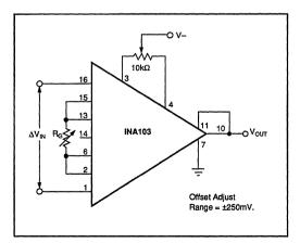
FIGURE 3. Offset Adjustment Circuit.
