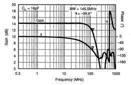
A<sub>v</sub> = +2V/V CLOSED-LOOP SMALL SIGNAL BAND WIDTH
