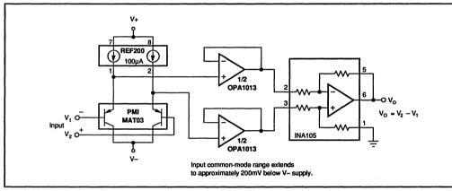
FIGURE 3. Instrumentation Amplifier.
