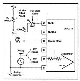
FIGURE 2. Unipolar Configuration.
