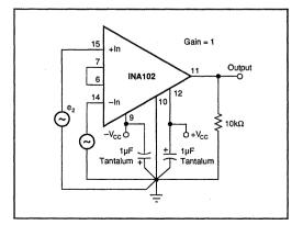
FIGURE 2. Basic Circuit Connection for the INA102.
