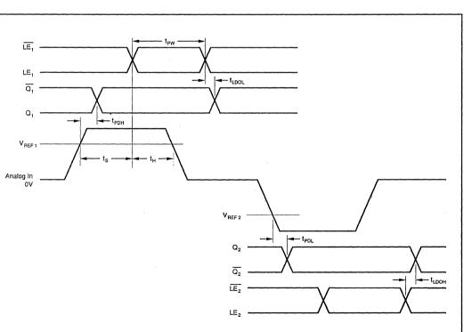
FIGURE 1. Analog and Logic Timing Definitions.
