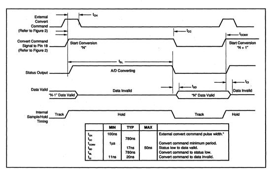
FIGURE 3. ADS602 Logic Timing Diagram.
