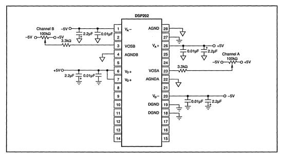
FIGURE 15. DSP202 Power Supply Connections and Optional Offset Voltage Adjustment.
