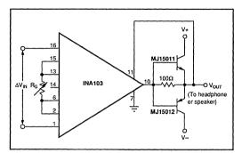
FIGURE 12. Current Boosting the Output.
