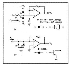
FIGURE 7. Input Protection Circuits.
