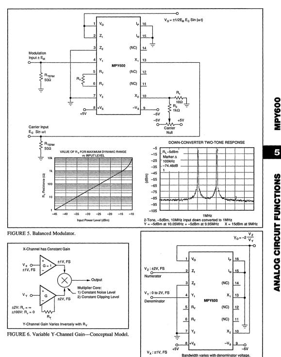
FIGURE 7. Divider Circuit.
