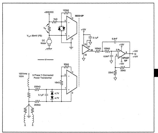
FIGURE 12. Isolated Current Monitoring Applications.
