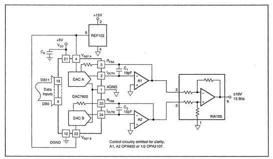
FIGURE 7. 13-Bit Bipolar DAC.
