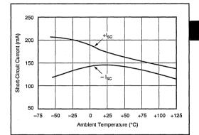
FIGURE 5. Short-Circuit Current vs Temperature.
