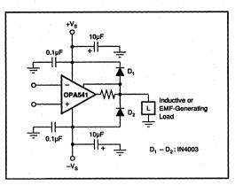
FIGURE 2. Clamping Output for EMF-Generating Loads.
