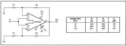
FIGURE 23. Programmable-Gain Amplifier.
