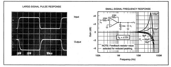
FIGURE 2. Dynamic Response- Inverting Unity-Gain.
