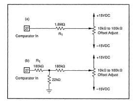
FIGURE 10. Two Methods of Connecting Optional Offset Adjust.
