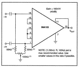
FIGURE 5. Input Offset Adjustment for AC-Coupled Inputs.
