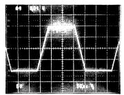
LARGE SIGNAL TRANSIENT RESPONSE V<sub>S</sub> = 5V/0V, G = +1, R<sub>L</sub> = 4.7kV to 5V
