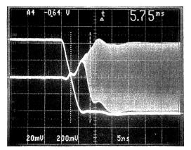
FIGURE 6. OPA676 Input Selection Time. Input B to A.
