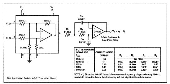
FIGURE 9. Output Filter for Noise Reduction.
