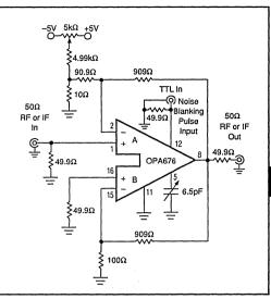
FIGURE 20. Receiver Noise Blanker: A Wideband Gated Video Amplifier.
