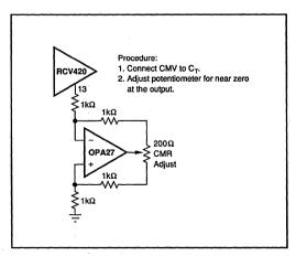
FIGURE 5. Optional Circuit for Externally Trimming CMR.
