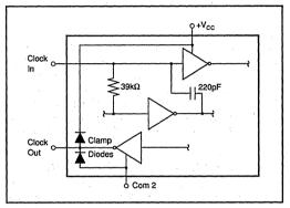
FIGURE 5. Equivalent Circuit, Clock Input/Output. Inverters are CMOS.
