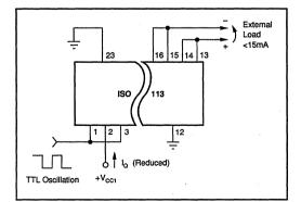
FIGURE 5. Reduced Power Dissipation.
