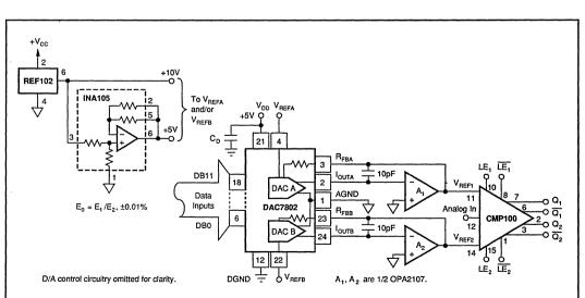
FIGURE 5. Dual DAC7802 (12-bit port), DAC7801 (8-bit port) or DAC7800 (serial port) D/A Converters Supply Reference Inputs to the CMP100. For higher resolution use DAC725, dual 16-bit D/A converter.
