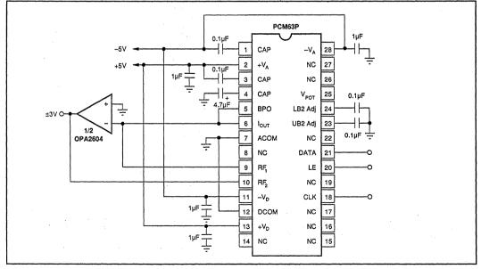
FIGURE 4. Connection Diagram.
