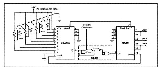
FIGURE 8. External Short Cycle Circuit.
