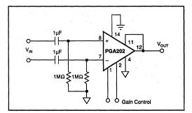
FIGURE 8. AC-Coupled Differential Amplifier for Frequencies above 0.16Hz.
