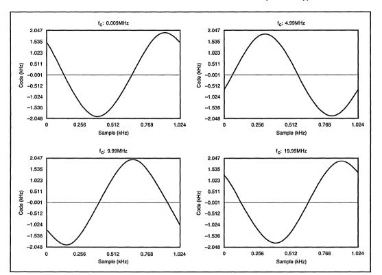
FIGURE 15. Digitized Sine Waves ( $f_s = 10MHz$ ).
