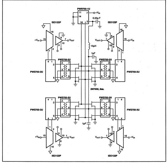
FIGURE 4. Four-Channels of ±10V Signal Isolation with Channel-to-Channel Isolation.
