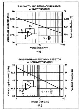
FIGURE 4. Feedback Resistor Selection Curves.
