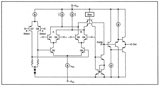
FIGURE 1. OPA675 Simplified Circuit Diagram.
