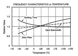
At  $V_{cc} = \pm 5$ VDC,  $R_{L} = 100\Omega$ , and  $T_{A} = +25^{\circ}$ C unless otherwise noted.
