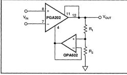
FIGURE 3. Gain Increase with Buffered Attenuator.
