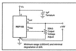
FIGURE 3. REF102 Optional Output Voltage Adjust.
