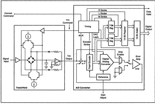
FIGURE 1. ADC604 Block Diagram—A Two-Step Subranging Architecture.
