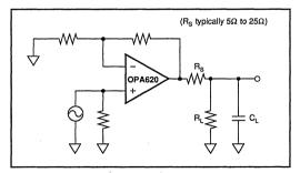
FIGURE 6. Driving Capacitive Loads.
