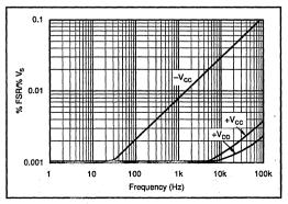
FIGURE 4. Power Supply Rejection Ripple vs Frequency.
