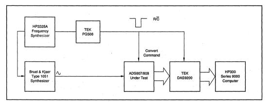
FIGURE 2. Equipment Configuration for Single-Tone Spectral Characterization.
