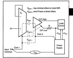
FIGURE 3. Technique for Connecting Com 1 and Com 2.
