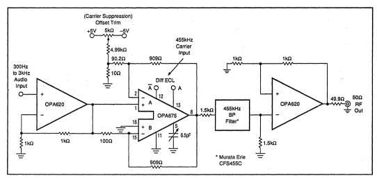
FIGURE 22. Single Sideband Supressed Carrier Generator.
