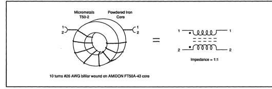
FIGURE 8. Balun Transformer Windings.
