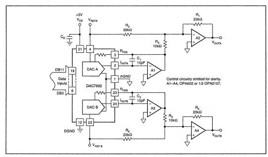
FIGURE 4. Bipolar Configuration.
