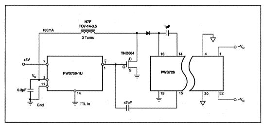
FIGURE 6. A PWS750 Driver Can Be Used to Boost the Input Voltage to 15V to Power a PWS726 From a 5V Supply.
