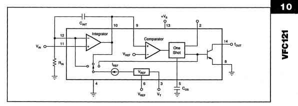
FIGURE 1. VFC121 Architecture.
