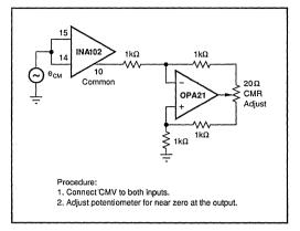
FIGURE 4. Optional Circuit for Externally Trimming CMR.
