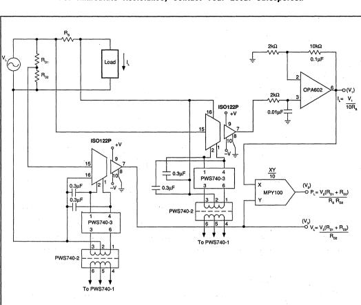
FIGURE 8. Isolated Power Line Monitor.
