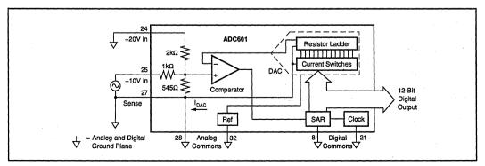
FIGURE 3. Analog and Digital Grounds, and Analog Input Sense.
