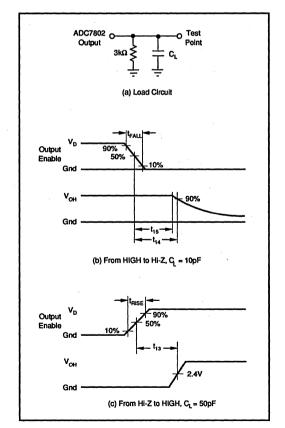
FIGURE 8. Measuring Active HIGH to/from Hi-Z State.
