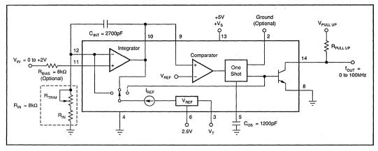
FIGURE 3. 2V Full Scale Input, 100kHz Full Scale Output.
