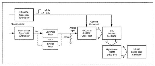
FIGURE 6. FFT Test Configuration for Single-Tone Testing.
