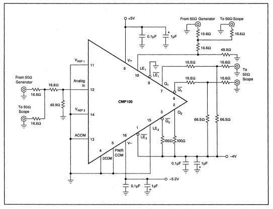
FIGURE 3. Circuit for Evaluating Logic Timing.
