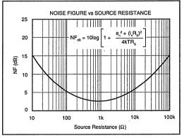
FIGURE 10. Noise Figure vs Source Resistance.
