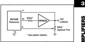
FIGURE 18. 10V with Output to Source/Sink 100mA.
