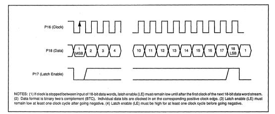
FIGURE 2. PCM61P Timing Diagram.
