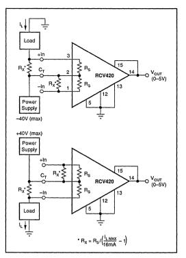
FIGURE 15. Power Supply Current Monitor Circuit.
