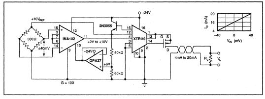
FIGURE 12. 4mA to 20mA Bridge Transmitter Using Single Supply Instrumentation Amplifier.
