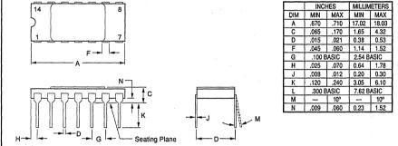
NOTE: Leads in true position within 0.01" (0.25mm) R at MMC at seating plane. Pin numbers shown for reference only. Numbers may not be marked on package.
