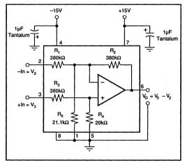
FIGURE 1. Basic Power and Signal Connections.
