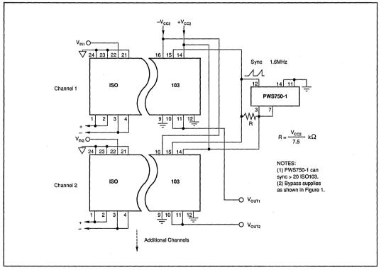
FIGURE 7. Synchronized-Multichannel Isolation.
