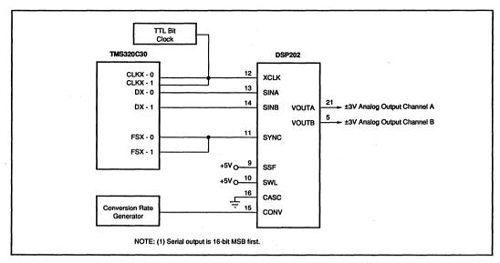
FIGURE 4. Using DSP202 with TMS320C30's Dual SIO.
