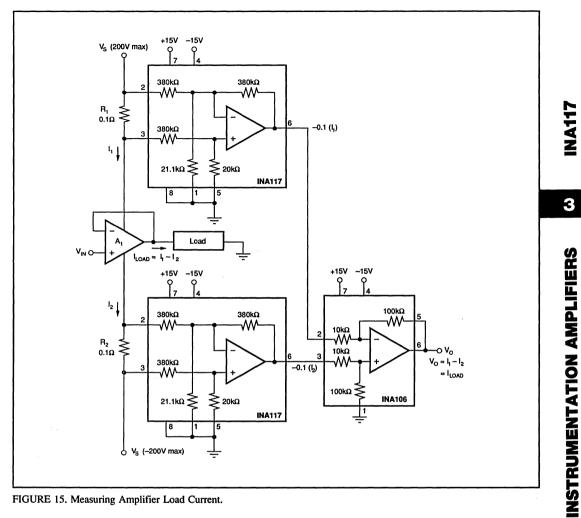
FIGURE 15. Measuring Amplifier Load Current.
