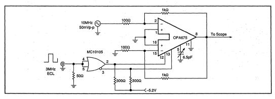
FIGURE 10. OPA675 Input Selection Transition Time Test Circuit.
