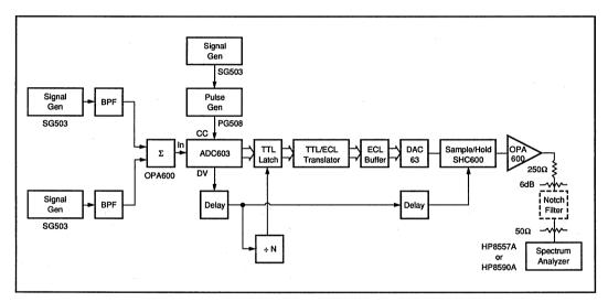
FIGURE 17. Analog-to-Analog Spectral Analysis by Beat-Frequency Techniques.
