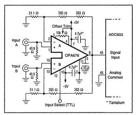
FIGURE 21. Multiplexed Input +16V/V Gain (24dB) Buffer Amplifier.
