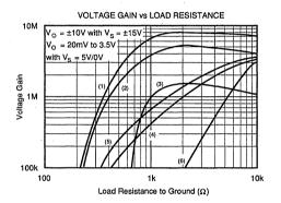
NOTES: (1)  $T_A = -55^{\circ}$ C,  $V_S = \pm 15$ V. (2)  $T_A = +25^{\circ}$ C,  $V_S = \pm 15$ V. (3)  $T_A = 125^{\circ}$ C,  $V_S = \pm 15$ V. (4)  $T_A = +25^{\circ}$ C,  $V_S = 5$ V/0V. (5)  $T_A = -55^{\circ}$ C,  $V_S = 5$ V/0V. (6)  $T_A = 125^{\circ}$ C,  $V_S = 5$ V/0V.
