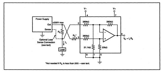
FIGURE 5. Measuring Power Supply Output Current.
