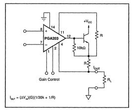
FIGURE 10. Programmable Current Source.
