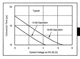
FIGURE 13. Conversion Time vs Clock Rate Control Voltage.
