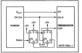
FIGURE 18. PCM78 Interface to TMS320C25/C30 DSP Processors.
