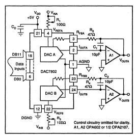
FIGURE 3. Unipolar Configuration with Gain Trim.
