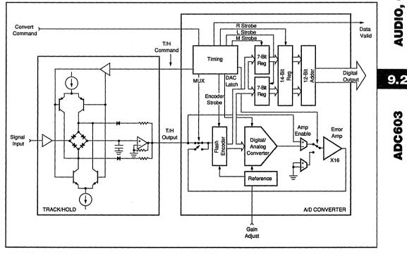
FIGURE 1. ADC603 Block Diagram—A Two-Step Subranging Architecture.
