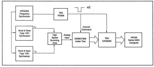
FIGURE 3. Equipment Configuration for Two-Tone Spectral Characterization.
