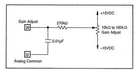
FIGURE 11. Connecting Optional Gain Adjust.
