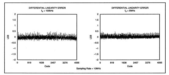
FIGURE 16. 100kHz and 5MHz Differential Linearity.
