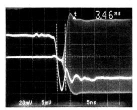
FIGURE 9. OPA675 Input Selection Time. Input B to A.
