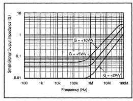
FIGURE 3. Small-Signal Output Impedance vs Frequency.
