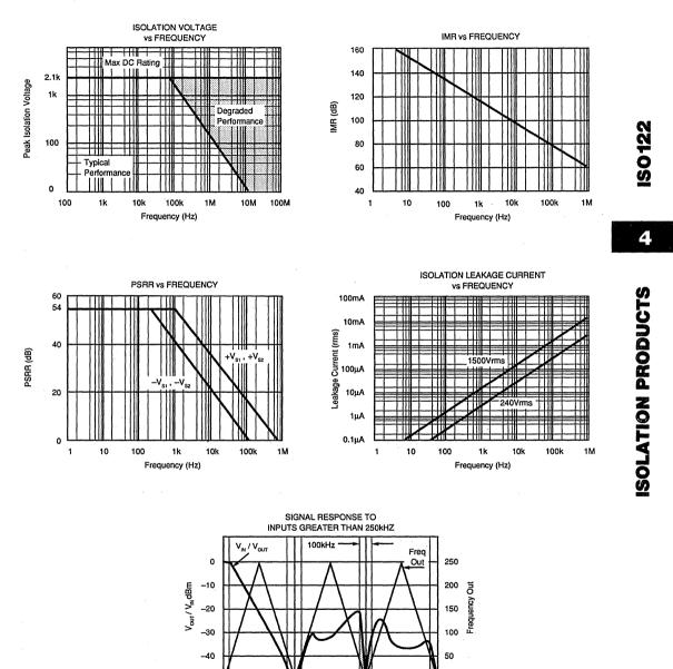
Input Frequency (NOTE: Shaded area shows aliasing frequencies that cannot be removed by a low-pass filter at the output.)
