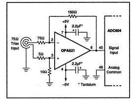
FIGURE 9. Differential Input Buffer Amplifier (Gain = -2V/V).
