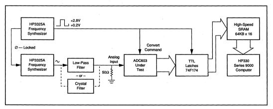
FIGURE 2. Block Diagram of FFT Test for THD, SNR, and SINAD.
