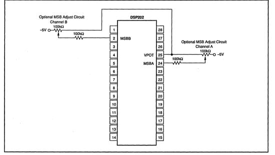
FIGURE 16. DSP202 Optional MSB Adjust Circuit.
