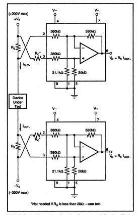
FIGURE 4. Measuring Supply Currents of Device Under Test.
