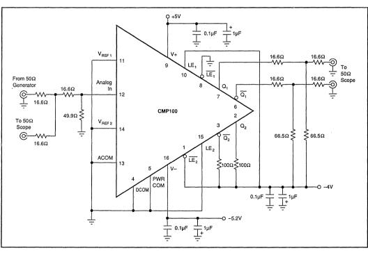
FIGURE 2. Circuit for Evaluating Analog Propagation Delay,  $t_{PDH}$ ,  $t_{PDL}$ .
