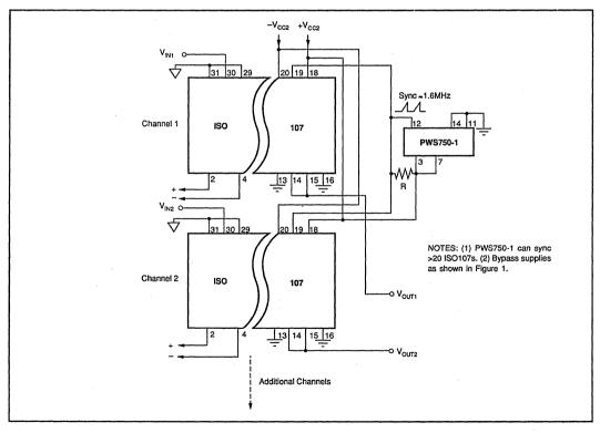
FIGURE 6. Synchronized-Multichannel Isolation.
