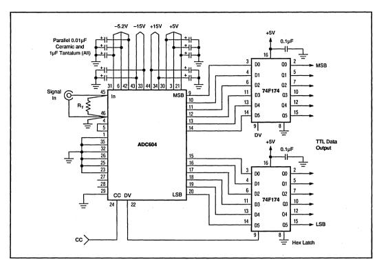
FIGURE 11. Interface Circuit—Digital Output Strobed by Data Valid Pulse. Supply connection shown: power supplies and grounds shared by analog and digital pins, using common ground plane.
