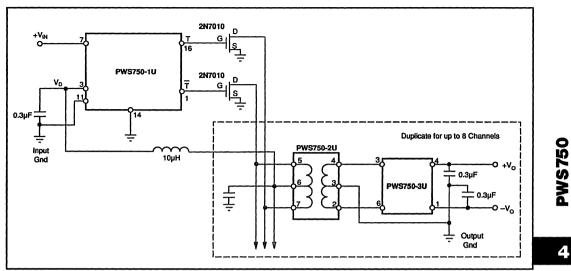
FIGURE 9. FET Pair Driving Up to Eight-Channels.
