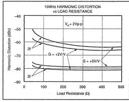
FIGURE 8. 10MHz Harmonic Distortion vs Load Resistance.
