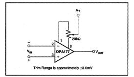
FIGURE 1. Optional Offset Nulling Circuit.
