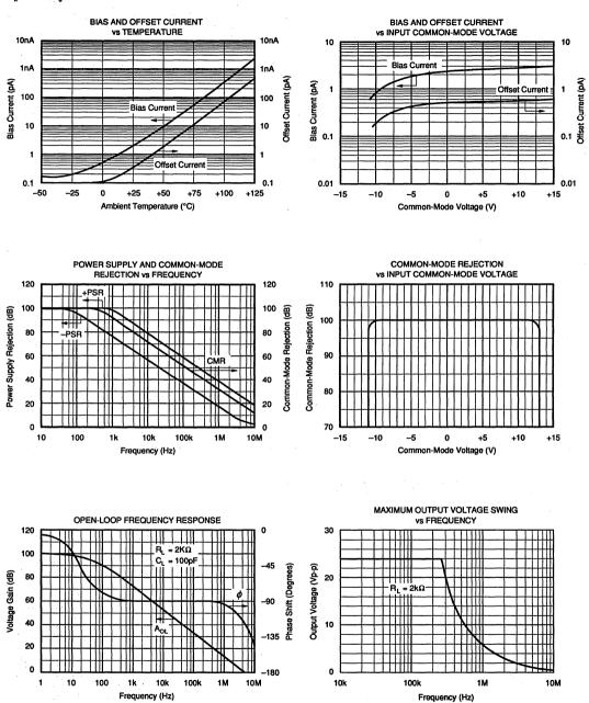
$T_{A} = +25^{\circ}C$ ,  $V_{B} = \pm 15V$  unless otherwise noted.
