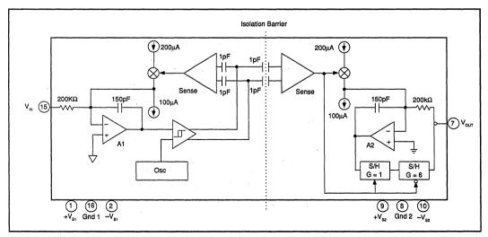
FIGURE 1. Block Diagram.
