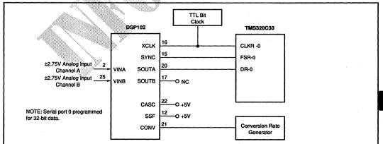
FIGURE 4. Using DSP102 with TMS320C30 in Cascade Mode.
