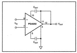
FIGURE 5. Output Filtering.
