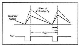
FIGURE 1. Basic Charge-Balance Waveforms.
