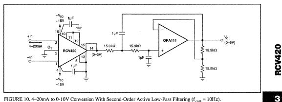
FIGURE 10. 4–20mA to 0-10V Conversion With Second-Order Active Low-Pass Filtering ( $f_{-1/R} = 10$ Hz).
