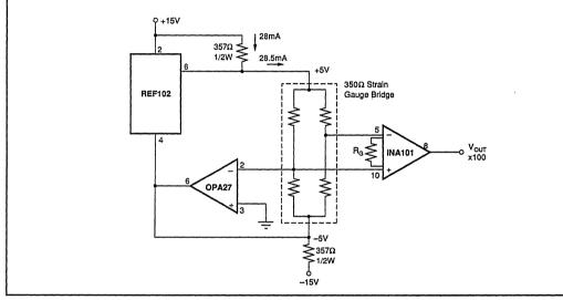
FIGURE 8. Strain Gauge Conditioner for  $350\Omega$  Bridge.
