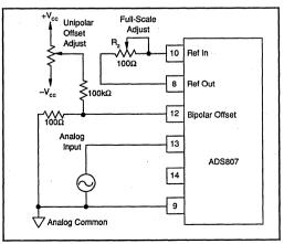
FIGURE 4. Unipolar Connection.
