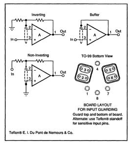
FIGURE 1. Connection of Input Guard.
