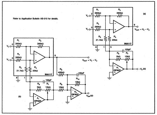
FIGURE 12. Common-Mode Voltage Monitoring.
