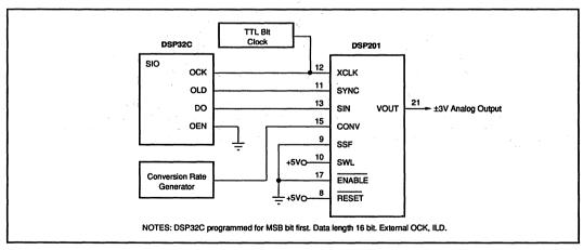
FIGURE 10. Using DSP201 with DSP32C with 16-Bit Data Words.
