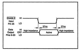
FIGURE 16. Digital Data Tri-State Output.
