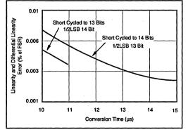
FIGURE 6. Linearity Versus Conversion Time.
