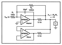
FIGURE 5. Paralleled Operation, Extended SOA.
