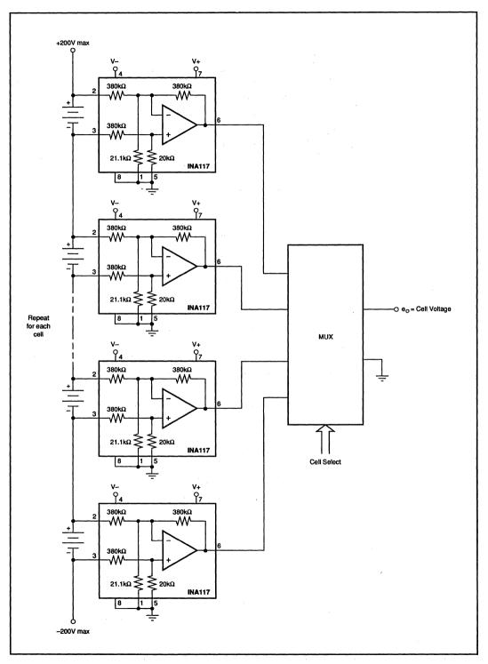
FIGURE 14. Battery Cell Voltage Monitor.
