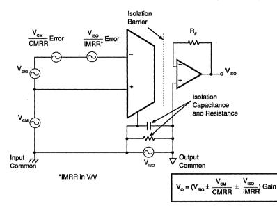
Figure 2. Typical Isolation Amplifier, Voltage (Input) Mode.
