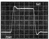
$\begin{array}{l} \text{SMALL SIGNAL RESPONSE} \\ \text{R}_{\text{L}} = \infty, \text{C}_{\text{L}} = 1000 \text{pF} \end{array}$
