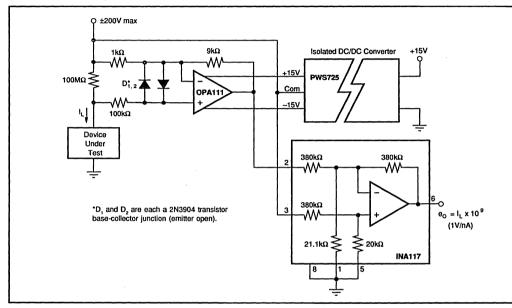
FIGURE 8. Leakage Current Measurement Circuit.
