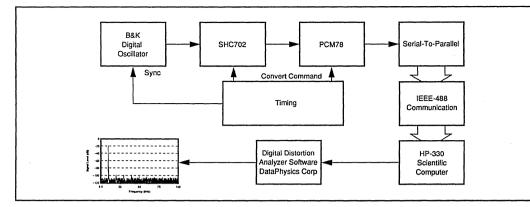
FIGURE 2. Block Diagram of Distortion Test Circuit.
