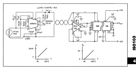
FIGURE 6. Isolated 4-20mA Instrument Loop.
