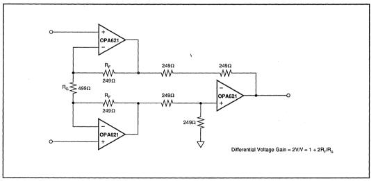
FIGURE 15. Wideband, Fast-Settling Instrumentation Amplifier.
