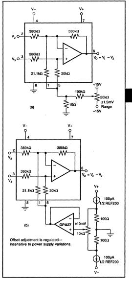
FIGURE 2. Offset Voltage Trim Circuits.
