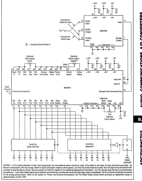
FIGURE 3. ADC701/SHC702 Connection Diagram.
