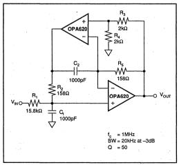
FIGURE 12. High-Q 1MHz Bandpass Filter.
