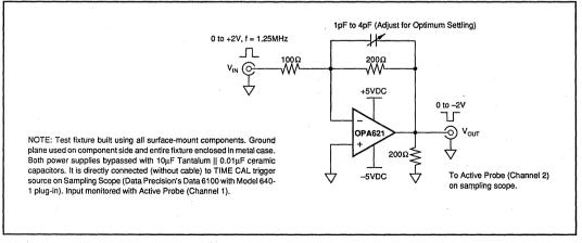
FIGURE 7. Settling Time Test Circuit.
