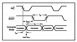
FIGURE 3. Acquisition and Conversion Timing.
