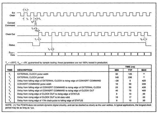
FIGURE 7. Conversion Timing when using External Clock.
