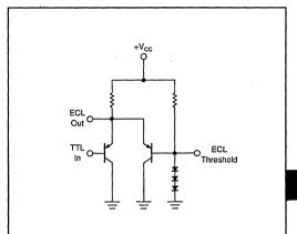
FIGURE 2. Internal OPA676 TTL Logic Level Shifter.
