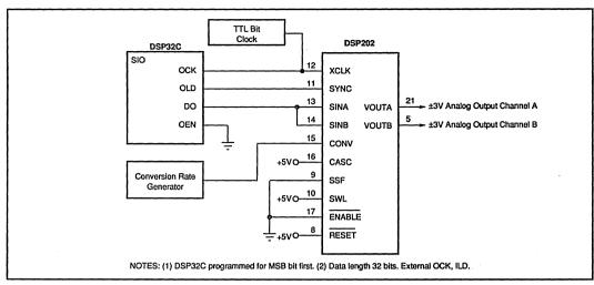
FIGURE 11. Using DSP202 with DSP32C in Cascade Mode.
