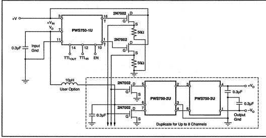
FIGURE 3. MOSFET Driver Booster Circuits.
