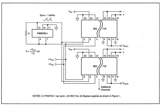
FIGURE 7. Synchronized-Multichannel Isolation.
