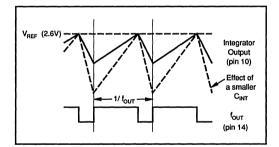
FIGURE 2. Timing Diagram.
