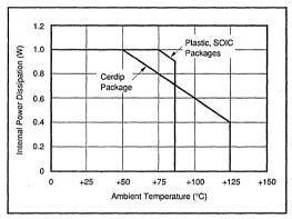
FIGURE 4. Maximum Power Dissipation.
