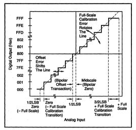
FIGURE 1. ADC774 Transfer Characteristics Terminology.
