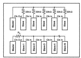
FIGURE 7. Isolating the Clk Out Node.
