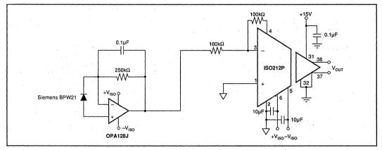
FIGURE 10. Photodiode Isolation Amplifier.
