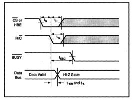
FIGURE 8. Conversion Start Timing.
