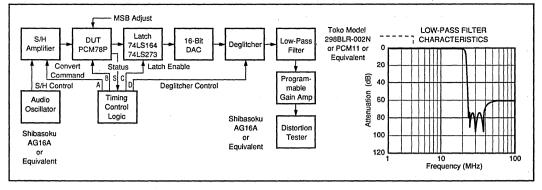
FIGURE 4. Production Distortion + Noise Test System Block Diagram.
