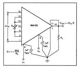
FIGURE 1. Basic Circuit Configuration.
