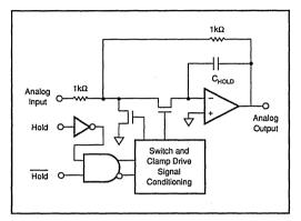
FIGURE 1. Simplified Block Diagram of the SHC702.
