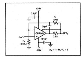
FIGURE 3. Isolating Capacitive Loads.
