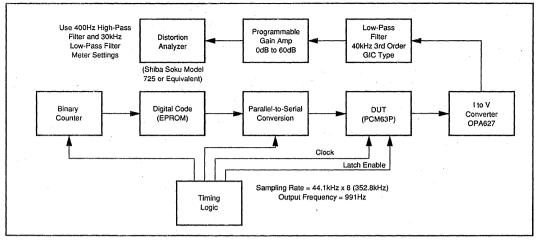
FIGURE 1. Production THD + N Test Setup.
