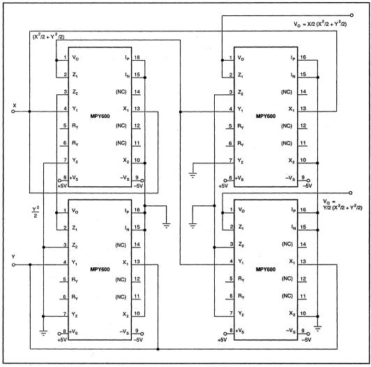
FIGURE 15. CRT Geometry Correction.
