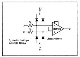
FIGURE 6. Input Protection Circuit.
