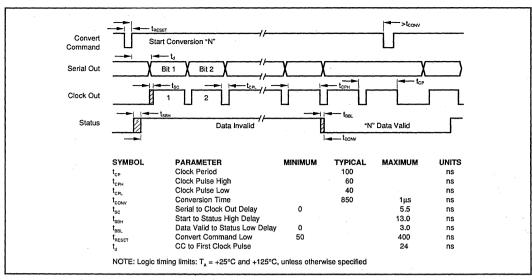
FIGURE 9. ADC601 Logic Timing Diagram.
