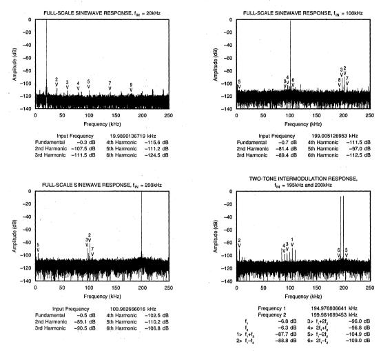
NOTE: For figures above, sampling rate = 500.000000000kHz. 16,384 point FFT, non-windowed. Noise floor limited by synthesized generators.
