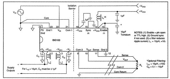
FIGURE 1. Signal and Power Connections.
