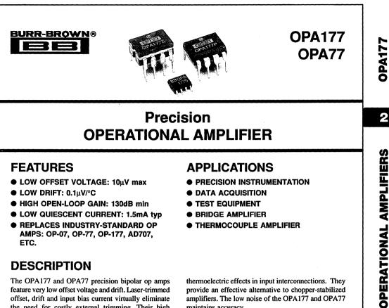
offset, drift and input bias current virtually eliminate the need for costly external trimming. Their high performance and low cost make them ideally suited to a wide range of precision instrumentation.
