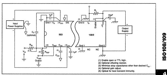
FIGURE 2. ISO108/109 Connection Diagram.
