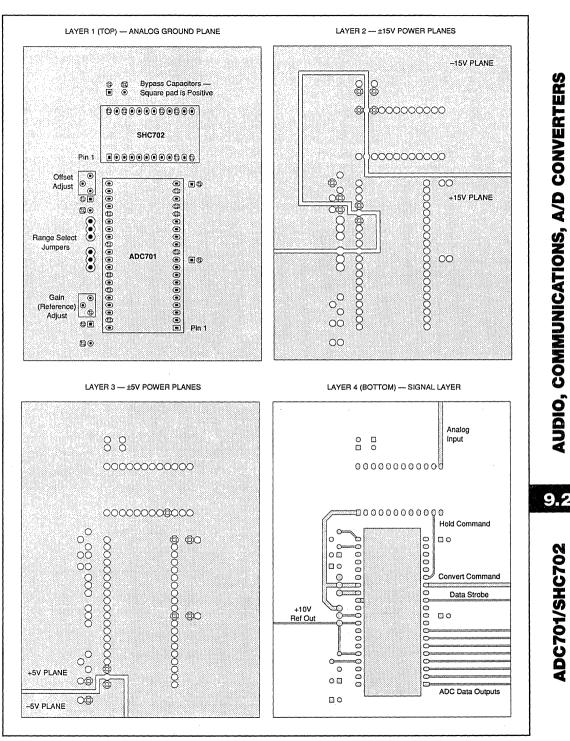
FIGURE 4. Example of Four-Layer PC Board Layout.
