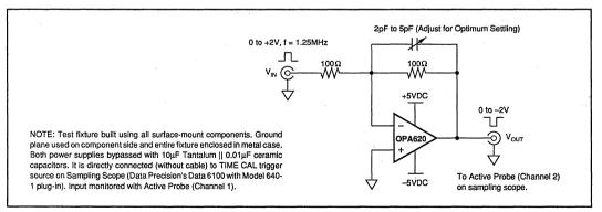
FIGURE 7. Settling Time Test Circuit.
