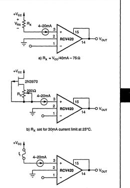
c) f, is 0.032A, Lifflefuse Series 217 fast-acting fuse.
