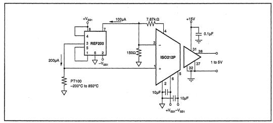
FIGURE 13. Isolated temperature Sensing and Amplification.
