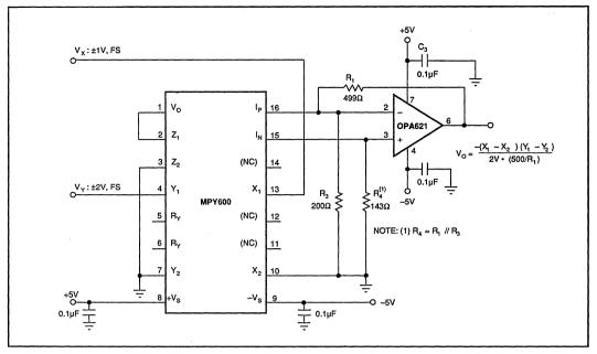
FIGURE 4. 75MHz DC-Coupled Multiplier.
