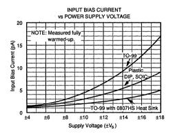
$T_{_{A}}$  = +25°C,  $V_{_{S}}$  = ±15V unless otherwise noted.
