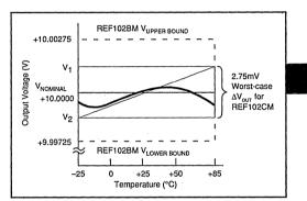
FIGURE 1. REF102CM Output Voltage Drift.
