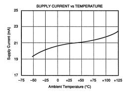
At V<sub>cc</sub> = ±5VDC, R<sub>L</sub> = 100 $\Omega$ , and T<sub>A</sub> = +25°C unless otherwise noted.
