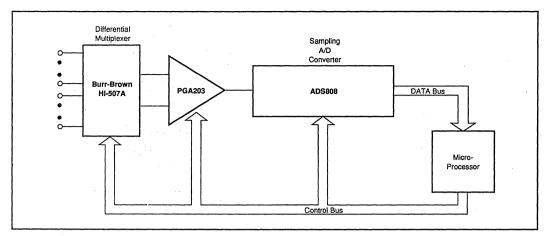
FIGURE 14. 8-Channel Differential Data Acquisition System.
