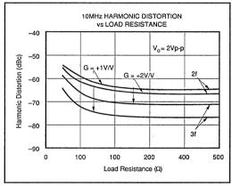
FIGURE 8. 10MHz Harmonic Distortion vs Load Resistance.
