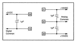
FIGURE 7. Recommended Power Supply Decoupling.
