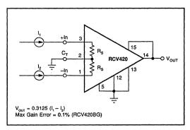
FIGURE 13. Differential Current-to-Voltage Converter.
