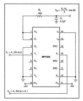
FIGURE 10. Phase Detector.
