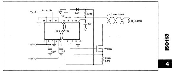
FIGURE 6. Isolated Current Loop Driver.
