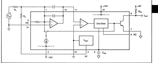
FIGURE 3. Offsetting the Frequency Output.
