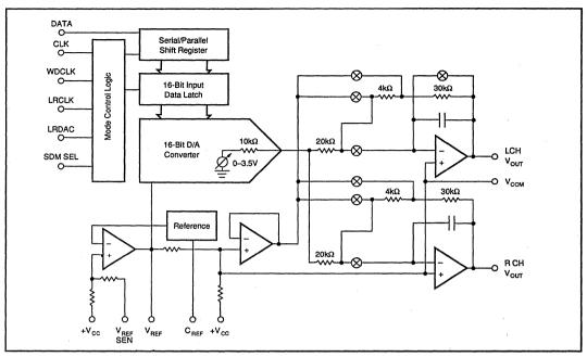
FIGURE 2. PCM60P/66P Block Diagram.
