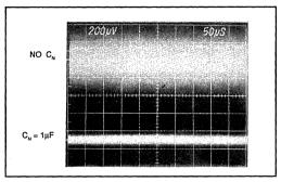
FIGURE 5. Effect of 1µF Noise Reduction Capacitor on Broadband Noise ( $f_{-3dB} = 1$ MHz).
