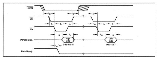
ADC700 Parallel Output Timing.
