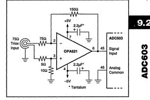
FIGURE 10. Differential Input Buffer Amplifier (Gain = -2V/V).
