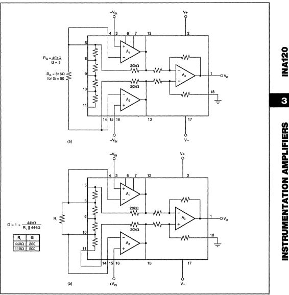
FIGURE 3. External Gain-Setting Resistors.
