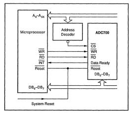
FIGURE 9. Parallel Data Bus Interface.
