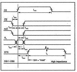
FIGURE 8. Conversion Cycle Timing.
