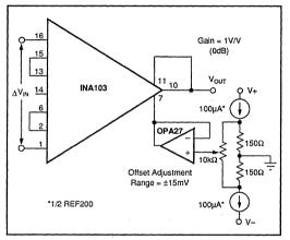
FIGURE 4. Output Offsetting.
