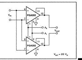
FIGURE 11. Programable Differential In/Differential Out Amplifier.
