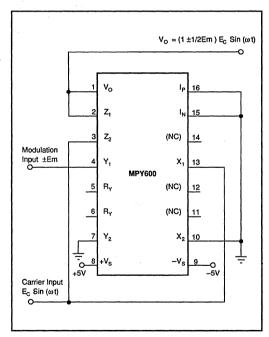
FIGURE 11. Linear AM Modulator.
