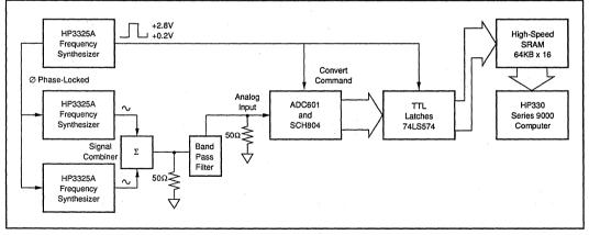
FIGURE 15. Block Diagram of FFT Test for Two-Tone IMD.
