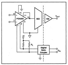
FIGURE 6. Isolated Programmable Gain Instrumentation Amplifier.
