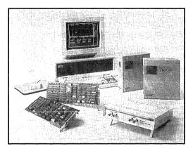
the DSP-SYS603 can be used to analyze the performance of the ADC603 in specific applications. As a test instrument, it can be used to establish and measure specification profiles for certifying device system performance. As a development system, the DSP-SYS603 can receive direct analog signals and use them as inputs for the DSP processor.
