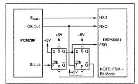
FIGURE 19. PCM78 Interface to Motorola DSP56001 DSP Processor.
