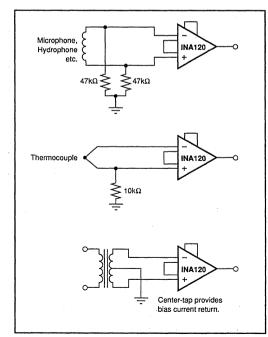
FIGURE 5. Providing an Input Bias Current Path.
