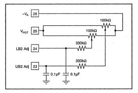
FIGURE 5. Optional Bit-2 Adjustment Circuitry.
