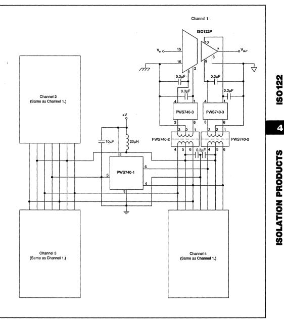
FIGURE 9. Three-Port, Low-Cost, Four-Channel Isolated, Data Acquisition System.
