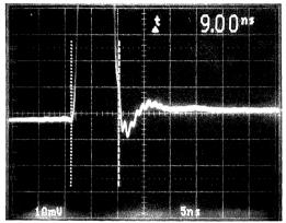
FIGURE 3. 1% Settling Time.
