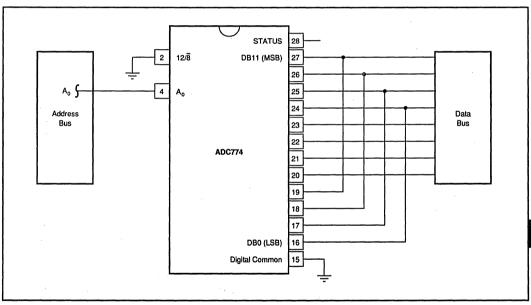
FIGURE 9. Connection to an 8-Bit Bus.
