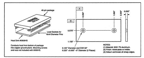
FIGURE 18. Heat Sink Transfers Heat from the DIP Package into a Copper Ground Plane.
