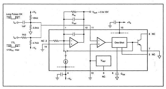
FIGURE 4. Frequency-to-Voltage Conversion.
