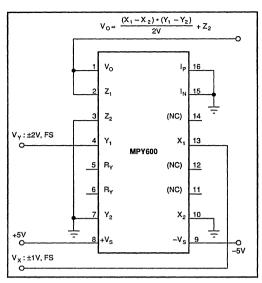
FIGURE 1. Basic Multiplier Connection.
