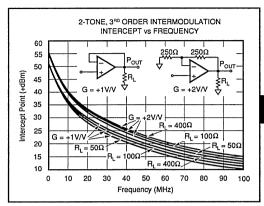
FIGURE 9. 2-Tone, 3rd Order Intermodulation Intercept vs Frequency.
