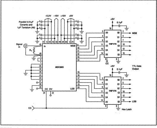
FIGURE 11. Interface Circuit—Digital Output Strobed by Convert Command. Supply connection shown: power supplies and grounds shared by analog and digital pins using common ground plane (recommended circuit).
