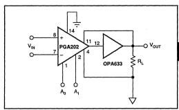
FIGURE 4. Current Boosting the Output.
