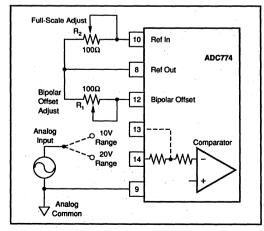
FIGURE 3. Bipolar Configuration.
