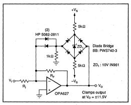
FIGURE 5. Clamp Circuit for Improved Overload Recovery.
