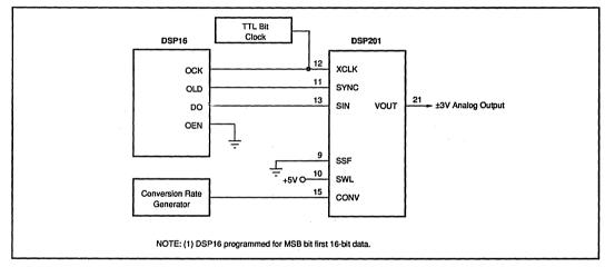
FIGURE 12. Using DSP201 with DSP16.
