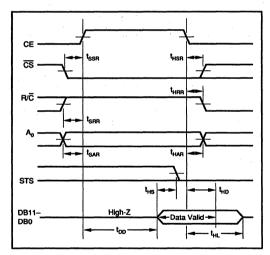
FIGURE 7. Read Cycle Timing.
