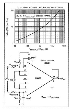
FIGURE 13. Input Decoupling and Protection.
