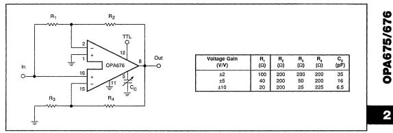
FIGURE 25. Synchronous Modulator/Demodulator (with gain).
