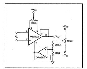
FIGURE 2. Offset Adjustment Circuits.
