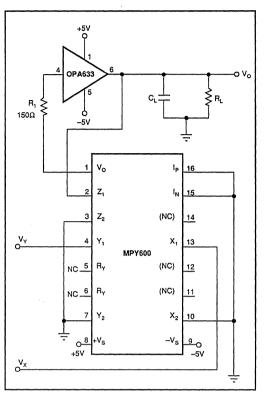
FIGURE 12. 25MHz Multiplier with Improved Load Driving Capability.
