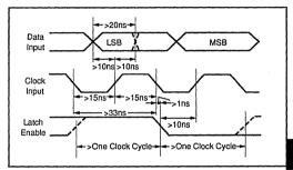
FIGURE 3. Setup and Hold Timing Diagram.
