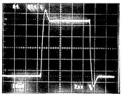
SMALL SIGNAL TRANSIENT RESPONSE V\_{S} = 5V/0V, G = +1, R\_L = 600 \Omega to Ground
