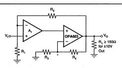
This composite amplifier uses the OPA603 current-feedback op amp to provide extended bandwidth and slew rate at high closed-loop gain. The feedback loop is closed around the composite amp, preserving the precision input characteristics of the OPA627/637. Use separate power supply bypass capacitors for each op amp.
