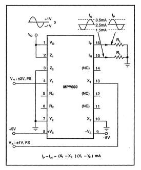
FIGURE 3. Current Output Connection.
