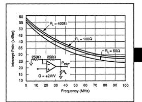
FIGURE 9. 2-Tone, 3rd Order Intermodulation Intercept vs Frequency.
