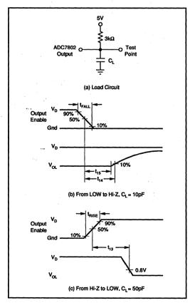
FIGURE 7. Measuring Active LOW to/from Hi-Z State.
