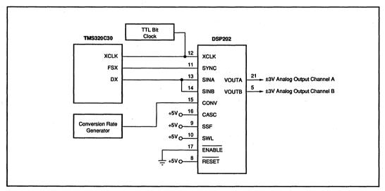
FIGURE 5. Using DSP202 with TMS320C30 in Cascade Mode.
