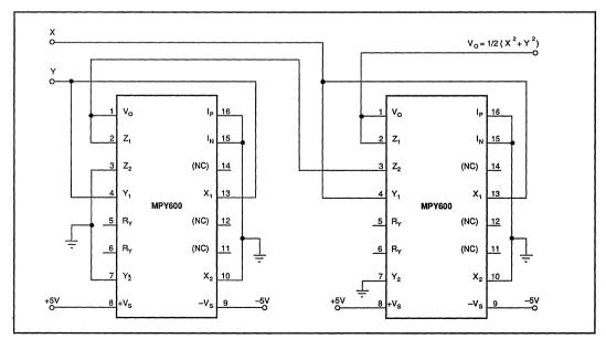
FIGURE 14. CRT Focus Correction.
