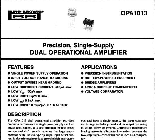
The OPA1013 is characterized for operation at both +5V (single supply) and  $\pm 15V$  power supplies. When
