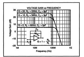
FIGURE 5. Bandwidth Results with Added Capacitor C<sub>r</sub>.
