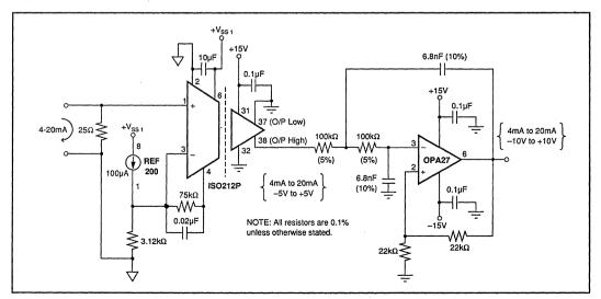
FIGURE 8. Isolated 4-20mA Current Receiver with Output Filter.
