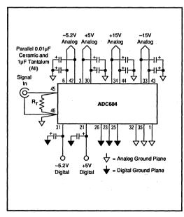
FIGURE 12. Power Supply Connections with Separate Analog and Digital Power Supplies and Ground Planes.
