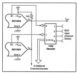
FIGURE 3. Multichannel Isolated Data Acquisition with Single Serial Output.
