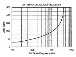
Jitter is the ratio of the  $1\sigma$  value of the distribution of the period ( $1/f_{our}$ , max) to the mean of the period.
