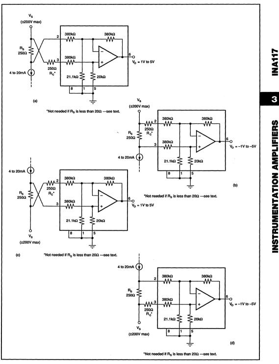
FIGURE 6. Current to Voltage Converter.
