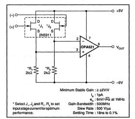
FIGURE 13. Low Noise, Wideband FET Input Op Amp.
