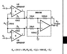
Using the INA106 for an output difference amplifier extends the input common-mode range of an instrumentation amplifier to  $\pm 10V$ . A conventional IA with a unity-gain difference amplifier has an input common-mode range limited to  $\pm 5V$  for an output swing of  $\pm 10V$ . This is because a unity-gain difference amp needs  $\pm 5V$  at the input for 10V at the output, allowing only 5V additional for common mode range.
