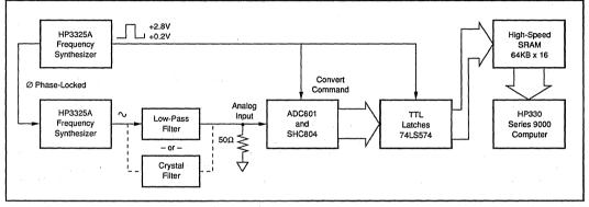
FIGURE 14. Block Diagram of FFT Test for THD, SNR, and SINAD.
