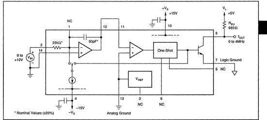
FIGURE 1. 4MHz Full-Scale Operation.
