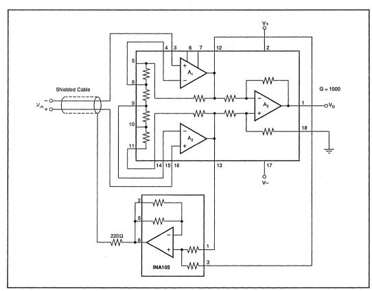
FIGURE 8. Guard Drive Circuit.
