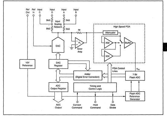
FIGURE 2. Simplified Block Diagram of the ADC701.
