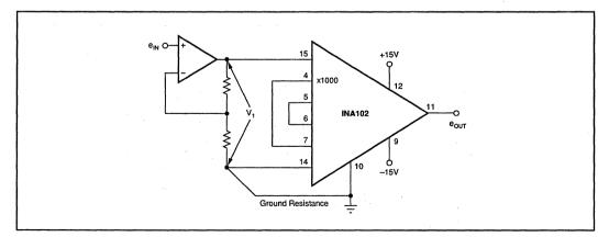
FIGURE 14. Ground Resistance Loop Eliminator (INA102 senses and amplifies V1 accurately).
