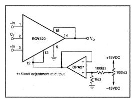
FIGURE 3. Optional Output Offset Nulling Using External Amplifier.
