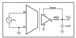
FIGURE 4. Ripple Reduction.
