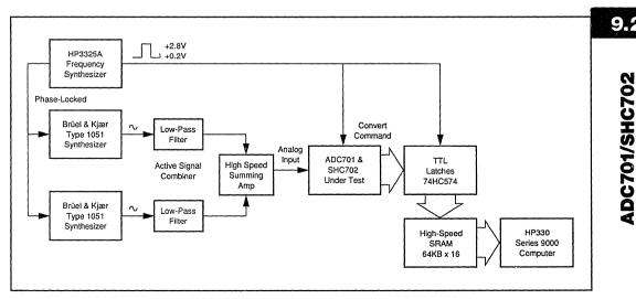
FIGURE 7. FFT Test Configuration for Two-Tone (Intermodulation) Testing.
