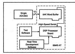
FIGURE 1. Single Channel Analog Input System.
