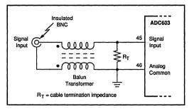
FIGURE 7. Floating-Input Balun Transformer.
