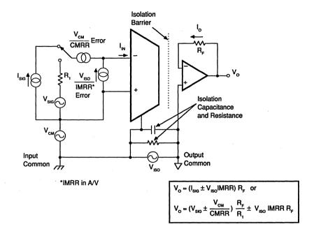
Figure 1. Typical Isolation Amplifier, Current (Input) Mode.
