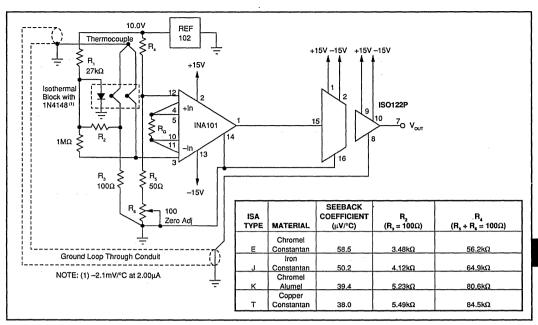
FIGURE 6. Thermocouple Amplifier with Ground Loop Elimination, Cold Junction Compensation, and Up-scale Burn-out.
