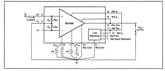
FIGURE 1. Basic Power Supply and Signal Connections.
