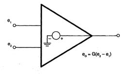
Figure 1. Idealized Model of an Instrumentation Amplifier.
