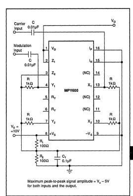
FIGURE 13. Single-Supply Balanced Modulator.
