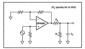
FIGURE 6. Driving Capacitive Loads.
