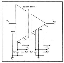
FIGURE 2. Basic Signal and Power Connections.
