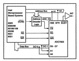
FIGURE 16. Interface to Intel Microprocessors.
