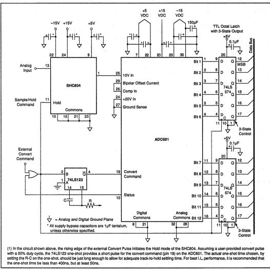
FIGURE 2. Basic Connection Diagram in Bipolar Operation and Dynamic Test Circuit.
