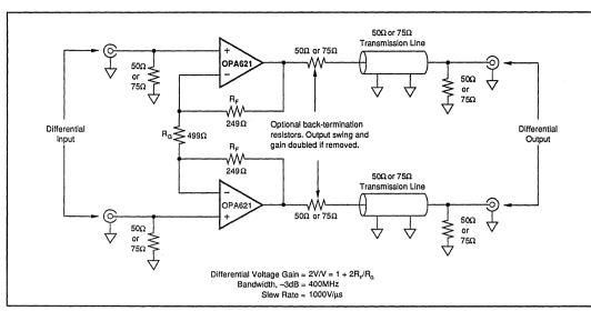
FIGURE 14. Differential Line Driver for  $50\Omega$  or  $75\Omega$  Systems.
