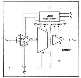
FIGURE 3. Programmable-Gain Isolation Channel with Gains of 1, 10, and 100.
