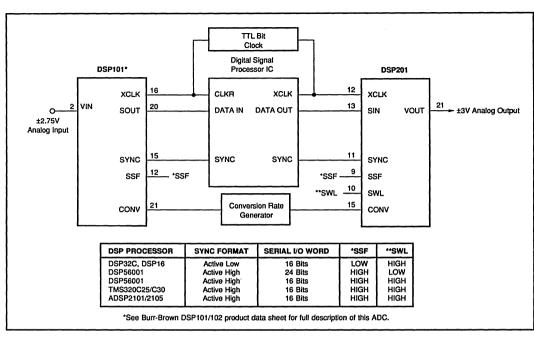
FIGURE 2. Analog Input and Analog Output System.
