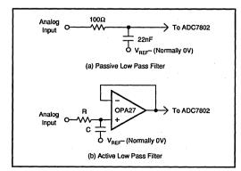
FIGURE 9. Input Signal Conditioning.
