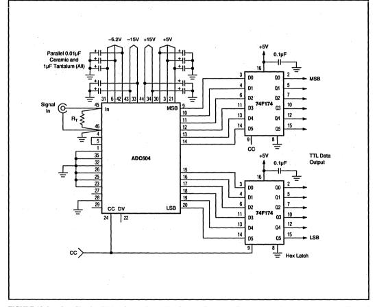
FIGURE 10. Interface Circuit—Digital Output Strobed by Convert Command. Supply connection shown: power supplies and grounds shared by analog and digital pins using common ground plane. (Recommended circuit)
