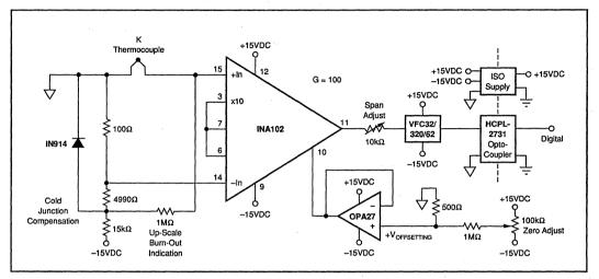
FIGURE 7. Isolated Thermocouple Amplifier with Cold Junction Compensation.
