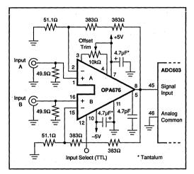
FIGURE 21. A Multiplexed-Input Buffer Amplifier (Gain = +16V/V).
