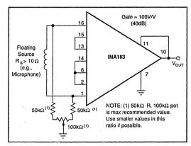
FIGURE 7. Input Offset Adjustment for Floating Source.
