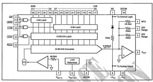
FIGURE 1. DAC813 Block Diagram.
