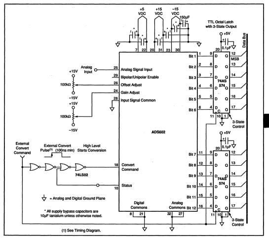
FIGURE 2. ADS602 Application Circuit.
