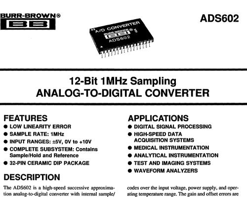
hold amplifier. This unique design utilizes a bipolar technology with on-chip thin film resistors to preserve analog accuracy and a high-speed CMOS chip to perform digital logic control. Outstanding linearity, noise, and dynamic range are achieved by this converter design. The ADS602 is thoroughly tested for dynamic performance.
