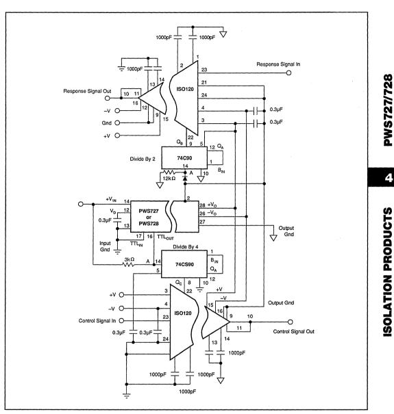
FIGURE 3. The PWS727 or PWS728 Can Be Used to Synchronize the ISO120. The Output Sync Must be Divided by 2 and the TTL<sub>OUT</sub> Must Be Divided by 4.
