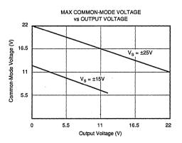
At  $T_{A} = +25^{\circ}$ C,  $V_{S} = \pm 15$ V unless otherwise noted.
