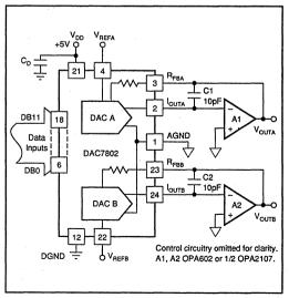
FIGURE 2. Unipolar Configuration.
