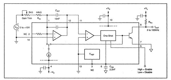
FIGURE 2. 100kHz Full-Scale Operation.
