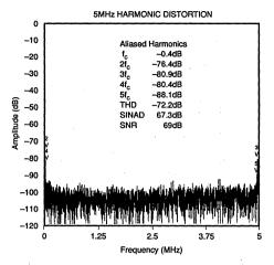
NOTE: Sample rate = 9.99 MHz; even harmonics folded to left edge and odd harmonics folded to right edge. Any nonharmonically related spurious products show clearly in the center.
