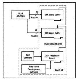
FIGURE 2. Dual Channel Analog Input System.
