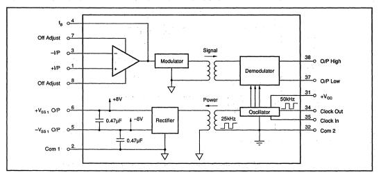
FIGURE 2. Simplified Diagram of Isolation Amplifier.
