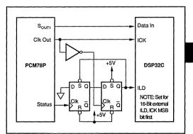
FIGURE 20. PCM78 Interface to AT&T DSP16 & DSP32C Processors.
