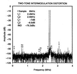
NOTE: Sample rate = 8MHz; highest IMD product is cursor number 1: f1 +f2. The second-order -76.3dBc product determines the wideband spurious-free dynamic range of this example. For RF applications third-order IMD products such as those at cursors 3 and 6 are the limiting spurs. Under these conditions spurious-free dynamic range is limited by 2f2+f1 to 84.3dBc.
