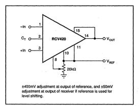
FIGURE 8. Optional Voltage Reference External Trim Circuit.
