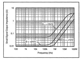
FIGURE 3. Small-Signal Output Impedance vs Frequency.
