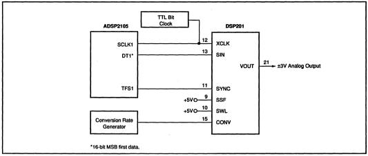
FIGURE 13. Using DSP201 with ADSP-2105.
