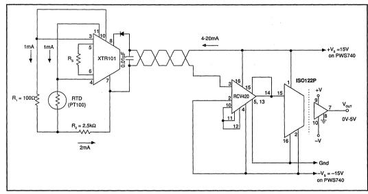
FIGURE 7. Isolated 4-20mA Instrument Loop. (RTD shown.)
