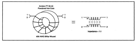
FIGURE 7. Balun Transformer Windings.
