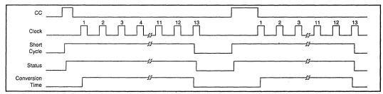
FIGURE 12. Short Cycle Operation Timing.
