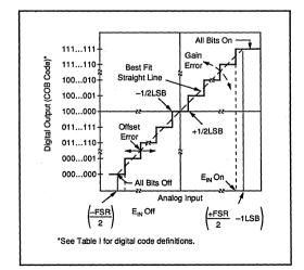
FIGURE 1. Input vs Ouput for an Ideal Bipolar A/D Converter.
