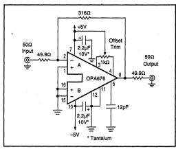
FIGURE 14. OPA676 Used As A Conventional Op-Amp: A 10dB Gain Wideband Video Amplifier with  $50\Omega$  Input/Output Impedance.
