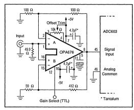
FIGURE 18. Programmable-Gain +2V/V (6dB) or +8V/V (18dB) Buffer Amplifier for Floating-Point Conversion.
