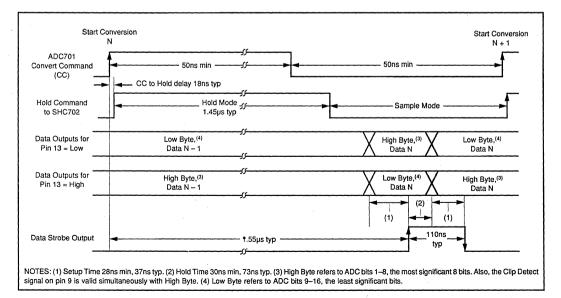
FIGURE 5. ADC701 Interface Timing Diagram.
