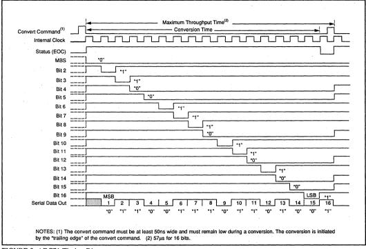
FIGURE 2. ADC71 Timing Diagram.
