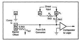
FIGURE 8. ADC76 Input Scaling Circuit.
