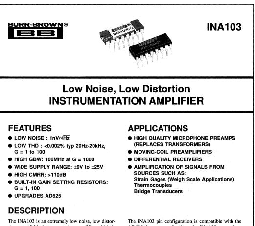
tion monolithic instrumentation amplifier which is especially suitable for amplification of low level signals in audio systems. Input circuitry provides near-theoretical limit noise performance for  $200\Omega$ source impedances. A unique distortion-cancellation network in the input stage reduces THD to extremely low levels.
