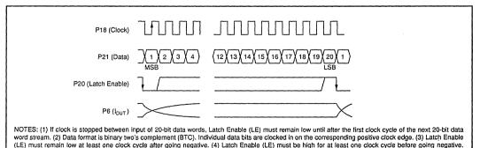
(5) Iour changes on negative going edge of Latch Enable (LE).
