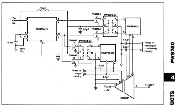
FIGURE 5. A Complete ±10V Signal Acquisition System Operating From a Single 5V Supply.
