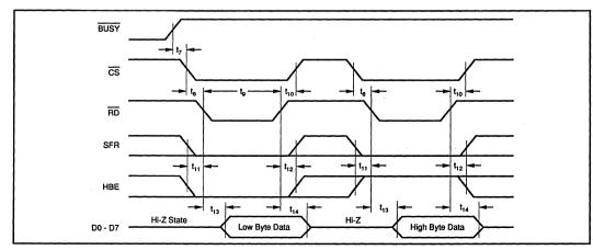
FIGURE 4. Read Cycle Timing.
