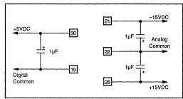
FIGURE 8. Recommended Power Supply Decoupling.
