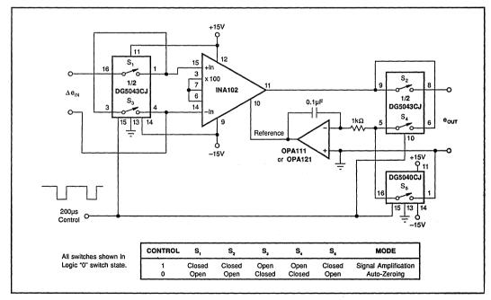
FIGURE 16. Auto-Zeroing Instrumentation Amplifier Circuit.
