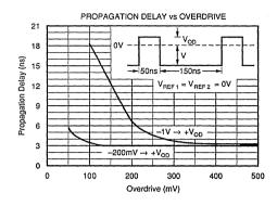
NOTE: Propagation Delay vs Overdrive is shown for two amplitudes of input pulse: from -200mV  $\rightarrow$  +V<sub>00</sub> (0.2nV/ns slew rate) and -1V  $\rightarrow$  +V<sub>00</sub> (1V/ns slew rate). For an inverse input waveform: from +1V  $\rightarrow$  -V<sub>00</sub> and from +200mV  $\rightarrow$  -V<sub>00</sub>, propagation delays identical to those above are produced.
