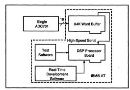
FIGURE 2. Single Channel Analog Input System with Digital Input Buffer.
