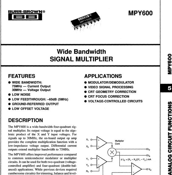
anced) applications. While previous devices required cumbersome circuitry for trimming, balance and levelshifting, the MPY600 requires no external components. A single external resistor can be used to program the conversion gain for optimum spurious-free dynamic range. When used as a modulator, carrier feedthrough measures -60dB at 5MHz.
