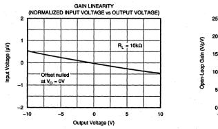
$T_{A} = +25^{\circ}C$ ,  $V_{S} = \pm 15V$  unless otherwise noted.
