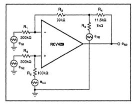
FIGURE 7. Resistor Noise Model.
