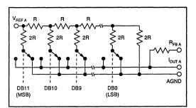
FIGURE 1. Simplified DAC Circuit.
