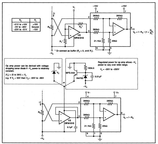
FIGURE 7. Current Sensing with Input Buffer.
