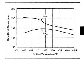
FIGURE 5. Short-Circuit Current vs Temperature.
