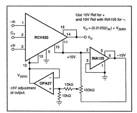
FIGURE 4. Optional Zero Adjust Circuit.
