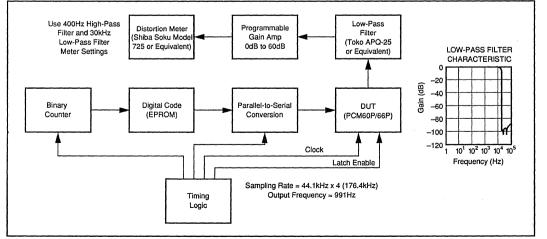
FIGURE 4. THD + N Test Setup Diagram.
