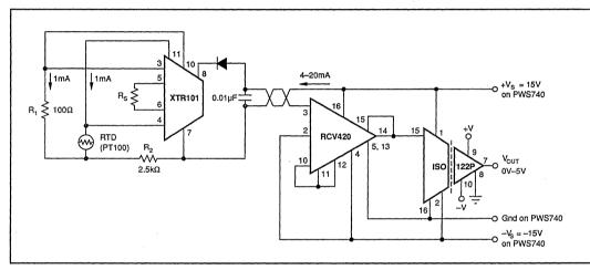
FIGURE 11. Isolated 4-20mA Instrument Loop (RTD shown).
