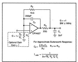
FIGURE 6. Driving Large Capacitive Loads.
