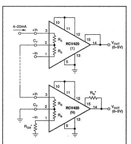
$^*R_{\text{CM}}$  and  $R_{\text{G}}$  are used to provide a first order correction of CMR and Gain Error, respectively. Table 1 gives typical resistor values for  $R_{\text{CM}}$  and  $R_{\text{G}}$  when as many as three RCV420s are stacked. Table 2 gives typical CMR and Gain Error with no correction. Further improvement in CMR and Gain Error can be achieved using a 500kΩ potentiometer for  $R_{\text{CM}}$  and a 100Ω potentiometer for  $R_{\text{C}}$ .
