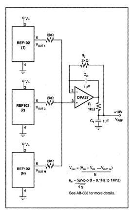
FIGURE 14. Precision Voltage Reference with Extremely Low Noise.
