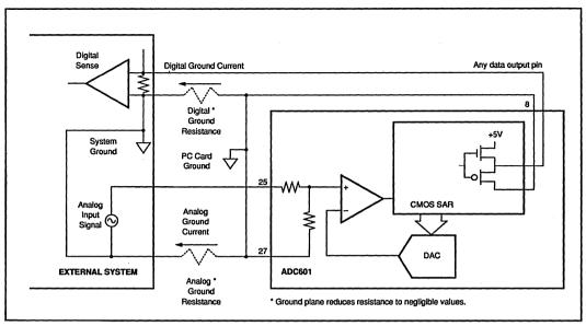
FIGURE 4. Ground Loop Interaction Between Analog and Digital Grounds when ADC Is Connected.
