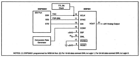
FIGURE 9. Using DSP201 with DSP56001.
