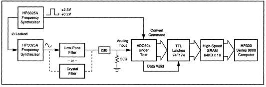
FIGURE 2. Block Diagram of FFT Test for HD, SNR, SFDR and Swept-Power Test.
