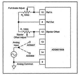
FIGURE 5. Bipolar Connection.
