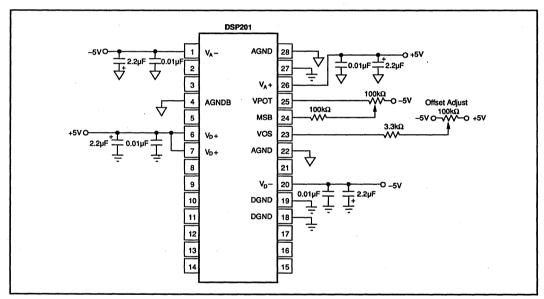
FIGURE 14. DSP201 Power Supply Connections and Adjust Circuits.
