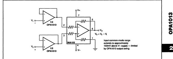
FIGURE 2. Instrumentation Amplifier.
