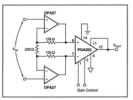
FIGURE 12. Low Noise Differential Amplifier with Gains of 100, 200, 400, 800.
