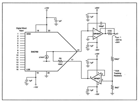
FIGURE 7. 16-Bit Programmable Voltage Source.
