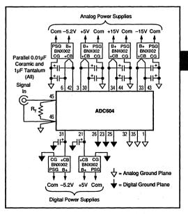
FIGURE 13. Power Supply Connections with Separate Analog and Digital Power Supplies and Ground Planes with Noise Filtering
