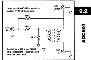
FIGURE 17. Passive Signal Combiner.
