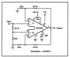
FIGURE 15. Very Fast Programmable Gain Amplifier with Voltage Gains of +1V/V and +16V/V (0dB and 24dB).
