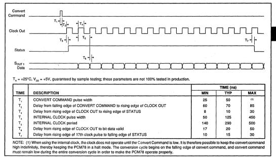
FIGURE 6. Conversion Timing when using Internal Clock.
