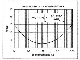
FIGURE 10. Noise Figure vs Source Resistance.
