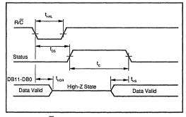
FIGURE 6. R/C Pulse Low — Output Enables After Conversion.
