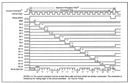
FIGURE 2. ADC76 Timing Diagram.
