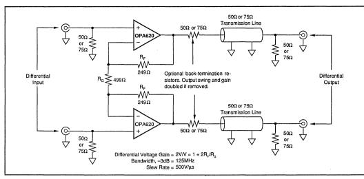
FIGURE 14. Differential Line Driver for  $50\Omega$  or  $75\Omega$  Systems.
