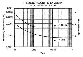
This graph describes the low frequency stability of the VFC110: the ratio of the 1 or point of the distribution of 100 runs (where each mean frequency came from 1000 readings for each gate time) to the overall mean frequency.
