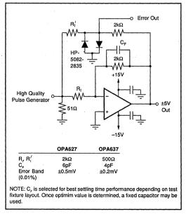
FIGURE 11. Settling Time and Slew Rate Test Circuit.
