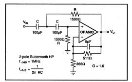
FIGURE 9. High-Pass Filter - 1MHz.
