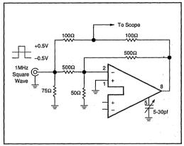
FIGURE 4. OPA675/676 Settling Time Test Circuit.
