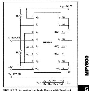
FIGURE 2. Adjusting the Scale Factor with Feedback.
