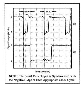
FIGURE 11. (a) Clock, (b) Serial Out.
