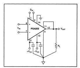
FIGURE 1. Basic Circuit Connections.
