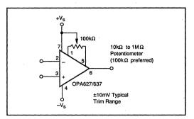
FIGURE 3. Optional Offset Voltage Trim Circuit.
