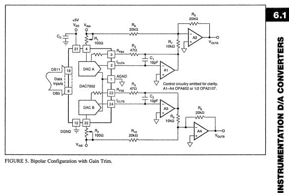
FIGURE 5. Bipolar Configuration with Gain Trim.
