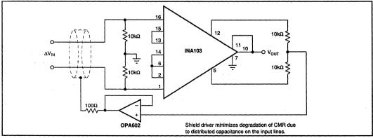
FIGURE 16. Instrumentation Amplifier with Shield Driver.
