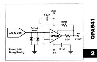
FIGURE 6. Programmable Voltage Source.
