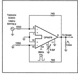
FIGURE 7. OPA676 Input Selection Transition Time Test Circuit.
