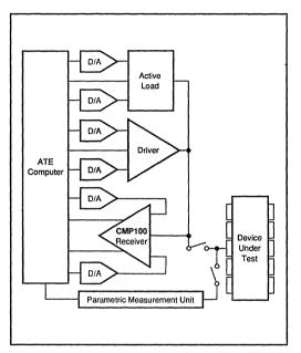
FIGURE 4. Typical ATE Pin Receiver Application.
