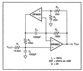
FIGURE 12. High-Q 1MHz Bandpass Filter
