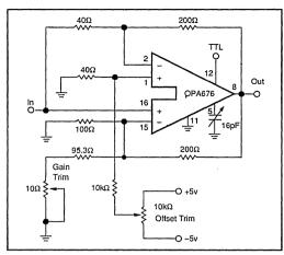
FIGURE 17. Synchronous Modulator/Demodulator with Carrier Balance Trim (Gain =  $\pm 5$ V/V).
