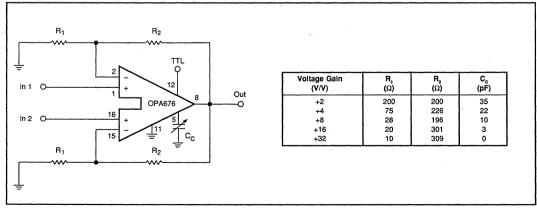
FIGURE 24. Two-Input Multiplexer (with gain).
