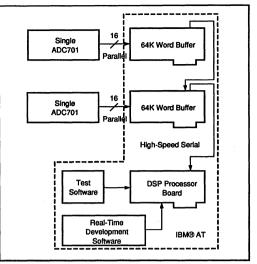
FIGURE 3. Dual Channel Analog Input System.
