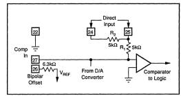
FIGURE 9. ADC71 Input Scaling Circuit.
