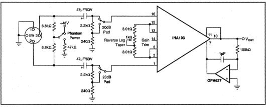
FIGURE 15. Microphone Preamplifier with Provision for Phantom Power Microphones.
