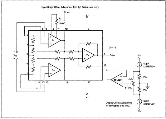
FIGURE 4. Offset Adjustment Circuits.
