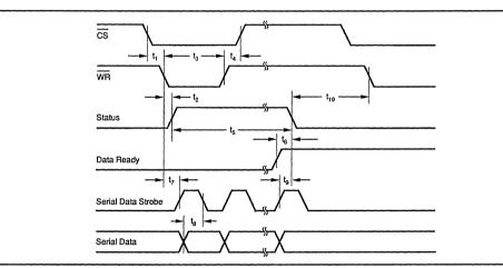
Start of Conversion and Serial Data Output Timing.
