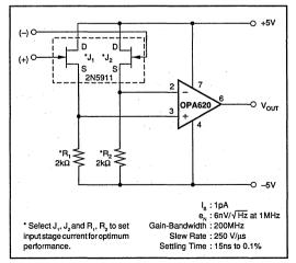
FIGURE 13. Low Noise, Wideband FET Input Op Amp.
