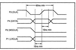
FIGURE 5. PCM60P/66P Setup and Hold Timing Diagram.
