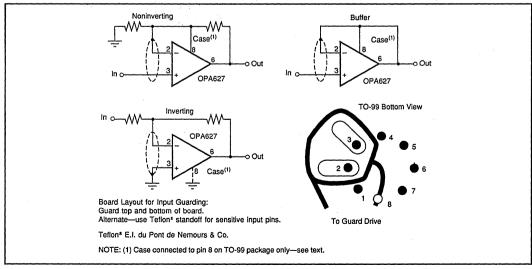
FIGURE 4. Connection of Input Guard for Lowest I<sub>B</sub>.
