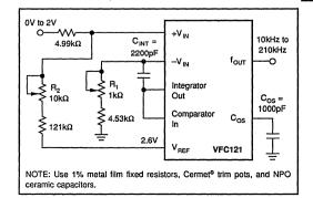
FIGURE 4. Offsetting the Output Frequency.
