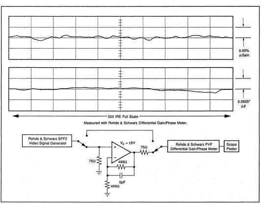
FIGURE 1. Video Differential Gain/Phase Performance.
