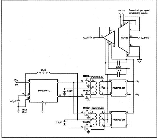
FIGURE 7. Powering the Internally Powered ISO103 Isolation Buffer From a Single 5V Supply. Two Power Channels Are Necessary to Provide the 80mA Nominal for the +V of the ISO103.
