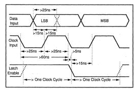
FIGURE 3. PCM61P Setup and Hold Timing Diagram.
