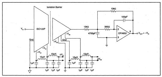
FIGURE 4. Optional  $\pi$  Filter to Minimize Power Supply Feedthrough Noise; Output Filter to Remove 500kHz Carrier Ripple.
