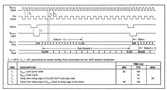
FIGURE 9. Timing when using S<sub>OUT2</sub> Latch.
