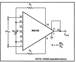
FIGURE 14. Use of External Resistors for Gain Set.
