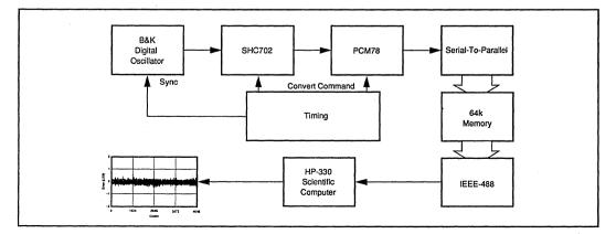
FIGURE 3. Block Diagram of Histogram Test .
