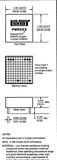
brass with a hot-solder-dipped surface to allow ease of solderability.
