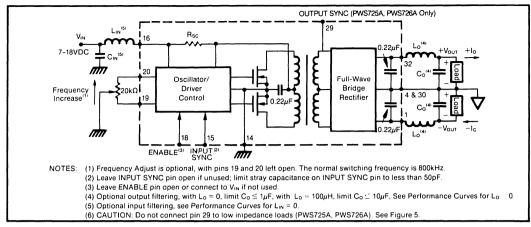
FIGURE 1. PWS725/726 Functional Diagram.
