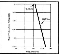
FIGURE 7. Linear First Order Approximation of Filter Circuit.
