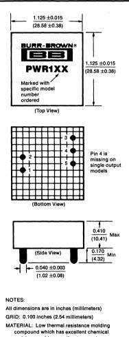
compound which has excellent chemical resistance, wide operating temperature range and good electrical properties under high humidity environments. Lead material is brass with a hot-solder-dipped surface to allow ease of solderability. BURR-BROWN®
