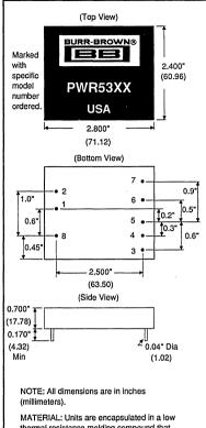
thermal resistance molding compound that has excellent chemical resistance, wide operating temperature range, and good electrical properties under high humidity environments. The shell is a non-conductive black diallylphthalate that allows for six-sided non-conductivity.
