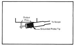
FIGURE 1. Recommended Noise Measurement Method.
