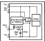
NOTE: Care should be taken when the synchronization input pin is not used, in order to avoid the possibility of noise pick-up and false PLL locking. This could destroy the unit and/or any other units that are coupled to its synchronization output (pin 4). This protection may be accomplished by either tying the synchronization pin to  $-V_{IN}$ , or clipping pin 1 off flush with the module surface. Tying pin 1 to  $-V_{IN}$  is preferred.
