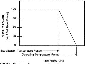
FIGURE 1. Derating Curve.
