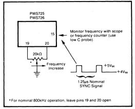
FIGURE 4. Frequency Adjustment Procedure.
