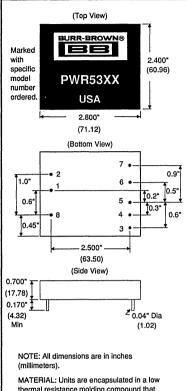
thermal resistance molding compound that has excellent chemical resistance, wide operating temperature range, and good electrical properties under high humidity environments. The shell is a non-conductive black diallyiphthalate which allows for sixsided non-conductivity.
