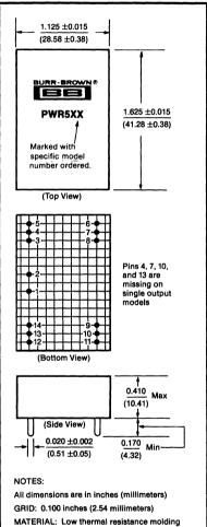
AN EHIAL: Low thermal resistance molding compound which has excellent chemical resistance, wide operating temperature range and good electrical properties under high humidity environments. Lead material is brass with a hot-solder-dipped surface to allow ease of solderability.
