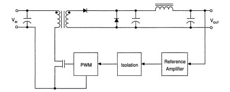
FIGURE 3. The Forward Converter (With Output PI Filter).
