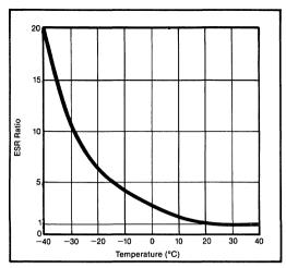
FIGURE 4. ESR Ratio Relative to Room Temperature.
