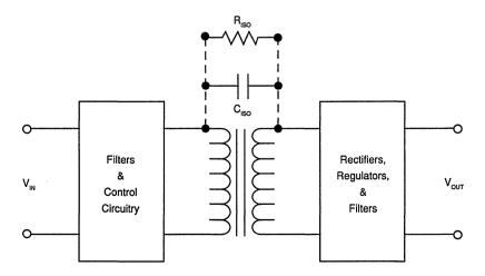
FIGURE 4. Isolation Resistance And Capacitance.
