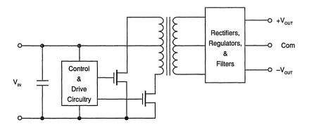
FIGURE 6. Push-Pull Converter.
