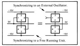
Tha master pin is a buffered output designed to drive other slave inputs. In split rail applications it is recommended that the external oscillator drive only one unit and all others be driven from the master outputs of other PWR1017s.
