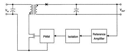
FIGURE 2. The Flyback Converter.
