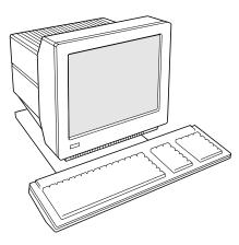
This terminal can emulate a number of ASCII and ANSI terminals, including PC-Term and SCO™ Console. The keyboards supported by the terminal include the 101/102 key extended PC (EPC), the 106/107 PC/+, the VT220™-style ANSI keyboards, and ASCII keyboards.
