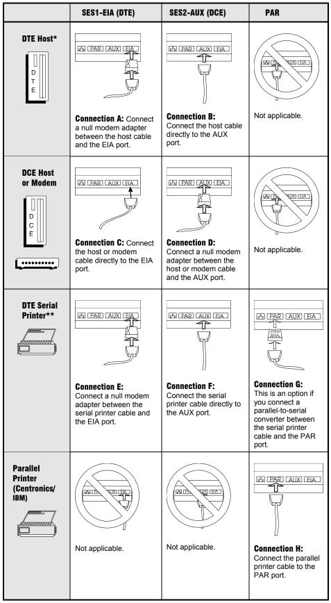
\* Most host computers are configured as a DTE device. The Mentor® System is an example of a DCE host system.
