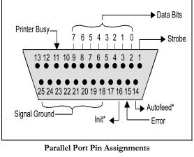
\* These signals are held high, in an inactive state.
