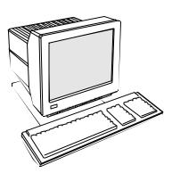
This terminal can emulate a number of This terminal can emulate a number of ASCII and ANSI terminals, including PC-Term and SCO™ Console. The keyboards supported by the terminal are the 101/102 key extended PC (EPC), the 106/107 PC/+, and the VT220™-style ANSI keyboards.
