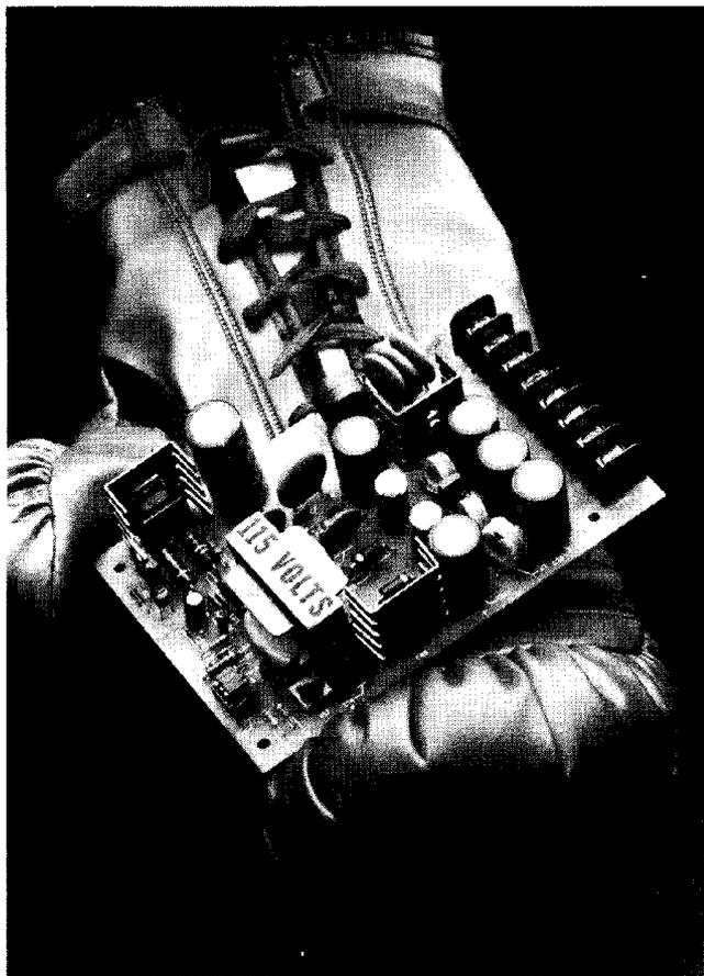
**1. The big punch.** The OL25 switcher measures 2.5 by 4 by 6 inches and weighs 12 ounces; yet it delivers a hefty 25 watts of switching power. An adaptation of the flyback converter, the design minimizes both magnetic and semiconductor costs.
