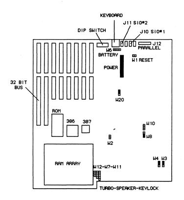
Figure 4. Locations of Items on System Board
