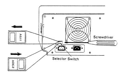
Figure 12. Set the Voltage Selector Switch
