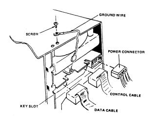
Figure 11. Cable Connections to Peripheral Device
