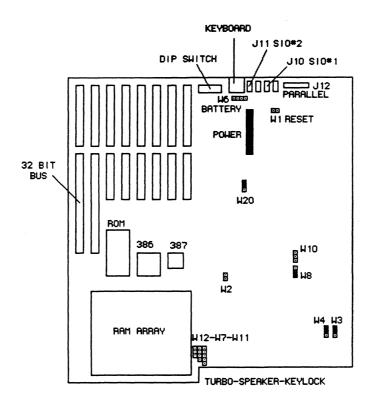
Figure 15. Locations of Items on System Board
