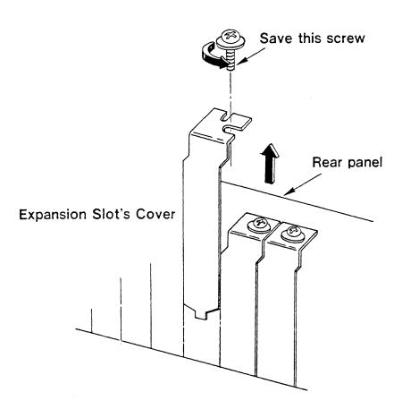
Figure 5. Remove the Expansion Slot Cover
