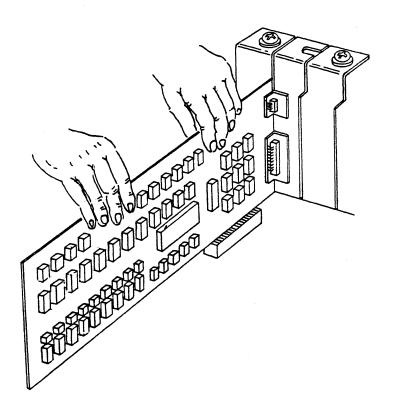
Figure 6. Installing an Option Card
