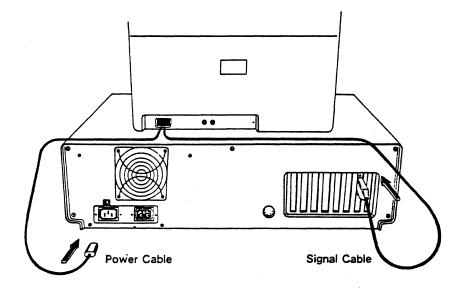
Figure 13. Connect Monitor Cables
