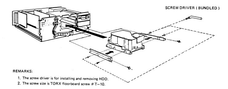
Figure 10. Installing a Peripheral Device
