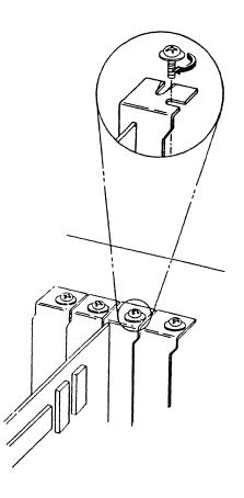
Figure 9. Replace the Bracket Screw
