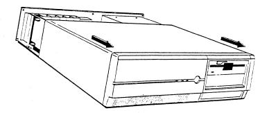
Figure 3. Removing the Cover
