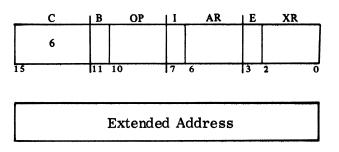
(M) operates on (AR). (XR) is incremented after use.
