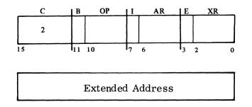
(AR) operates on (M). (XR) is incremented after use.
