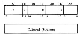
The word following the instruction is the literal source operand. It operates on (AR). If XR is not 0, then (XR) is added to the literal before operating on (AR).
