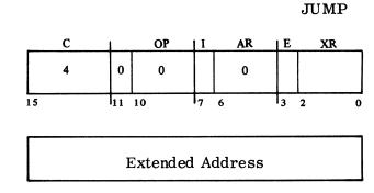
(M) operates on PC, setting it to the jump-location address. The jump function is the same as a MOV (M) to PC, but does not affect status indicators.
