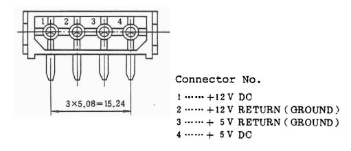
Fig. 2-2 Power supply connector
