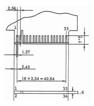
Fig. 2-1 Signal connector
