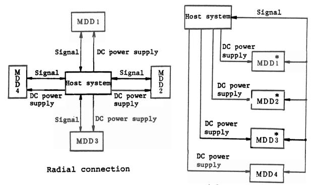
\* Remove resistor arrays. Daisy chain connection
