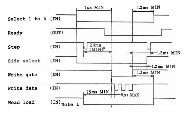
Note 1: The necessary head load waiting time is 25ms from the commencement of actual head loading. (For example, 25ms from 'select on' when head loading by 'select' signal.)
