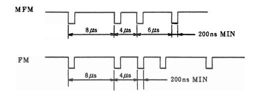
Use a write clock accuracy of  $\pm 0.5$ % (4µs $\pm 20$ ns). Normally, write pre-compensation is not necessary. If it is necessary on account of the system, use it only from the center track in the peripheral direction.
