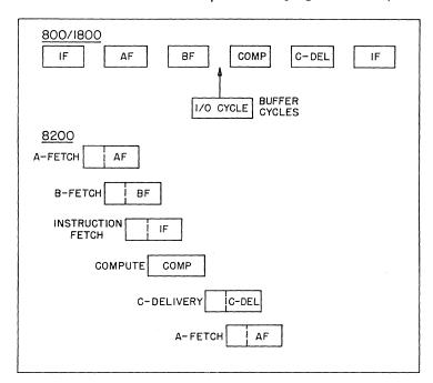
Figure 1. Honeywell 8200 Memory Overlap Compared to Non-Overlapped Operations of Honeywell 800 and 1800.
