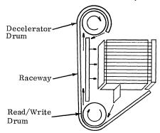
Figure 1: Logical Diagram of the Honeywell Mass Memory File
