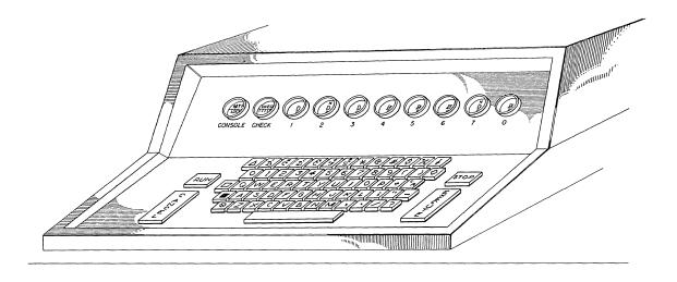
Figure 1. Keyboard and Indicator Lights on Honeywell 800 Console
