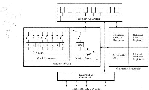
Figure 1. Logical Diagram of the Principal Components of the Honeywell Model 8200.
