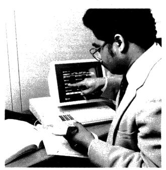
The AT&T Personal Terminal Model 510 is an integrated voice/data terminal (IVDT) equipped with a touch-sensitive screen. Designed for use in conjunction with the AT&T System 75 and System 85 PABXs, the Model 510 provides one-touch access to voice and data functions.
