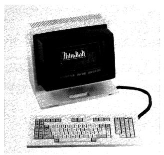
The 4425 is AT&T's high-end asynchronous display terminal offering. The terminal is buffered and features horizontal split screen, windowing, 80-/132-column display capability, and compatibility with both the Unix operating system and the Digital VT102 display. An integral modem is optional.
