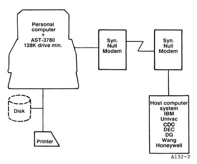
Figure 3. Remote Connection Using a Modem.
