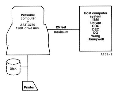
Figure 1. Local Connection Using Null Modem.
