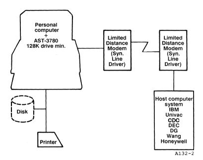
Figure 2. Local Connection Using a Limited Distance Modem.
