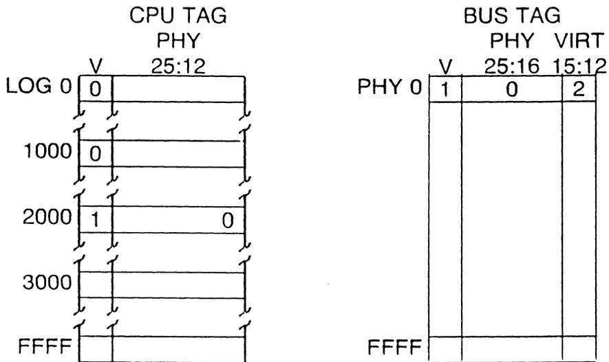
Figure 3-3. Cache Fill: Read Virtual 2000 And Physical 0
