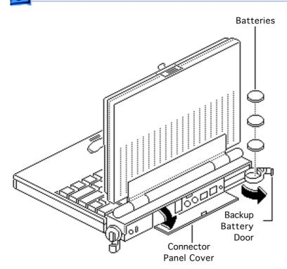
If you are changing the backup batteries without performing other Take Apart procedures, make sure the main battery or the AC adapter is providing power to the computer. You can then remove the batteries without losing the contents of parameter RAM.
