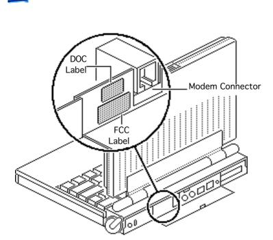
5 Apply the DOC and FCC labels to the left of the modem connector.
