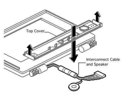
Slip the interconnect cable and speaker through the top cover and remove the top cover.
