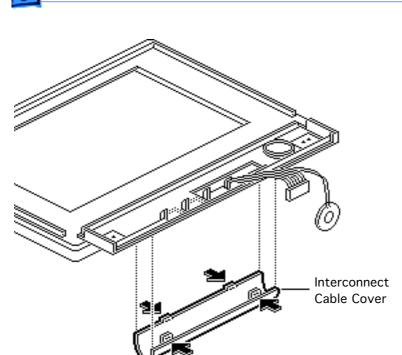
**Replacement Note:** Position the speaker so that the soldered wire terminals are closest to the cable cover.
