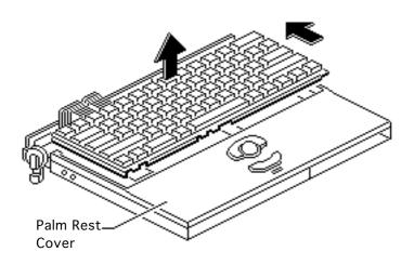
**Caution:** Be careful not to stress the keyboard cables or the connectors on the motherboard.
