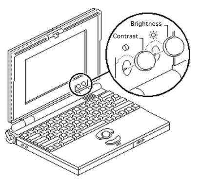
Using your fingers, pry the contrast and brightness knobs off the control shafts.
