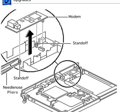
Replacement Note: To remove the fax/data modem, use needlenose pliers to release the locking tabs of the two standoffs and lift the modem from the motherboard.
