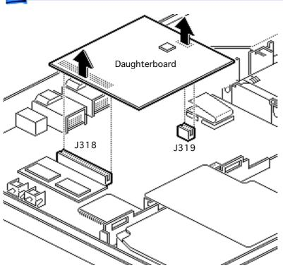
**Note:** To disconnect connector J318, rock it gently from end to end as you lift.
