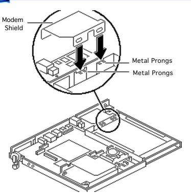
**Caution:** Make sure the modem shield does not extend into the battery cavity.
