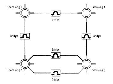
In the mesh network shown in Figure 2-3, a frame has two possible paths from ring 1 to ring 3. The same can be routed through ring 4 or through ring 2.
