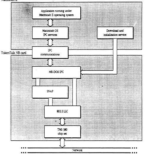
As shown in Figure 1-5, the primary communication interface between the TokenTalk NB card and the Macintosh II is through the interprocess communication (IPC) services. These services are provided by the Macintosh OS on the Macintosh II and by MR-DOS on the TokenTalk NB card. A specific set of services for the 802.2 LLC and SNAP provide the interface to the chip set that handles the low-level protocol processing and physical communication with the token ring network.
