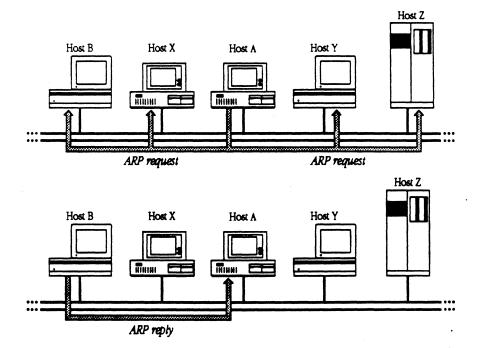
**Figure 3-3** ARP request and reply
