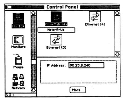
**Figure 7-1** The MacTCP Control Panel
